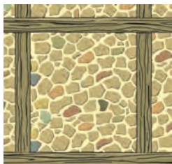
This form of wall called opus craticum is liable to catch fire and collapse unexpectedly.
