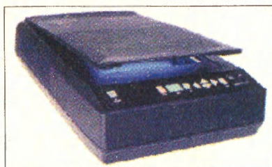
A flatbed scanner's important components are the light source and the photosensitive device, usually a CCD array
