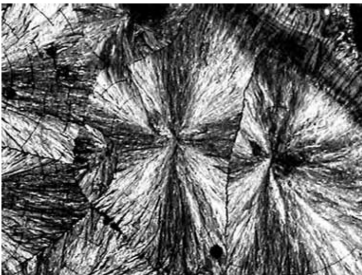
Fig. 2 Visible light micrograph of spherulites from a crystalline diepoxide taken with a 5X lens and cross polarization. The observed maltese cross pattern arises from the spiral positioning of lamella along the radial growth direction. The high refractive index c -axis is tangential to the spherulite's radius.
