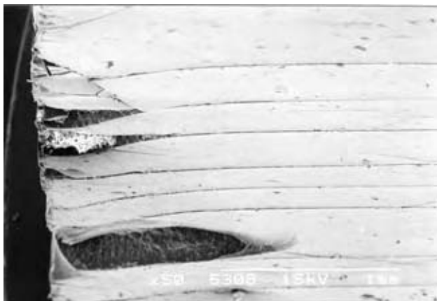
Fig. 8 Surface of polypropylene bar after 80 weeks of UV exposure followed by uniaxial tensile test. Bar axis is vertical. Cracks formed in degraded layer, perpendicular to stress axis. Degraded surface is very fragile and easily parted from underlying material that is less degraded. Degradation tends to be greatest nearer to the corner, possibly because oxygen can diffuse into the surface layers from two adjacent surfaces. (Courtesy of T.J. Turton. See also Refs. [16,24] .)
