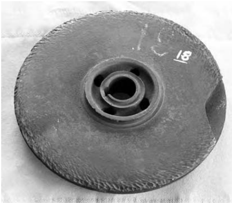
Fig. 4 Flow-induced corrosion of a pump impeller. (View this art in color at www.dekker.com .)
