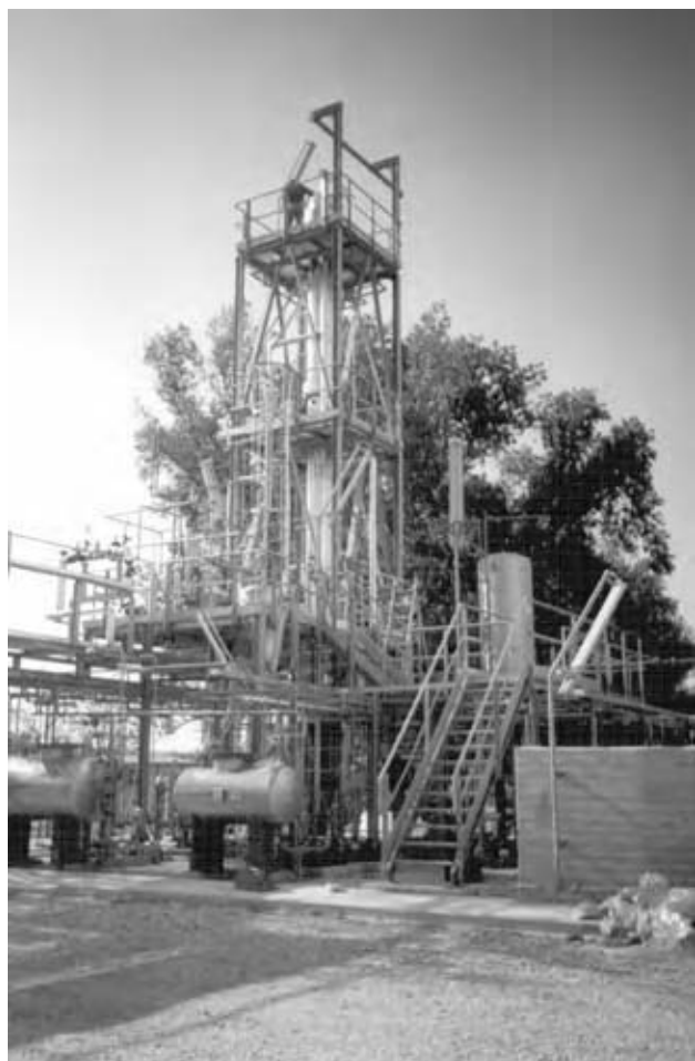
Fig. 7 Combination vapor permeation and distillation. (View this art in color at www.dekker.com .)
