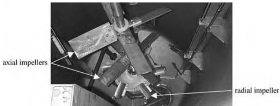
Fig. 2 A typical high efficiency gas-liquid mixing system. (View this art in color at www.dekker.com .)
