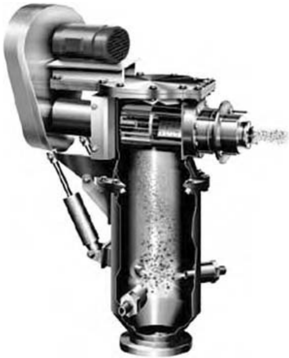
Fig. 14 Cutaway of Roto-Jet showing fluid jets. (Courtesy of Fluid Energy Processing, Telford, PA.) (View this art in color at www.dekker.com .)
