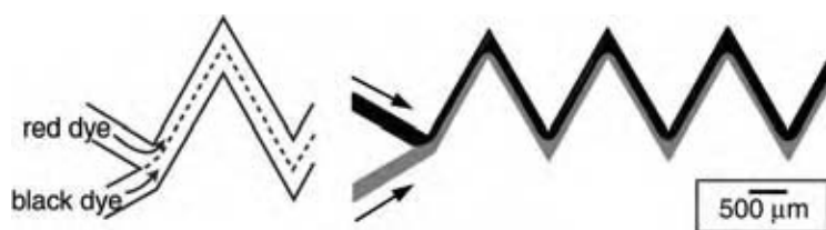
Fig. 3 Illustration of laminar flow in a microfluidic channel. (From Ref. [15] ) (View this art in color at www.dekker.com .)
