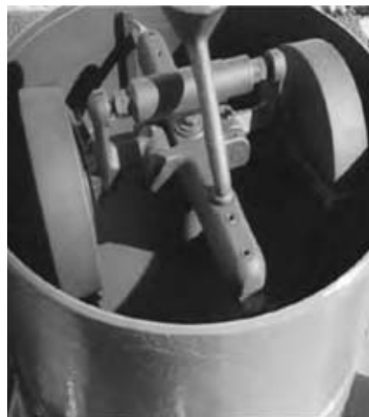
Fig. 5 Mix muller-type mixer. (Courtesy of Süd-Chemie Inc.) (View this art in color at www.dekker.com .)
