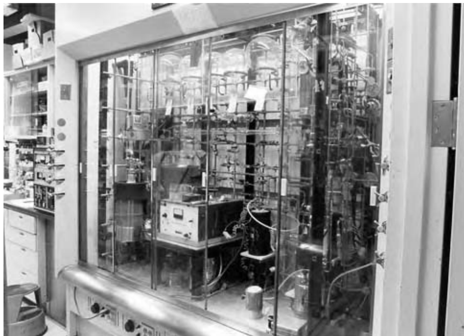
Fig. 1 A laboratory scale pilot installed in a knee height hood. (View this art in color at www.dekker.com .)
