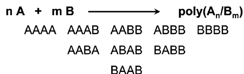
Fig. 10 Reaction of monomers A and B to form a copolymer, and the 10 possible tetrad monomer sequences.
