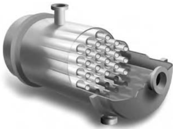
Fig. 13 High flux pervaporation module for silica membrane. (View this art in color at www.dekker.com .)
