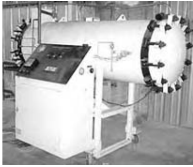
Fig. 6 Example of a small autoclave. (View this art in color at www.dekker.com .)
