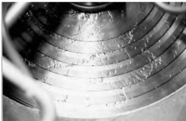
Fig. 1 View of sheared liquid films on an SDR. (View this art in color at www.dekker.com .)
