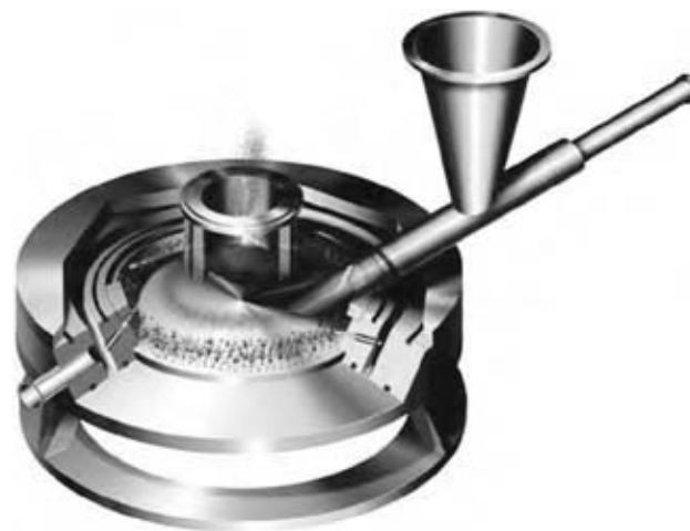
Fig. 13 Cutaway of the Micro-Jet mill showing fluid jets. (Courtesy of Fluid Energy Processing, Telford, PA.) (View this art in color at www.dekker.com .)
