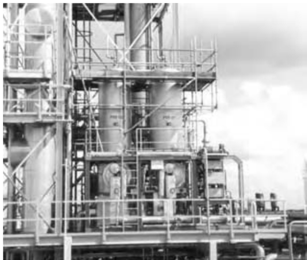
Fig. 25 A pervaporation plant for methanol removal. (View this art in color at www.dekker.com .)
