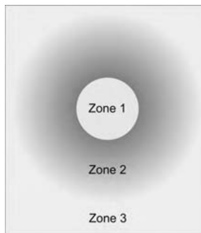
Fig. 4 Three reaction zones generated by acoustic cavitation. Zone 1 is the vapor phase, Zone 2 consists of the supercritical fluid region, and Zone 3 represents the bulk liquid. (View this art in color at www.dekker.com .)
