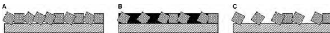
Fig. 1 Schematic of the three types of zeolite membranes: (A) a polycrystalline zeolite membrane; (B) a zeolite matrix composite membrane; and, (C) a zeolite crystal layer.
