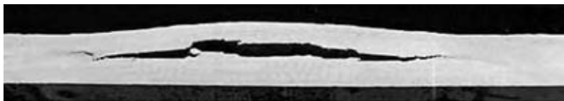
Fig. 8 Hydrogen-induced cracking—note the internal split produced by the precipitation of hydrogen gas onto flattened sulfide inclusions.
