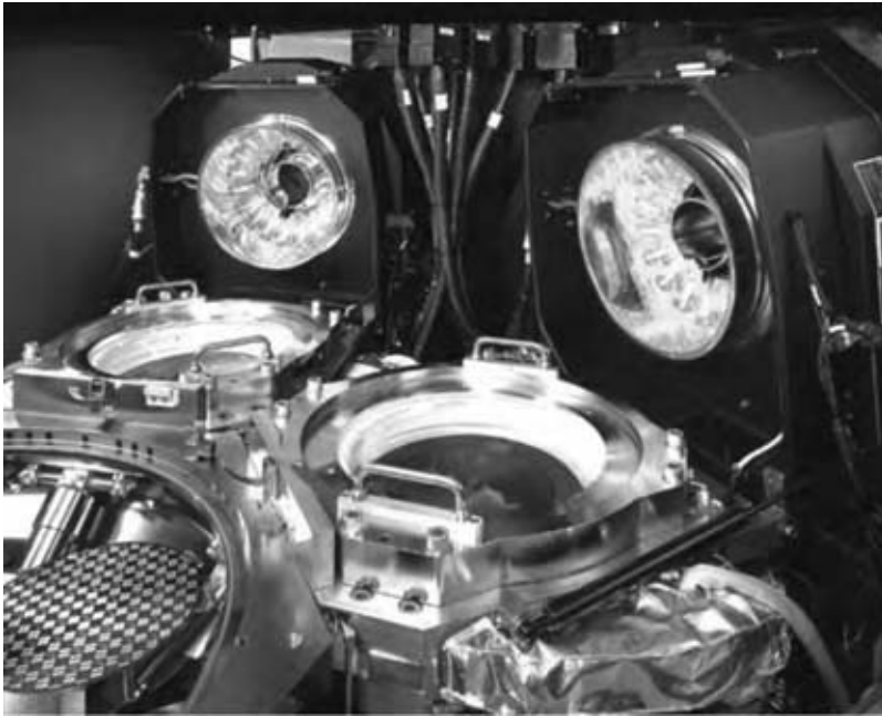
Fig. 6 Deposition system used for epitaxial CVD. Heating in this case is accomplished by banks of lamps (e.g., upper right). (Photo courtesy of Applied Materials Inc.) ( View this art in color at www.dekker.com . )
