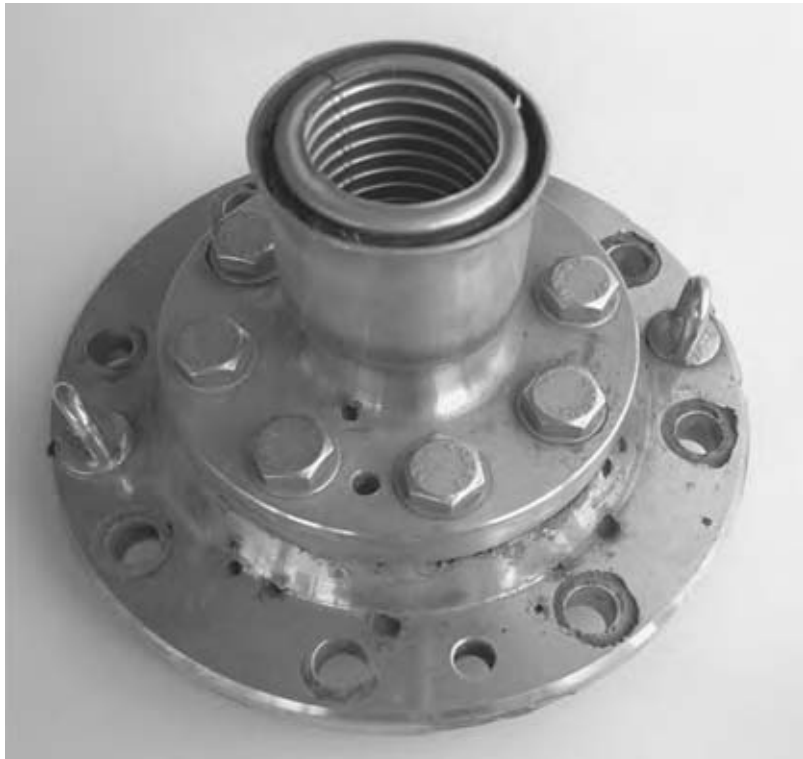
Fig. 3 Crevice and pitting corrosion of a stainless steel autoclave head. Note the crevice corrosion underneath the bolts (now removed) and in the gap between the two parts that are still assembled, and the pitting corrosion on the free surface. This corrosion was probably caused by chloride derived from thermal insulation. (View this art in color at www.dekker.com .)
