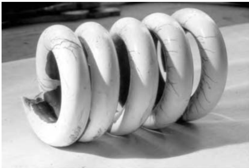
Fig. 7 Cracks in a high strength steel relief valve spring. The cracks have been revealed using a dye that penetrates into the crack then seeps back out into a porous white coating. The cracks were caused by hydrogen embrittlement of the excessively hard steel, coupled with tensile residual stresses and the storage environment on a chemical plant (with an occasional trace of H_2S ). (View this art in color at www.dekker.com .)
