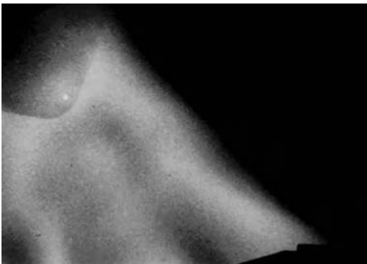
Fig. 4 Phosphor thermometry measured in an exhaust plume of jet engine afterburner.
