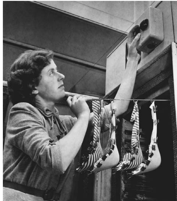
Bikini bras in production. Treated fabric, having been stretched over a plastic mold, is about to be baked in order to set its shape and create bikini brassieres. These bras were manufactured in 1949, but it was not until the 1960s that bikinis caught on in the United States. © HULTON-DEUTSCH COLLECTION/CORBIS. REPRODUCED BY PERMISSION.
