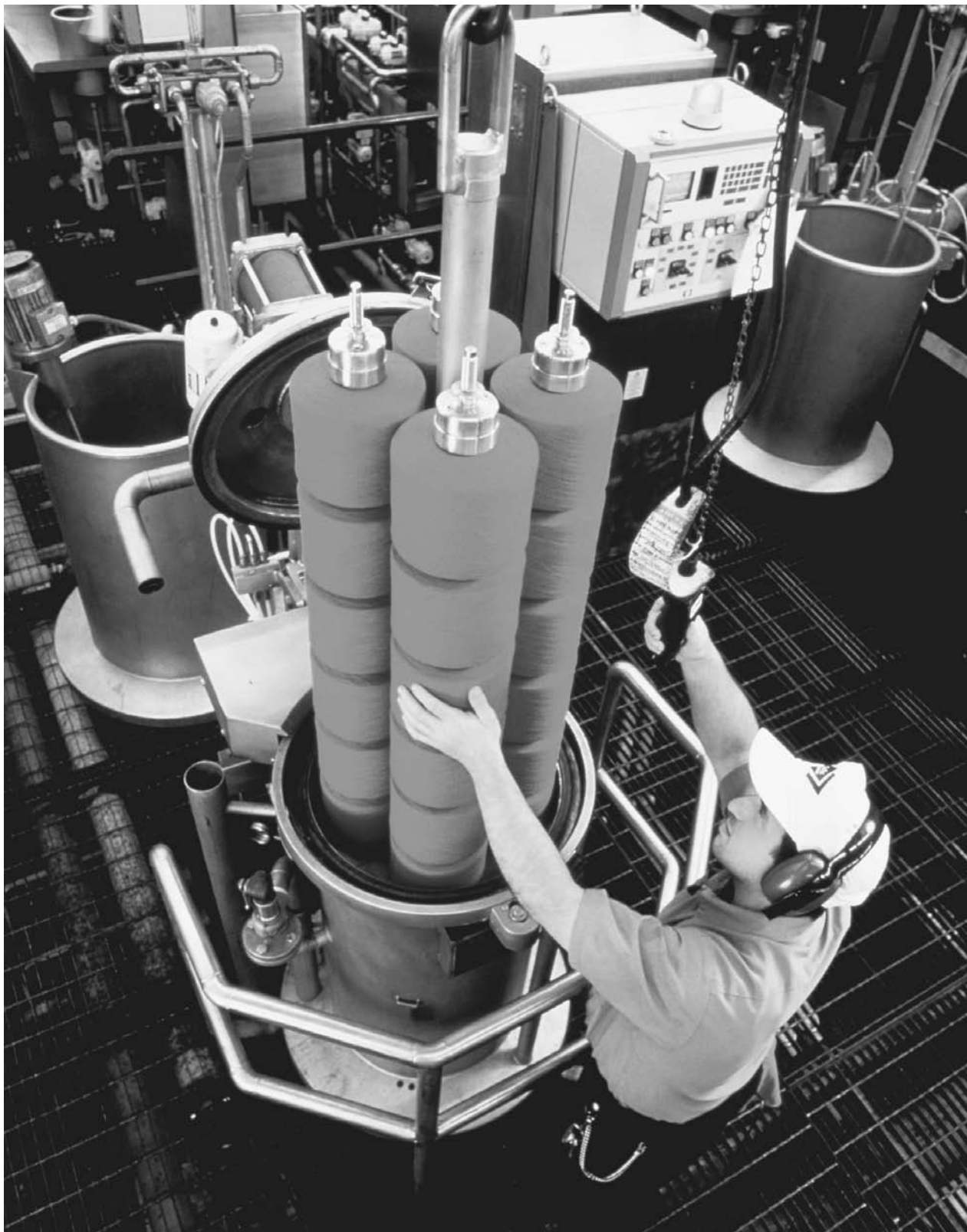
Yarn dyeing. A worker lowers four spoils of yarn into a dyeing vat with a remote control. Textile styles such as bouclé and tweed can be produced by blending different color yarns. © ROGER BALL/CORBIS. REPRODUCED BY PERMISSION.
