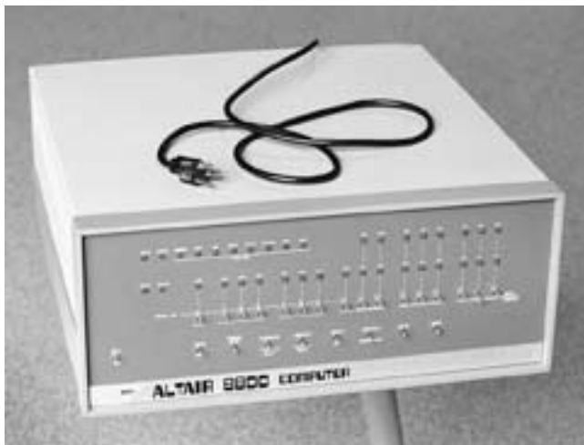
The MITS Altair (1975) was the first microcomputer available commercially. It was generally purchased in kit form. While the Altair did not have much processing capacity, it aroused great interest and inspired other computer builders such as Apple’s Steve Wozniak and Steve Jobs. (CHRISTOPHER FITZGERALD / THE IMAGE WORKS)
