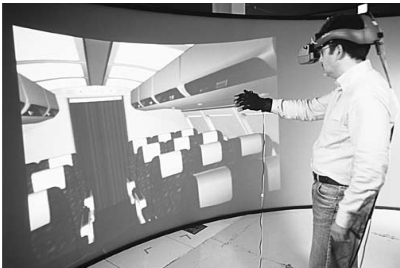
A NASA researcher wearing an early virtual reality (VR) outfit, including head-mounted display and gloves whose position can be tracked. (NASA PHOTO)
