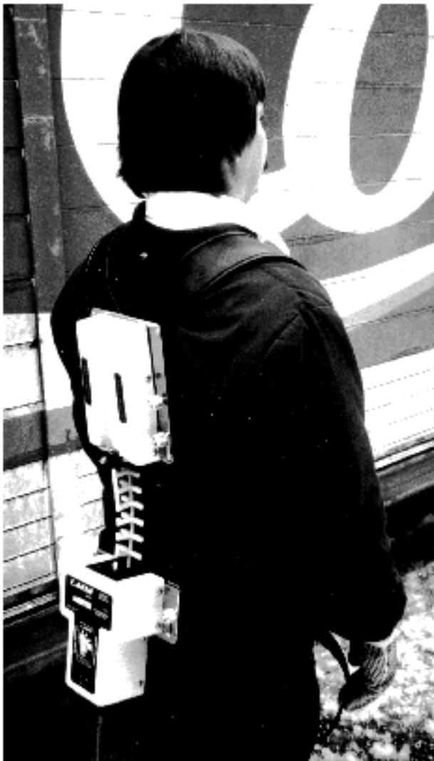
**Figure 3.** Electrical goniometers used to quantify postures and motions of the wrist (a) when performing a keyboarding task (photo courtesy Richard Marklin) and on the spine (b) when performing a beverage delivery job.
