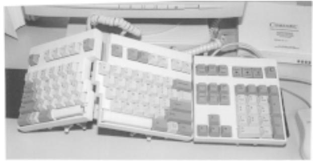
**Figure 2.** Example of a variable geometry ergonomic keyboard.
