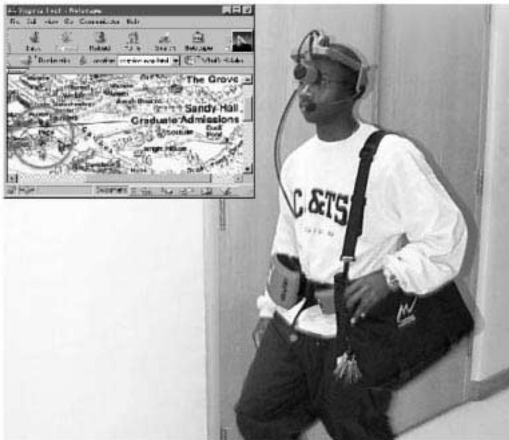
Figure 1. Picture of a user with a wirelessly networked "Mobile Assistant" wearable computer accessing a map of Virginia Tech through the World Wide Web (Picture courtesy of Virtual Environment Laboratory, Virginia Tech).
