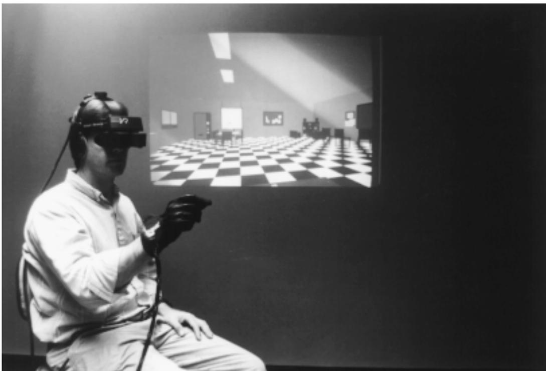
Figure 1. A virtual environment viewed through an opaque head-mounted display (HMD). Also shown is a glove with a 6° of freedom position sensor allowing the user to manipulate virtual objects.
