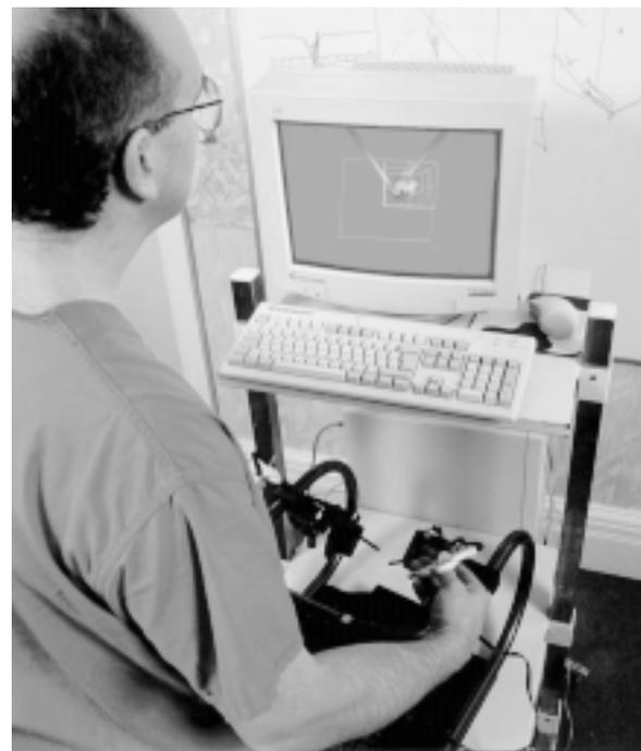
**Figure 9. Minimally invasive surgical trainer (MIST) in use. Courtesy Virtual Presence.**
