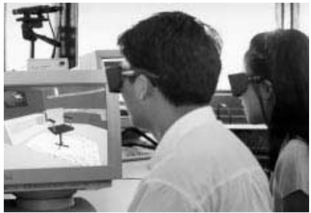
**Figure 3.** Two users viewing a desktop VR system in stereo, each wearing a pair of shutter-glasses™.
