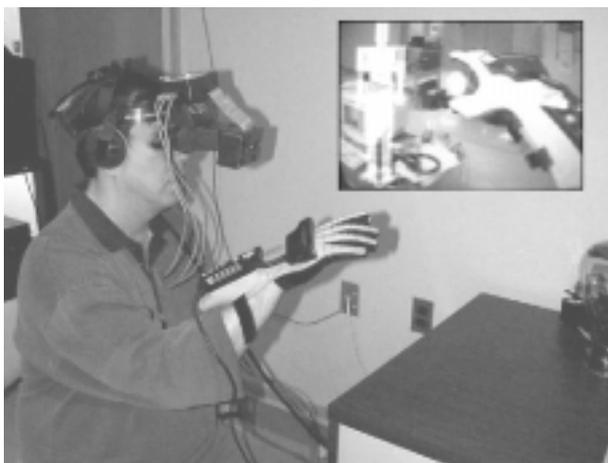
Figure 1. Graphical image overlaid onto video image. The user is wearing an opaque HMD with a CCD camera and luminance keyer. Courtesy: Virtual Environment Laboratory, Virginia Tech.
