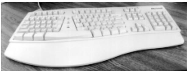
**Figure 1.** Example of a fixed geometry ergonomic keyboard.
