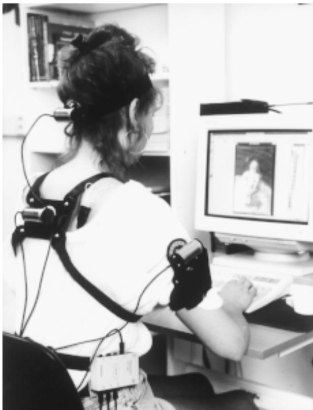
Figure 1. The physiometer records EMG on four channels; six channels are available for postural angles measurements. Inclinometers are attached to the upper arm, head and back
