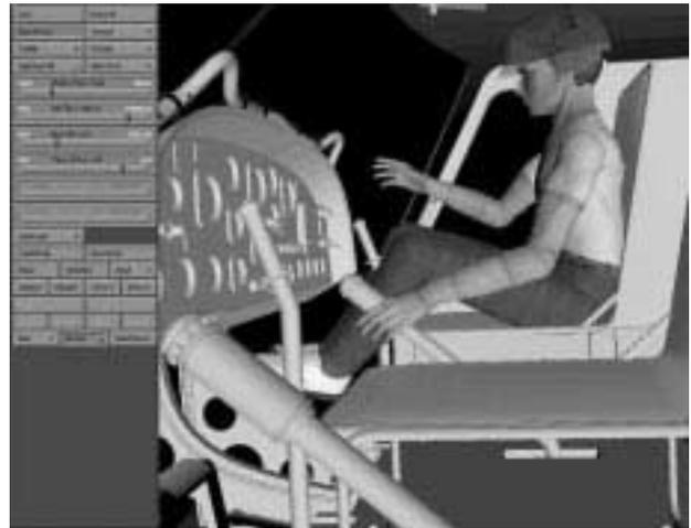
Figure 4. Anthropos as an example of Virtual Ergonomic Prototyping (source: IST).
