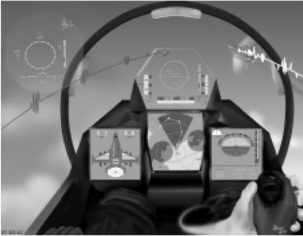
**Figure 1.** Within 7 years, the tactical cockpit will include a HUD, HMD, HLD, localized audio, DVI and haptic displays.
