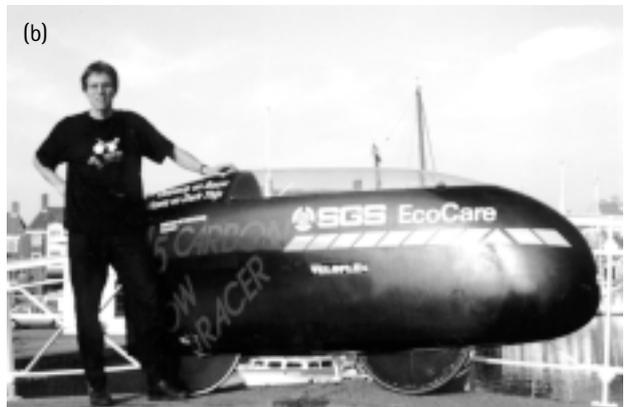
Figure 3. Two typical recumbents for racing: a carbon low racer with tail fairing (a) and a fully faired carbon racing recumbent (b) (both courtesy: Bram Moens, M<sub>3</sub>).
