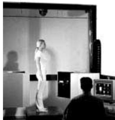
Figure 1. Collection of anthropometric data with the VITUS 3D Body Scanner (source: Tecmath, TUM).
