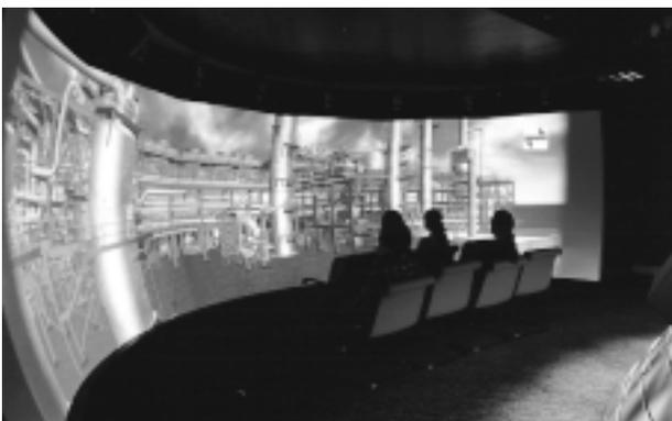
Figure 5. Example of a large-scale projection display. Courtesy CADCentre.
