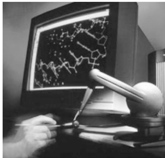
Figure 6. PHANTOM haptic interface. Courtesy Sensable Technologies.
