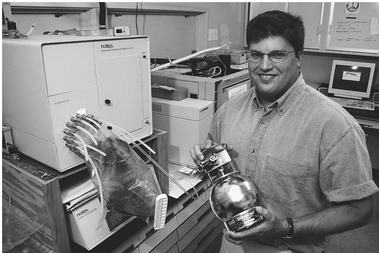
A researcher at the Environmental Technology Group at Pennsylvania State University holds a Suma canister, a device used to collect air samples, in front of a cryogenic concentrator and gas chromatograph that is used to analyze the sample. AP/WIDE WORLD PHOTOS.
