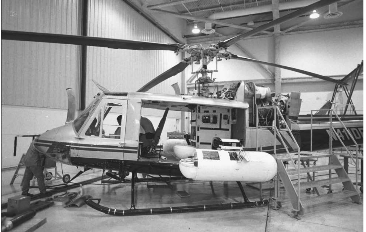
Nuclear Emergency Search Team members install radiation-sensing equipment into a helicopter at the NEST facility at Nellis Air Force Base in Nevada. AP/WIDE WORLD PHOTOS.
