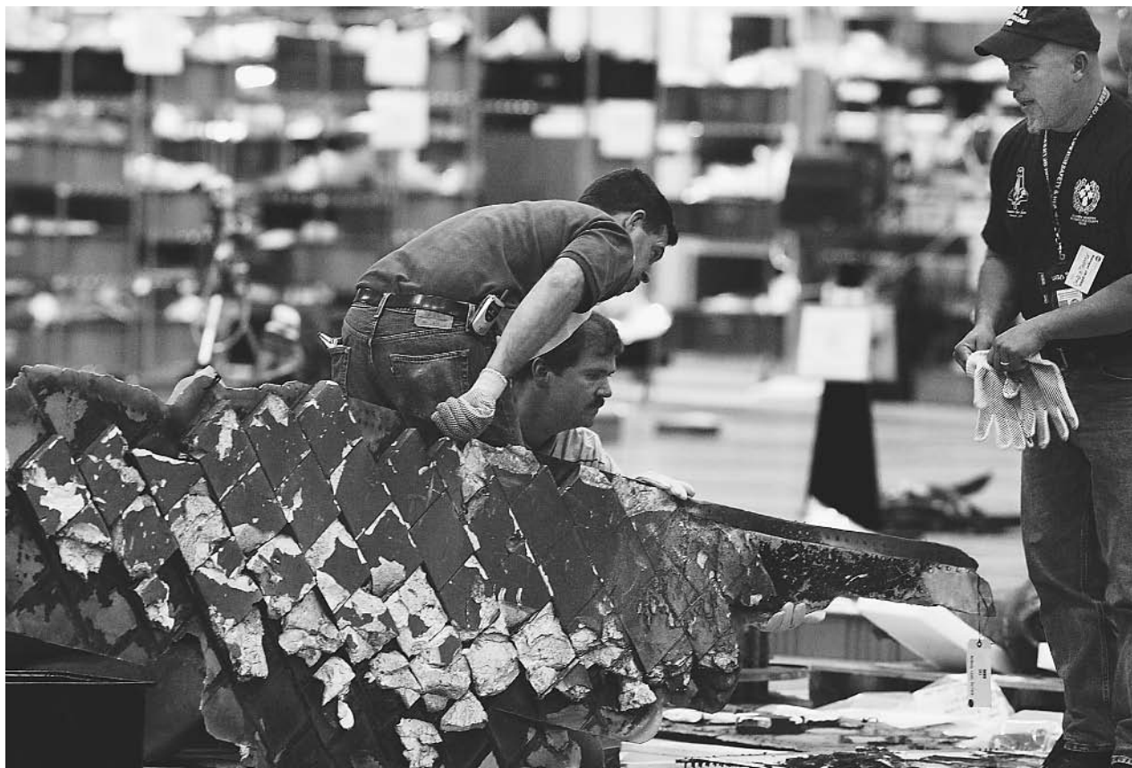
Members of the investigating team inspect part of the left wing from the Space Shuttle Columbia wreckage in the hangar where it is reconstructed at the Kennedy Space Center in Cape Canaveral, Florida. NASA engineers used GIS mapping technology to map debris field patterns that helped narrow the areas to be searched. AP/WIDE WORLD PHOTOS.
