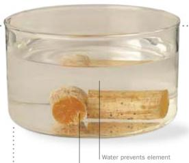
White phosphorus is volatile and ignites on contact with air
