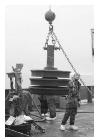
Railroad wheels are often used as anchors when deploying oceanographic buoys. (NOAA)
