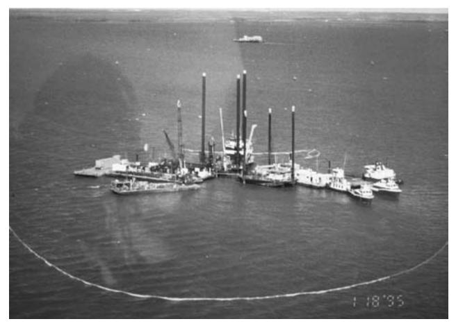
A containment boom helps to confine oil spilled from a drilling rig. (NOAA)
