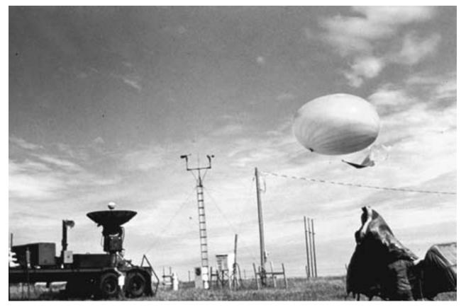
Meteorological measuring instruments including anemometers, wind vanes, temperature and humidity sensors, rain gauges, sounding balloons, and Doppler radar (NOAA/NWS)
