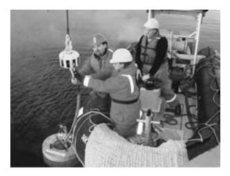
Recovery of an RD Instruments acoustic Doppler current profiler (ADCP) from a deep-sea deployment (RD Instruments)
