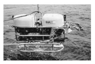
A Remotely Operated Vehicle, a tethered underwater robot, breaks the surface after extensive underwater operations. (NOAA/NURP)
