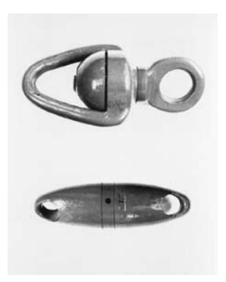
A swivel is a fitting composed of rotating elements (eye-bolt, nut, and box). Swivels normally connect mooring lines and chain and prevent twisting. Heavy swivels or swivel anchor connectors are designed to slide over anchor rollers and prevent snagging. (NOAA, Y. Berard)
