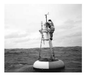
Oceanographic buoy deployed for detection of environmental conditions favorable for the development of El Niño (NOAA)
