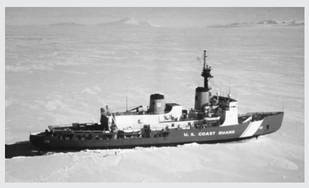
U.S. Coast Guard Cutter *Polar Sea* breaking ice epitomizes the powerful engines and reinforced bows that are required to maintain channels through sea ice. (*USCG*)
