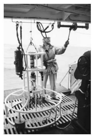
Conductivity-temperature-depth (CTD) instrument is being deployed at sea. In addition to the CTD probe, the frame supports a Niskin water sampling bottle and an acoustic "pinger" for probe location. (NOAA)
