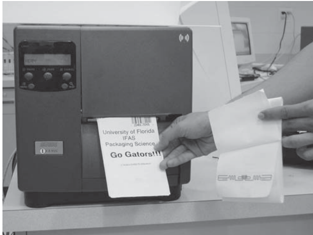
Figure 13. Datamax, Inc. (Orlando, FL) Model I-4210 RFID-enabled thermal transfer printer in the packaging laboratory at the University of Florida. (Photo by Bruce Welt University of Florida.)
