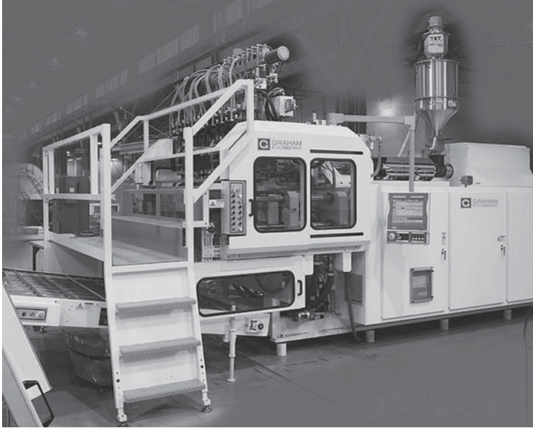
Figure 7. Typical reciprocating-screw intermittent-extrusion blow-molding machine. (Courtesy of Graham Engineering Corporation.)
