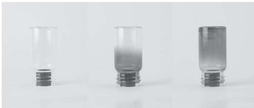
Figure 8. Typical bromophenol blue in poly(vinyl butyral)/tributyl phosphate film-coated sample bottle inverted over a sample bottle cap containing putrescine. The images were recorded after 0-, 10-, and 20-min exposure to the vapor above the sample bottle cap (33).
