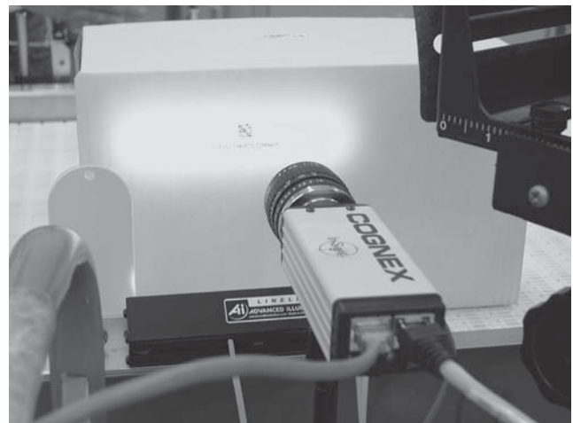
Figure 8. Cognex InSight camera reading a label. (Photo by Bruce Welt, University of Florida.)
