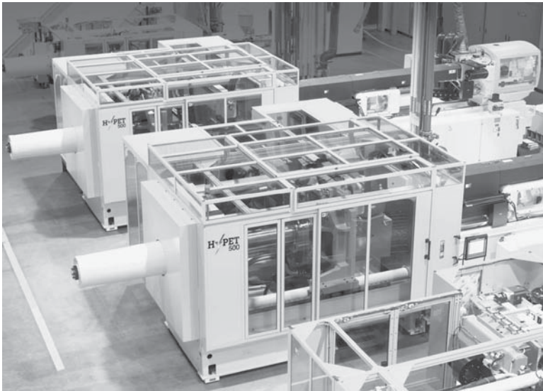
Figure 11. Typical high-output preform injection-molding machine. (Courtesy of Husky Injection Molding Systems.)
