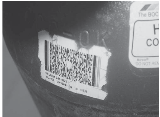
Figure 11. A slightly damaged 2D barcode. Although damaged, much of the remaining data can still be used.
