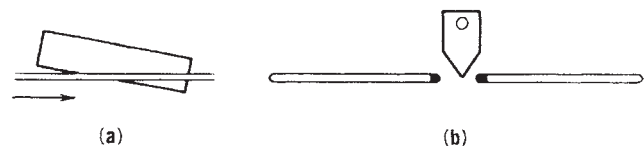
Figure 7. Slit sealer (hot-knife type). (a) side view; (b) top view.
