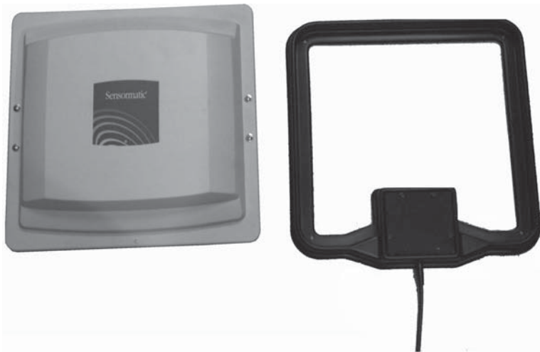
Figure 21. UHF (left) and HF (right) RFID antennas.
