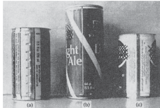
Figure 1. Three-piece can side seams (a) soldered; (b) cemented; (c) welded. Courtesy of Proceedings, 3rd International Tinplate Conference , 1984.
