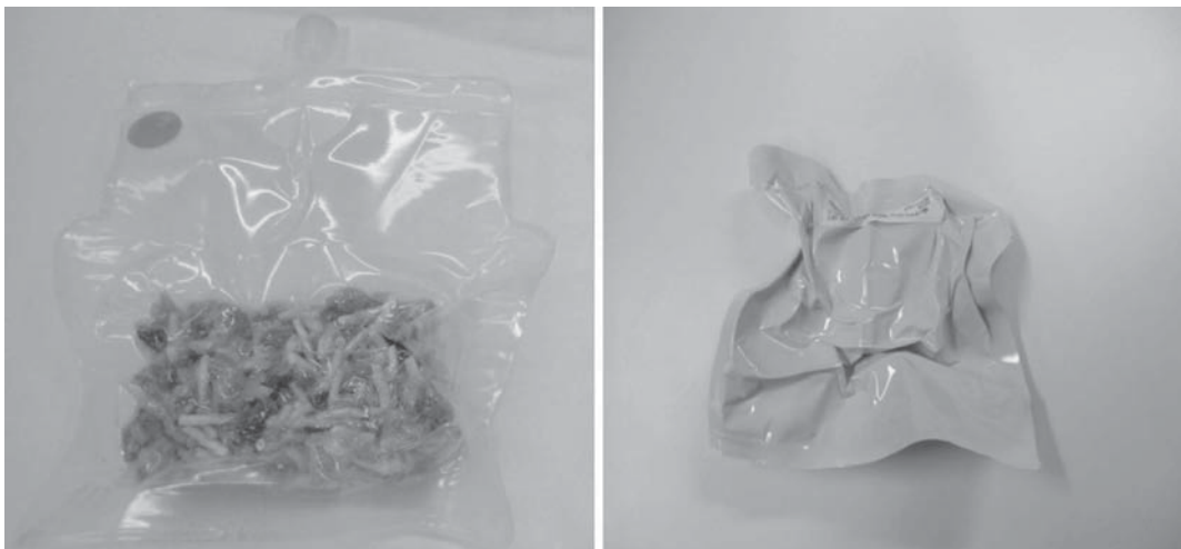
Figure 6. Freeze-dried item in primary COM packaging (left) and with RPP overwrap (right).
