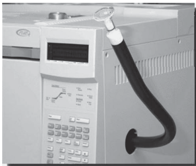
Figure 1. Gas Chromatograph equipped with a sniff port.
