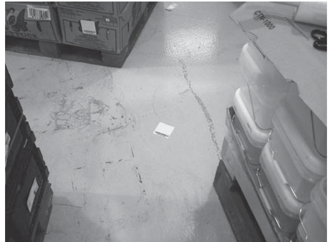
Figure 5. RFID tag that fell from palletized product. (Photo by Bruce Welt, University of Florida.)
