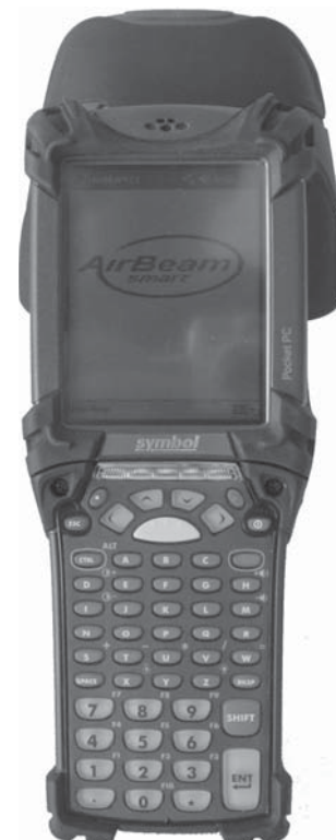
Figure 16. Symbol Personal Digital Assistant (PDA) with embedded barcode reader and RFID functionality.
