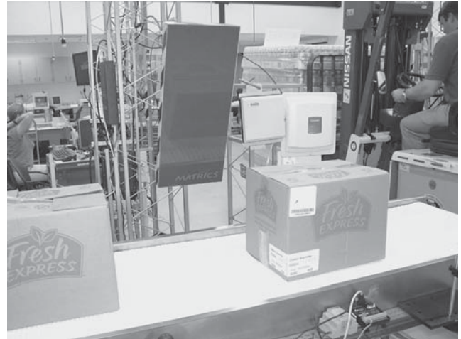
Figure 15. Tagged cartons pass RFID antennas on a conveyor belt in packaging laboratory at the University of Florida. (Photo by Bruce Welt, University of Florida.)
