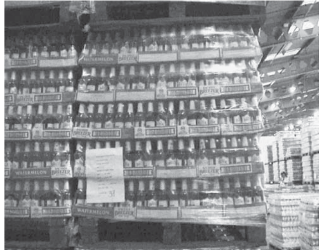
Figure 5. Uneven loading in the pallet stacks.
