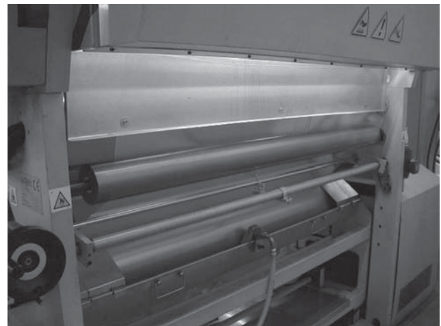
Figure 18. In-line infrared drying equipment (enlightened part). Note the engraved chrome-plated roll partially covered by the metallic pan. (Courtesy of Metalvuoto Spa, Roncello, Italy.)
