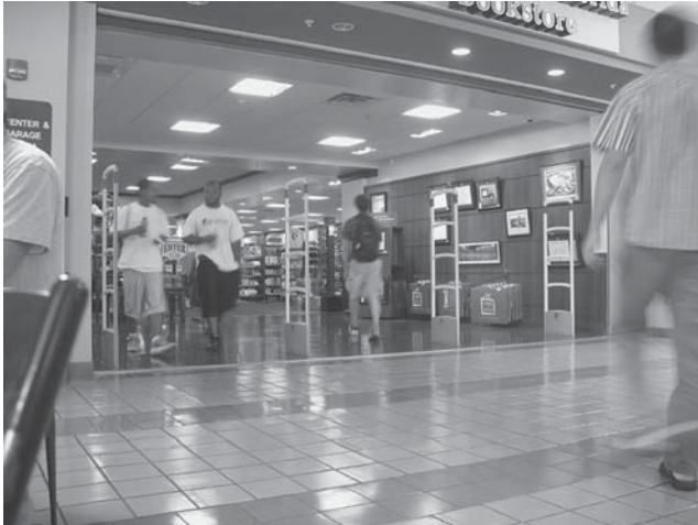
Figure 1. Checkpoint EAS antennas use special one-bit tags to detect unauthorized removal of products from premises.
