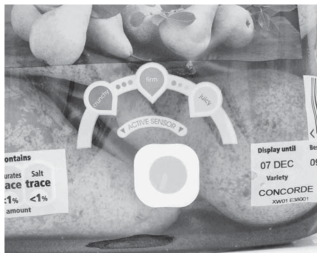
Figure 10. A pack of four Concorde pears with active ripeness indicator. The label inside the pack changes color from dark red to yellow as the pears ripen.
