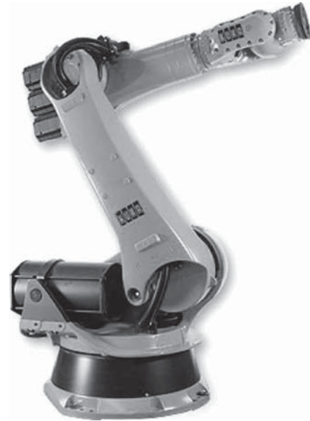
Figure 12. Floor-mounted 6-axis articulating robot. Models also come in platen-mounted designs. End of arm tooling not shown. (Photo courtesy of KUKA Robotics.)
