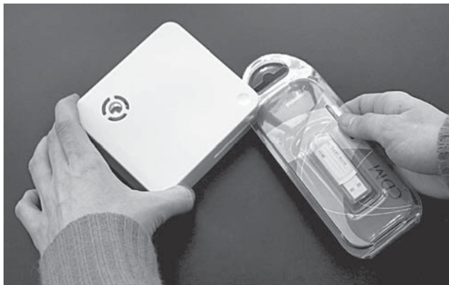
Figure 6. Electrical debonding at point of sale of a hard-to-open clamshell package via a hand-held power source. (Reproduced with permission from Stora Enso.)
