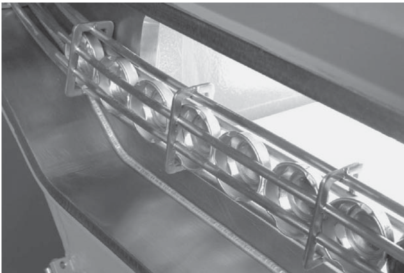
Figure 4. High-energy electron accelerator sterilizing bottle caps. (Photograph provided by Advanced Electron Beams, Inc. Wilmington, MA.)
