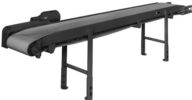
Fig. 6. Belt conveyor. (Aseeco Corp.)
