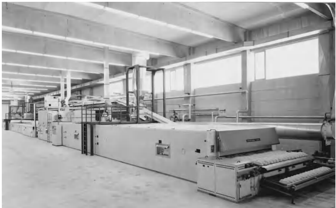
Fig. 7. Tunnel oven. Loaf-size dough pieces enter the oven at left background and are carried through the baking chamber on a continuous metal belt which serves as the hearth. The baked loaves exit at right foreground. Ordinary pan bread would require sets of pans conveyed by a slightly different mechanism, but the basic oven structure would be the same. (Adam Equipment Co.)
