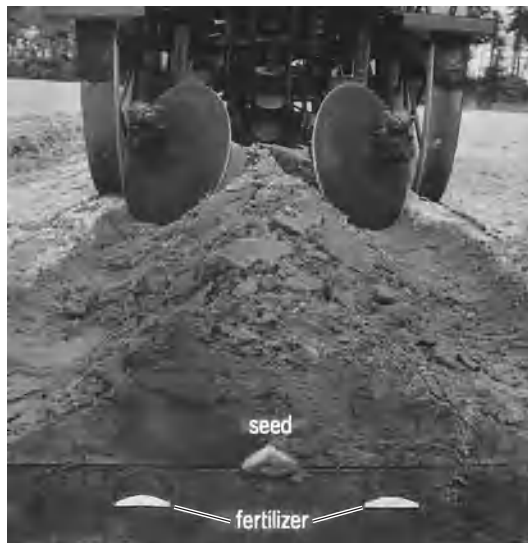
Fig. 1. Efficient placement of fertilizer for potatoes. Attachments to make fertilizer placement at the time of planting are available on most field row planters. (USDA, Agriculture Research Service)
