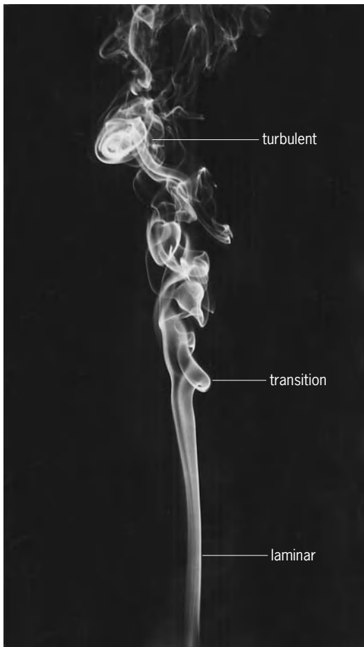
Fig. 5. Laminar and turbulent flow in a smoke plume. (From S. Whitaker, Introduction to Fluid Mechanics , Krieger Publishing, 1981)
