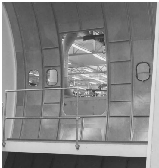
Fig. 10. Bonded honeycomb sandwich fuselage panel. (After J. E. McCarty, Application of advanced structures and materials to transport aircraft fuselages , AIAA Pap. 74-340, AIAA/ASME/SAE 15th Structures, Structural Dynamics and Materials Conference, Las Vegas, 1974)
