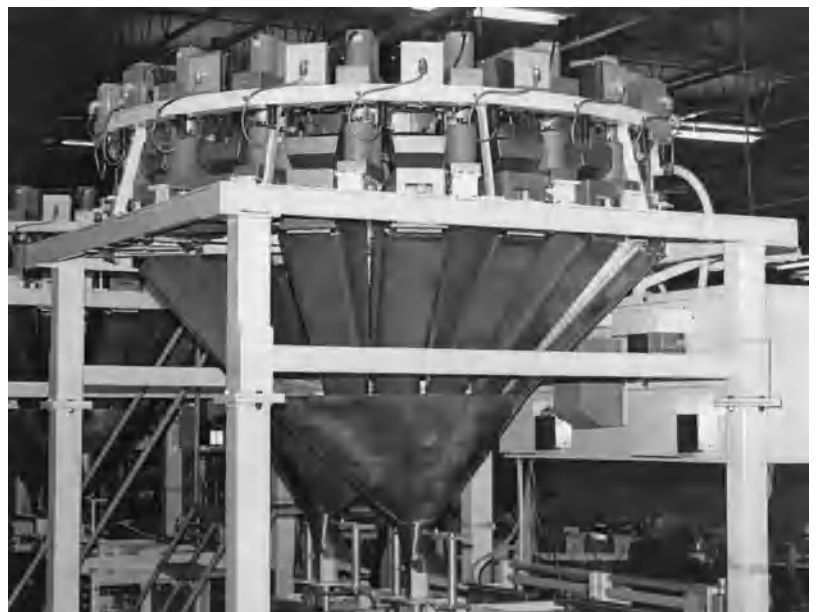
Fig. 48. Computer-controlled multiple-scale weighing device for snack foods used on vertical form/fill/seal flexible packaging machine. (Kliklok Co.)
