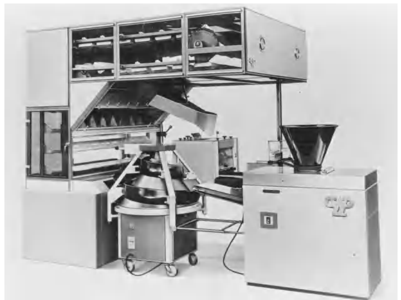
Fig. 6. Small integrated bread make-up system. A mass of bread dough is placed in the hopper of the divider (right) which cuts it into pieces of uniform weight. The rounder (center foreground) receives the rough pieces from the divider, forms them into spheroids, and delivers them to the overhead proofer. The dough undergoes a fermentation period while traveling through the proofer in individual pockets. The proofed dough pieces fall into the molder (center background) which sheets the dough and then curls it into a cylinder ready for depositing into baking pans. (Adam Equipment Co.)
