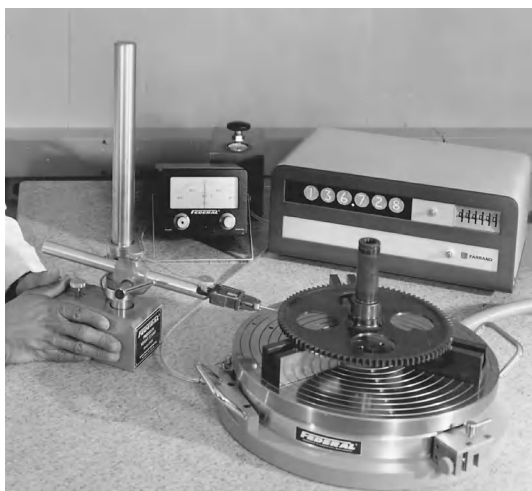
Fig. 4. Indicating gage of the electronic type being used to inspect a part. (Federal Products Corp.)
