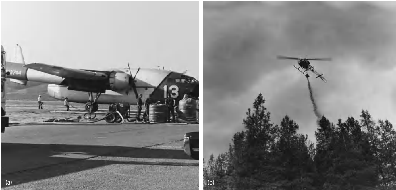
Fig. 7. Aerial fire suppression. (a) Mixing and loading fire retardants in preparation for an air drop. (b) A helicopter with a detachable 40-gal (151-liter) tank drops borate slurry on a pinpoint target. (U.S. Forest Service)
