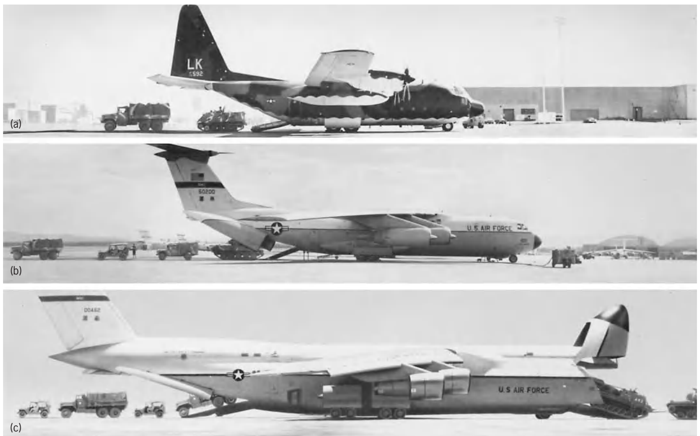
Fig. 1. Military cargo aircraft, showing fuselage configurations. (a) C-130 Hercules, (b) C-141 Star Lifter. (c) C-5A Galaxy. (Lockheed Corp.)
