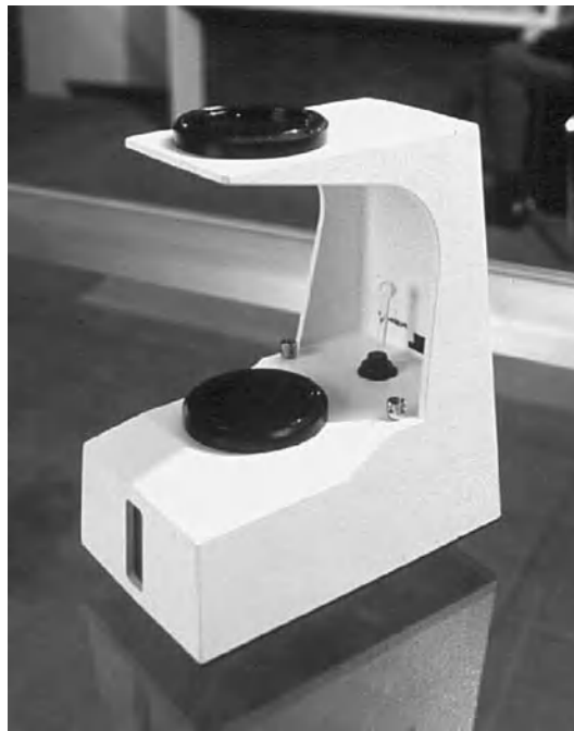
Fig. 2. Polariscope to distinguish between single and double refraction. (Gemological Institute of America)
