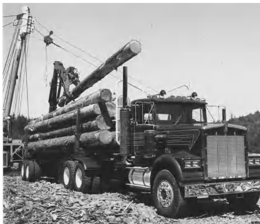
Fig. 3. Heavy-duty log truck-trailer being loaded with a grapple. Part of a steel yarding tower is visible at the left and is rigged with a skyline cable system. (Kenworth Truck Co., Division of PACCAR)
