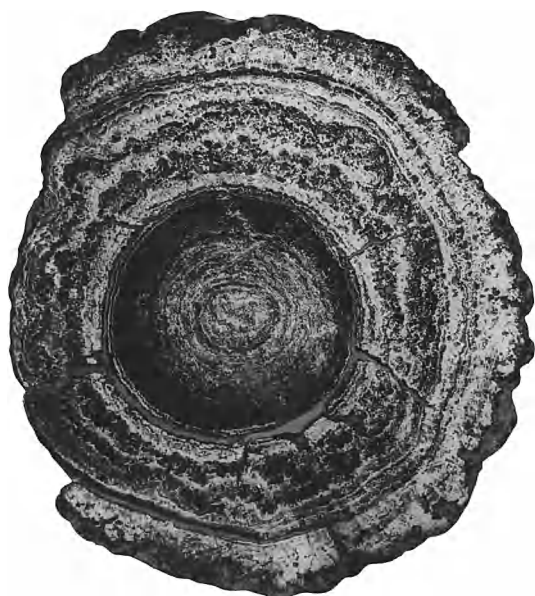
Fig. 1. Reflected-light photograph of the polished surface of a sectioned manganese nodule showing the complex growth history of the concretionary deposit (diameter 1.6 in. or 4 cm).
