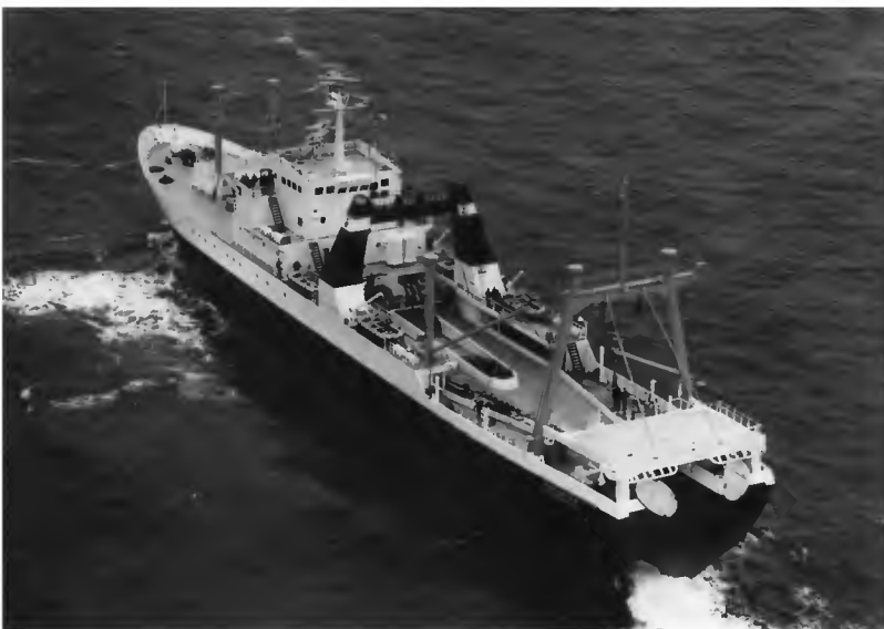
Fig. 4. Example of a long-distance factory trawler (3177 ft or 95 m long, 5000 hp or 3.7 MW) capable of bottom and midwater trawling anywhere in the world. ( Hansetische Hochseefischerei, Germany )
