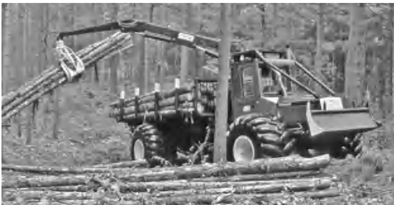
Fig. 2. Forwarder loading logs for transport to landing. (John Deere)
