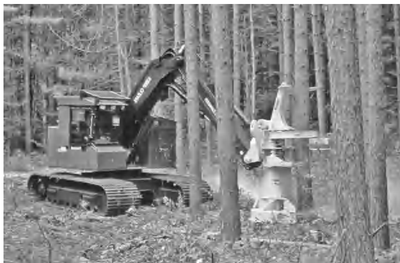
Fig. 1. Feller-buncher cutting tree. (John Deere)
