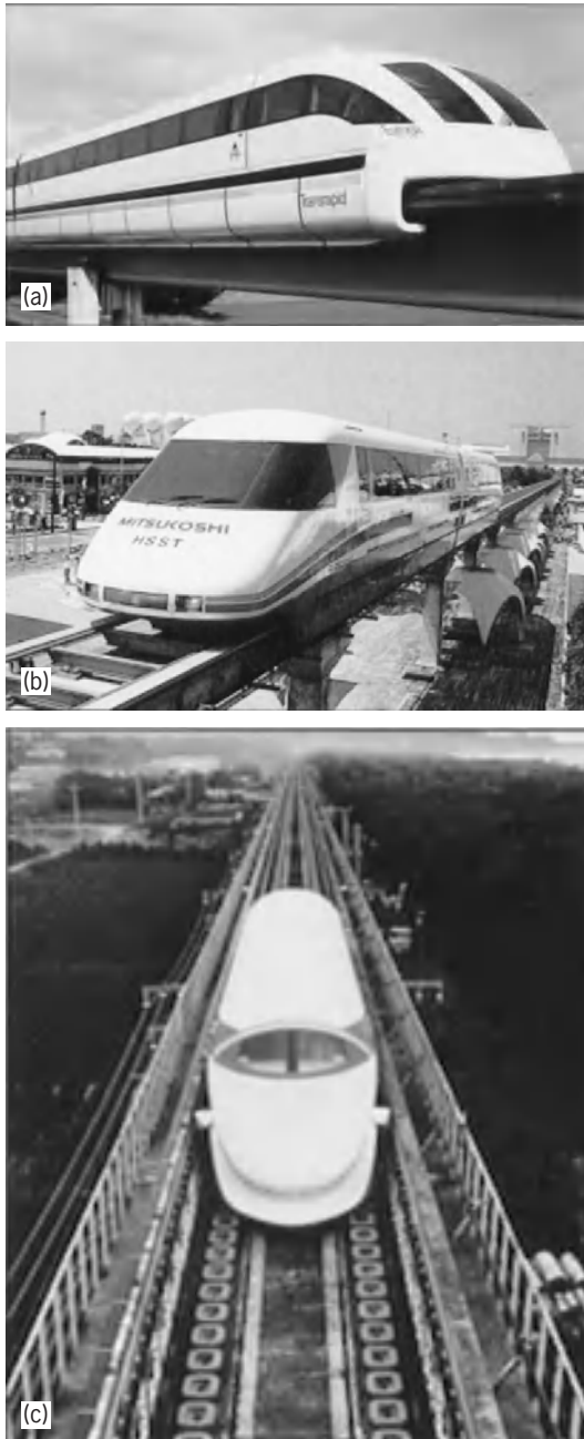
Fig. 3. Magnetic levitation systems and vehicles. (a) German Transrapid TR07 vehicle ( Thyssen Henschel, Munich ). (b) Japanese HSST system. (c) Japanese superconducting test vehicle MLU-002 ( HSST Corporation, Tokyo ).
