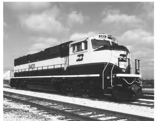
Fig. 1. Modern 4000-hp diesel-electric ac locomotive. (Electro-Motive Division of General Motors Corp.)
