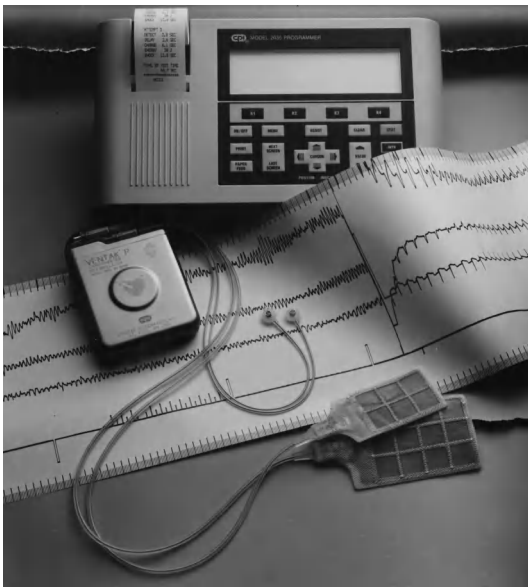
Fig. 5. Automatic implantable cardioverter defibrillator (AICD) system with pulse generator, leads, and external programmer. (S. Nisam, Cardiac Pacemakers, Inc.)
