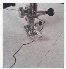
**2** Using a short stitch length, sew on the outside stitching line through all the layers. Sew along the inner appliqué lines, using a thread color matched to the appliqué fabric.
