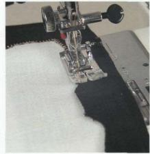
Reset the sewing machine for pin stitching in Step Two of Machine Set-Up. Remember to change your needle. Place a layer of tear-away stabilizer underneath the border and base fabric. Using the blade of the edgestitch foot as a guide, stitch the border in place.
