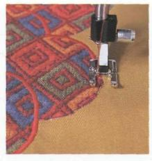
**5** Set your machine for Step Two, selecting a satin-stitch width appropriate to the size of the design. From the right side, stitch around the design following and covering the straight stitching.
