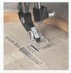
3 Lower the feed dogs, attach the darning foot, and adjust the machine settings for Step Two.
