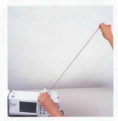
Using your free hand, pinch the twisted cords in the center. Bring the loose cord tail ends that are held in your other hand down to meet and touch the knot on the bobbin. Hold the cord tails and
