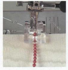
**2** Place the beads under the foot leaving a 4" tail in the back. Place a layer of tear-away stabilizer underneath the area to be couched. Adjust the stitch width to just pass over the beads.
