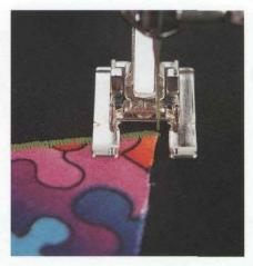
**6** When stitching outside corners, sew past the corner by one zig zag stitch. Stop with the needle swing in the outside edge of the satin stitching. Lower your needle into the fabric and pivot. Repostion the foot and continue to sew.
