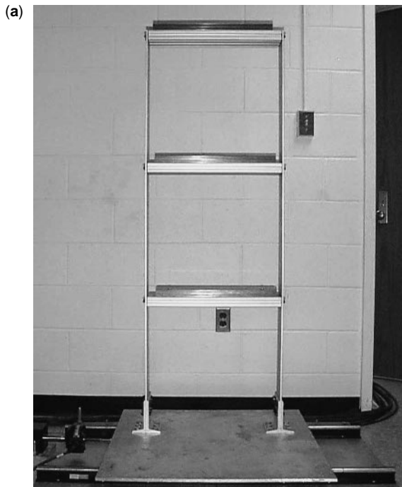
Figure 24. (a) Framed building structure. (b) Discrete three-DOF model.
