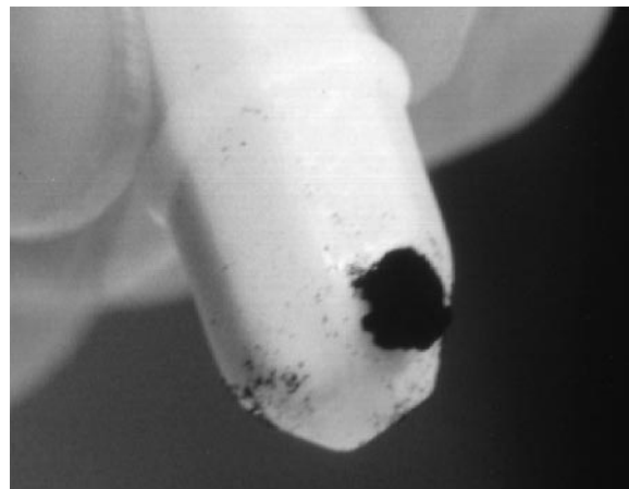
Figure 13. Sample of a \text{V}[\text{Cr}(\text{CN})_6]_y \cdot z\text{H}_2\text{O} magnet ( T_c = 372 K) attracted to a Teflon coated magnet at room temperature in the air (27a).
