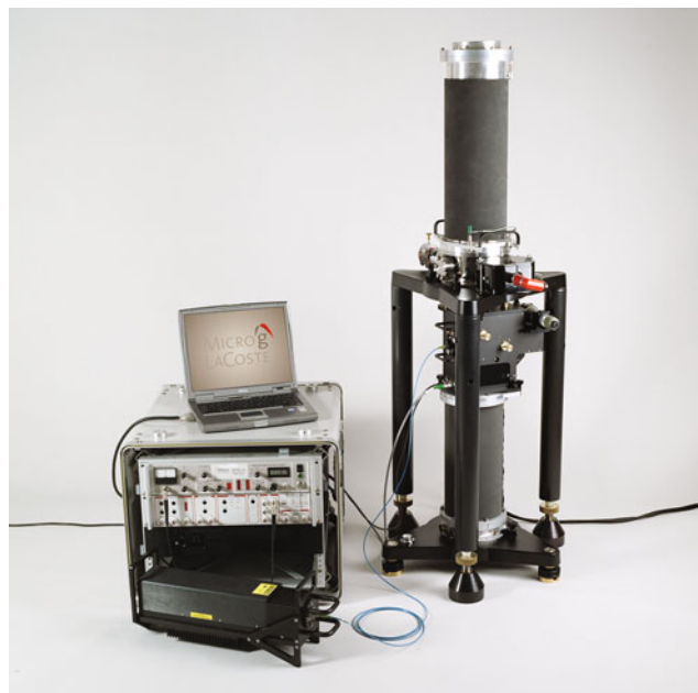
Gravity Measurements, Absolute, Figure 2 The micro-g LaCoste FG5 is a commonly used portable absolute gravity meter.
