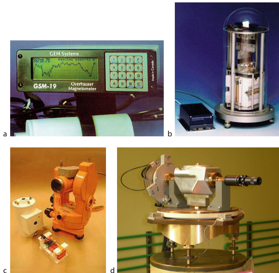
Geomagnetic Field, Measurement Techniques, Figure 1 Geomagnetic observatory sensor package: proton magnetometer (a), fluxgate magnetometer (b), theodolite with fluxgate coupled to the telescope (c). The new prototype of Geomagnetic AUtomatic SyStem (GAUSS) is also shown (d).
