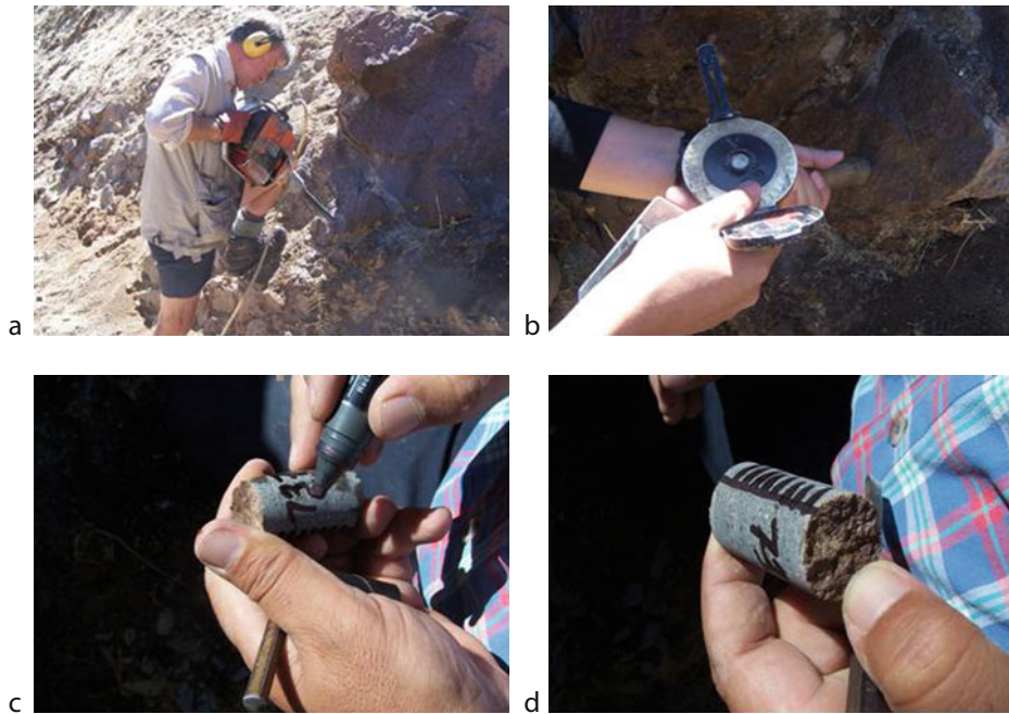
Paleomagnetism, Measurement Techniques and Instrumentation, Figure 2 Collecting and orienting rock samples for paleomagnetic study. The cores are drilled (a) with a portable motorized coring machine. (b) An orienting tool is inserted around the core to determine the inclination and the azimuth by Sun and magnetic compasses. (c) The core is extracted and coded. (d) A line on the core is used to fix the extracted core with respect to the orientation readings using a directed line on the top or the bottom.
