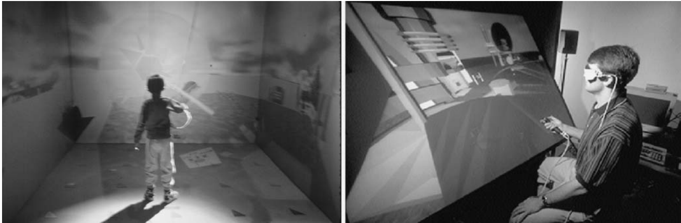
Figure 1: The CAVE and ImmersaDesk. (Left) A person in the CAVE wearing tracked shutter glasses to see the virtual world in stereo and carrying the wand. (Right) A user sitting in front of the ImmersaDesk wearing the same tracked glasses and carrying the same wand as in the CAVE. The CAVE and ImmersaDesk users can interact with the same virtual worlds from different perspectives.
