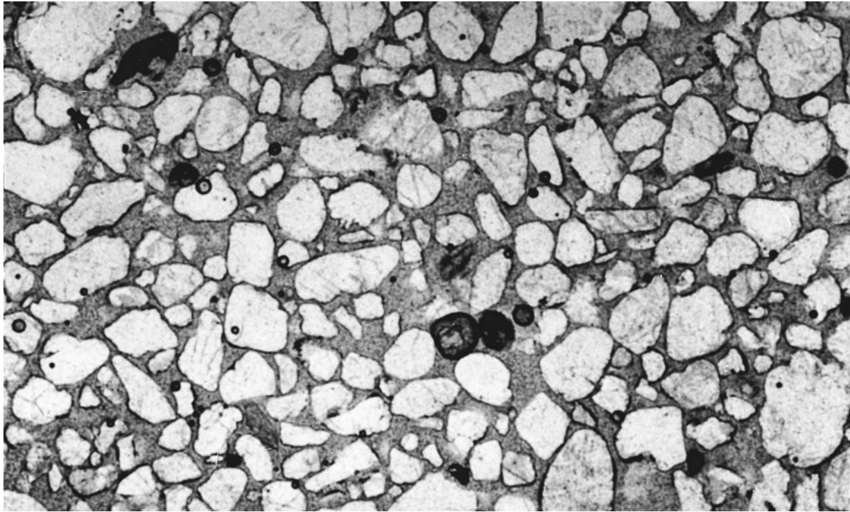
FIGURE 3 Photomicrograph of a thin section through a sandstone petroleum reservoir showing primary intergranular porosity between the quartz framework grains. (Simpson Group (Ordovician) Arbuckle Mountains, Oklahoma.) Width of photograph is 3 mm.
