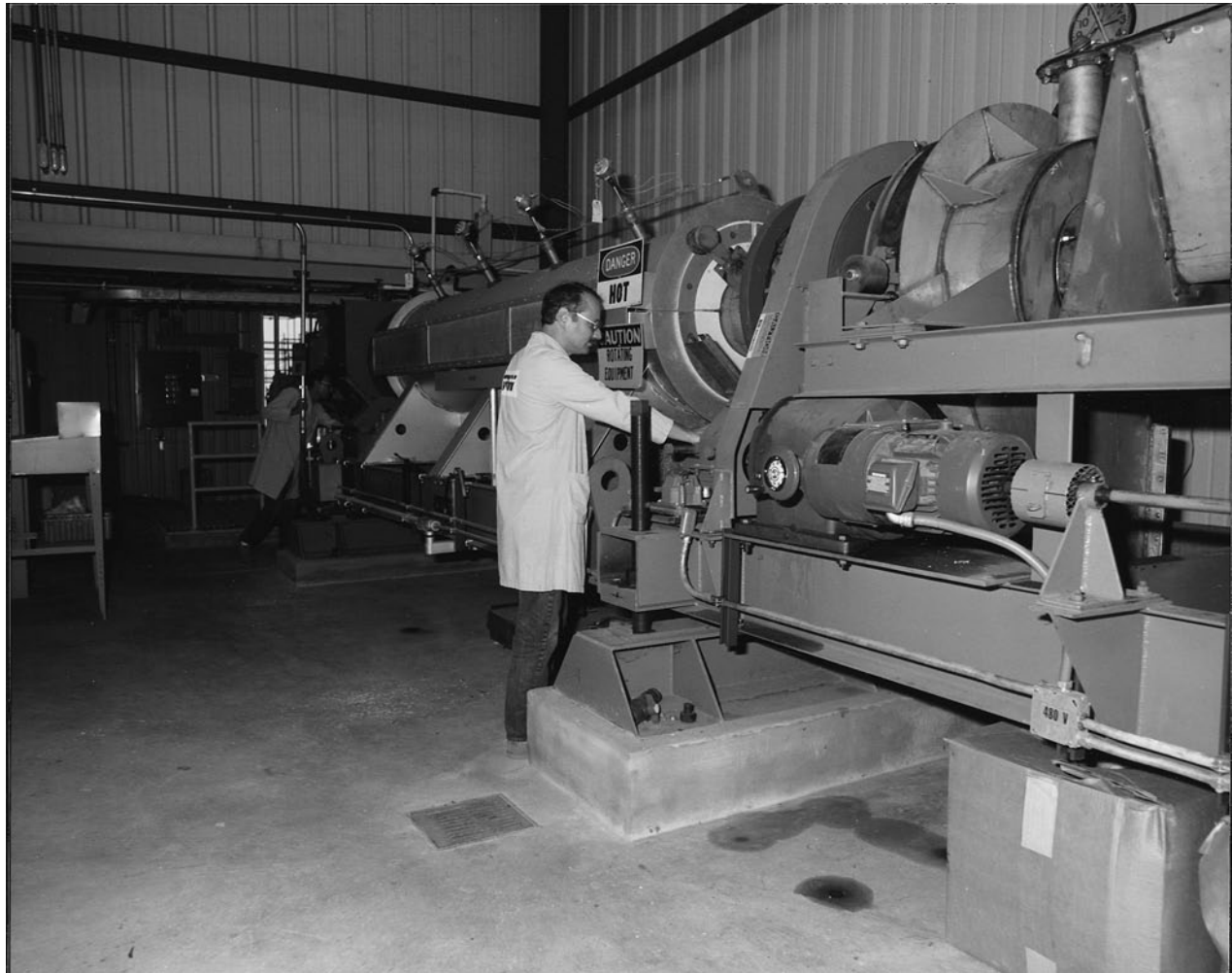
FIGURE 27 Rotary kiln reactor in operation at Gravimelt Test Plant Facility. The reactor consists of a 12-ft long furnace section, a 3-ft cooling zone, and a discharge area.
