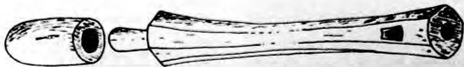
TOOLS. Figure 1. Kahun bow-driven drill stock, with its wooden drill cap. A tool can be removed by pushing a short stick into the ejection hole. (Drawn from Manchester Museum Catalogue number 23. Courtesy Denys A. Stocks)
