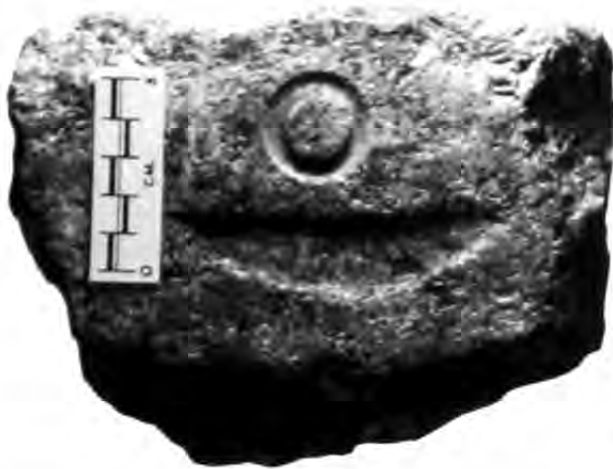
STONEMWORKING. Figure 3. The bilateral sign nb cut into granite by test flint punches and chisels. The sign was polished by sandstone grinders and drilling powders of the waste material.
