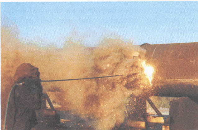
Figure O-12—Oxygen Lancing of a 102 cm (40-in.) Diameter Cast Iron Roll from a Paper Mill
