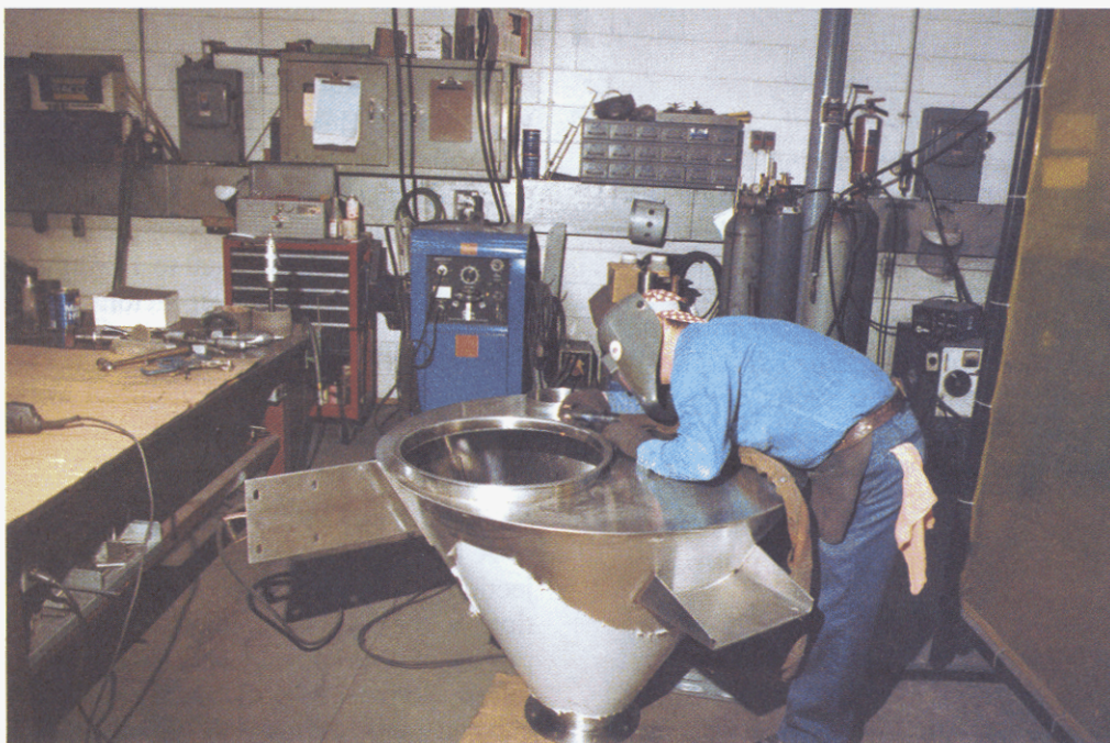
A welder uses the gas tungsten arc welding (GTAW) process to fabricate a hopper used in the food processing industry
