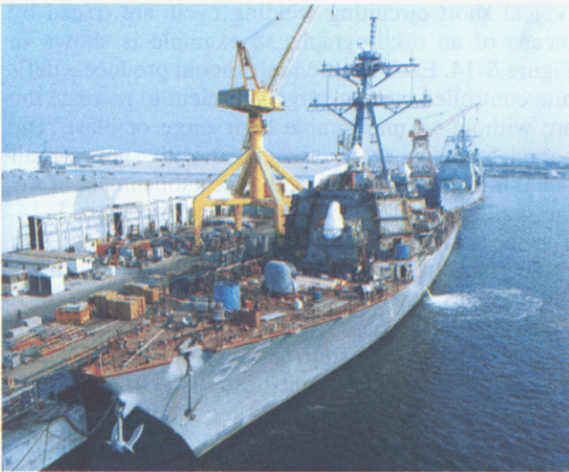
Figure S-13—Fitting Out an Arleigh Burke Class Aegis Destroyer in a Shipyard
