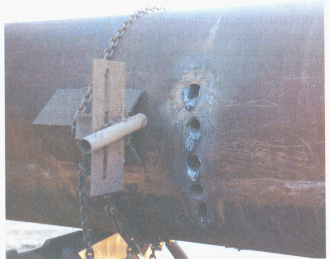
Figure O-13—Holes Pierced in a 102 cm (40-in.) Diameter Cast Iron Roll Using an Oxygen Lance
