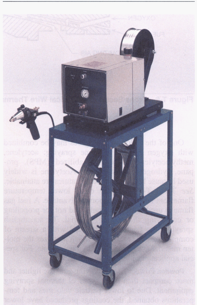
Figure T-5—Oxy-fuel Gas Wire Spray Equipment Capable of Spraying Wires Ranging from Low Melting Alloys (Babbitt) to Higher Melting Point Steels. Aluminum Wire Shown on Top Spool and Carbon Steel Wire on the Bottom Reel.
