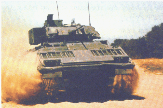
Figure C-6—Armored Vehicle Track Shoes Cast from an Aluminum Metal Matrix Composite will be Assembled into Treads for Field Tests on Vehicles such as this M551 Sheridan Light Tank
