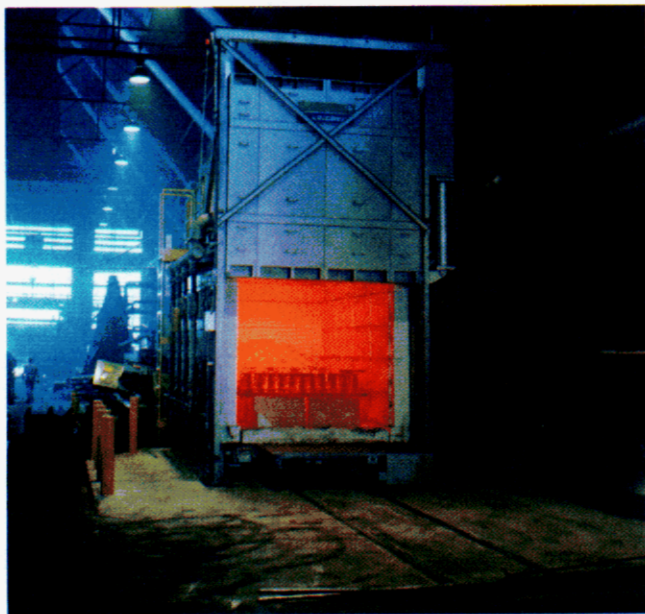
Figure S-26—A Gas-Fired Car Bottom Furnace Used for Stress-Relieving Steel Forgings up to a Maximum Operating Temperature of 1000°C (1800°F)
