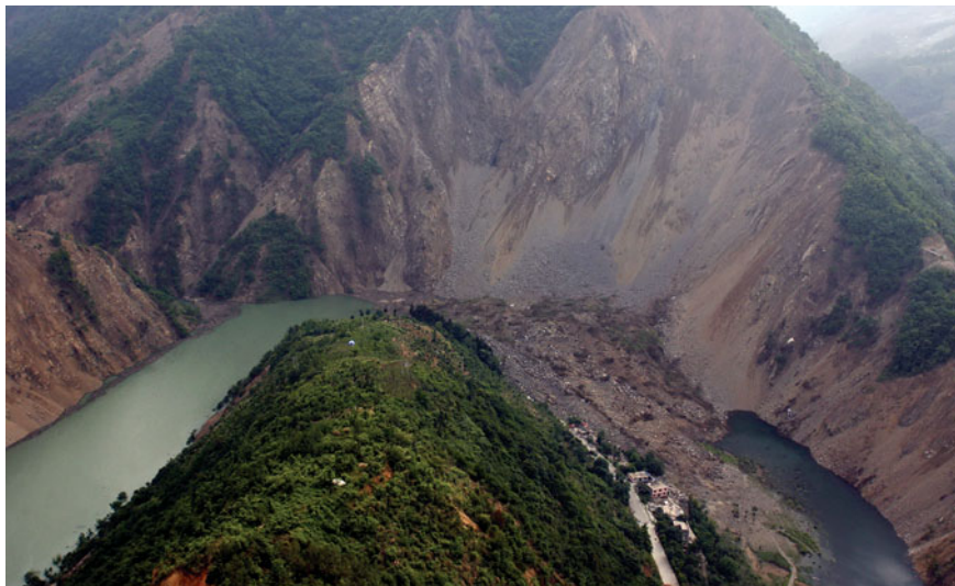
One of the many major landslides that was triggered by the Wenchuan (China) earthquake on May 12 blocked this river in the mountainous area near Beichuan. Engineers dug channels to drain water from the lake that rose behind the debris.
