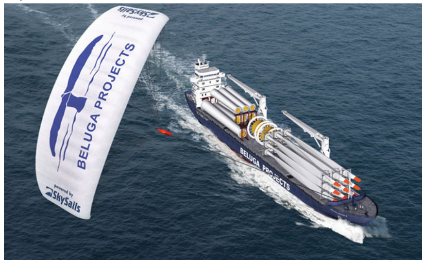
The world's first kite-assisted cargo ship the MV Beluga SkySails was chartered by the U.S. Navy to carry military supplies.
