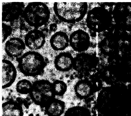
Fig. 5 Cryotransmission electron micrograph of poly(acrylic acid) hollow nanospheres obtained by polymerization method. (From Sauer, M.; Meier, W. RSC Chem. Commun. 2001 , No. 1, 55–56; reproduced by permission of The Royal Society of Chemistry.)
