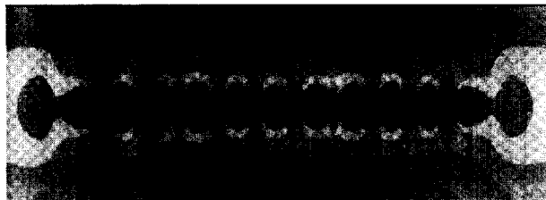
Fig. 4 Finite-difference time-domain simulation of electric fields (red) localized within a linear array of 50-nm Au particles (blue), with interparticle separations of \delta=75 nm. (From Ref. [23].) (View this art in color at www.dekker.com .)
