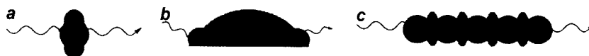
Fig. 1 Incident light on nanostructured metal surfaces can result in localized (standing) plasmon resonances (a), propagation of surface plasmon waves (b), or a combination of the two (c). Excitation of conduction electrons produces local electromagnetic fields (pink) near the metal surfaces. (View this art in color at www.dekker.com .)
