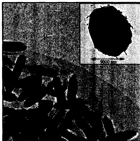
Fig. 10 Transmission electron microscopy image of Fe-based precipitates (240-nm elongated iron oxide particles) in capsules filled with PAH.
