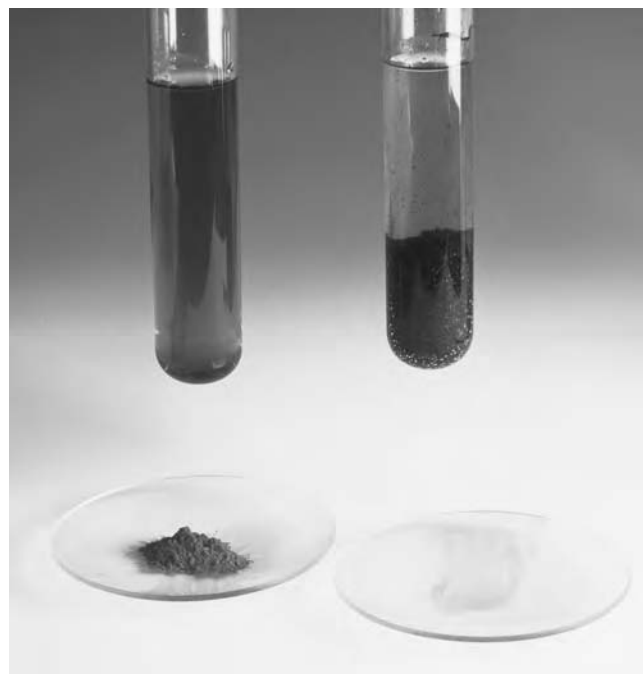
Demonstration of an electron-transfer reaction in a laboratory. At left is a test tube containing copper(II) sulfate solution; below this is a watch glass containing zinc powder. When the zinc is added to the sulfate, the solution loses its blue color (right). This is due to the electron transfer between copper(II) ions (blue) and the zinc to form zinc(II) ions (colorless). The copper is deposited as a metal. (Courtesy of Jerry Mason/Science Photo Library)
