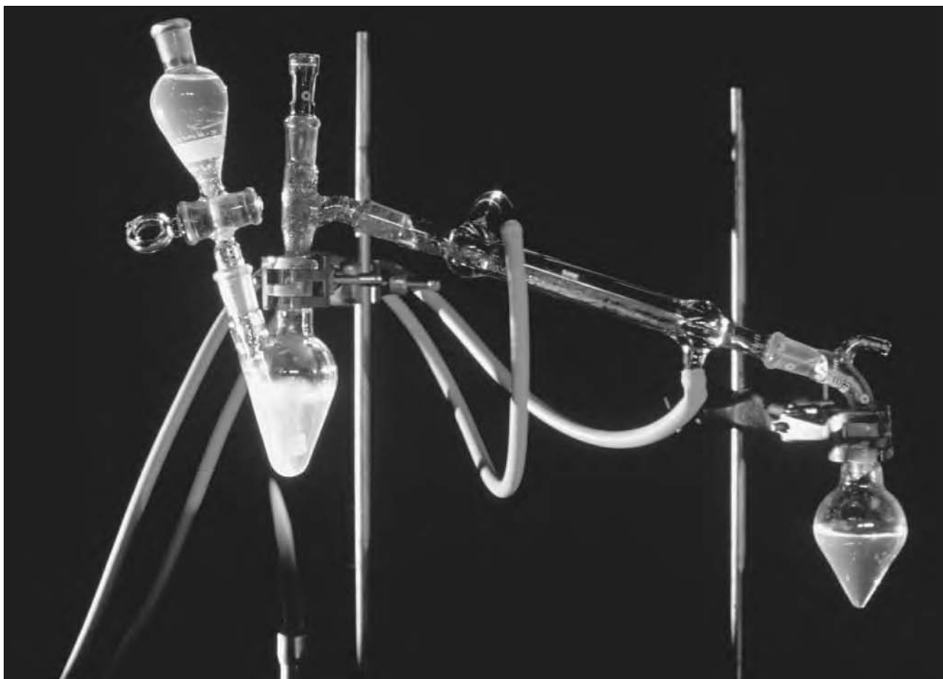
Apparatus used for chemical distillation. The liquid in the left-hand bulb is heated over a Bunsen burner, and a reagent is added from the flask above it. The products of the ensuing chemical reaction can then be separated by distillation. The most volatile compound will boil off at the lowest temperature. Its vapor passes into the condenser, a tube that is surrounded by a cooling water jacket. The hot vapor cools and condenses on the walls of the tube and is then collected in the "receiver" flask on the right of the photo. (Courtesy of David Taylor/Science Photo Library)
