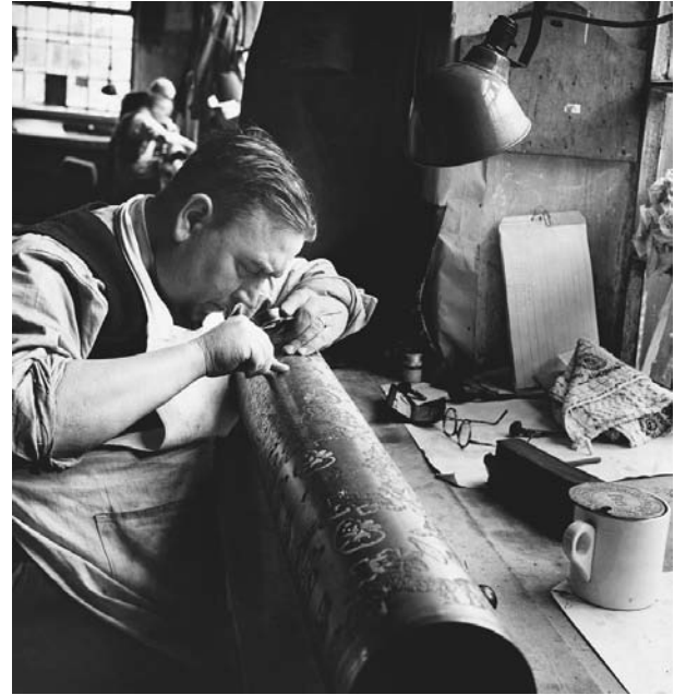
An engraver puts a design onto a printing roller. Hand-painted calico was very time-consuming and expensive to produce, and processes for printing and dyeing calico fabric were developed during the eighteenth and nineteenth centuries.
