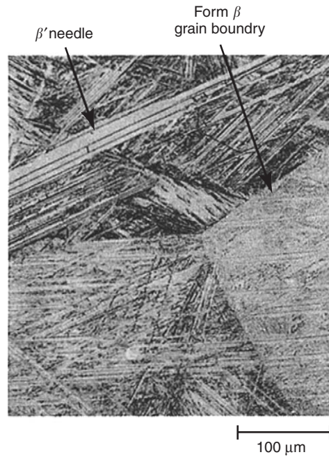
Figure 23 Martensitic structure of Cu–11.8% Al after rapid cooling from 800°C. (Adapted from ASM (2001) Copper and Copper Alloys , ASM Specialty Handbook, p. 48. Materials Park, OH: ASM.)
