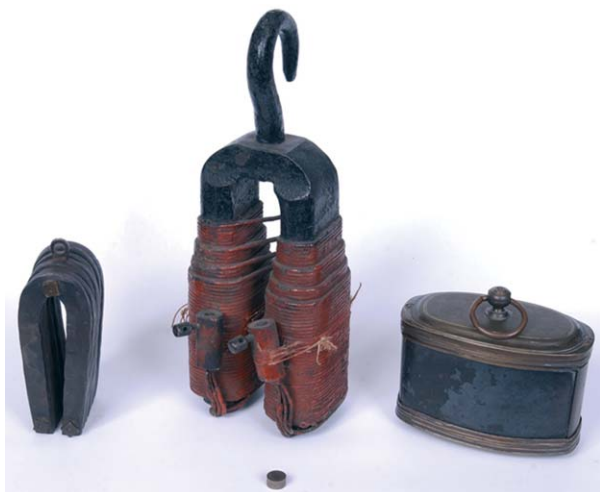
Figure 4 Four centuries of magnets shown clockwise from the left: eighteenth-century horseshoe magnet; nineteenth-century electromagnet; seventeenth-century lodestone; and twentieth-century \text{Nd}_2\text{Fe}_{14}\text{B} .
