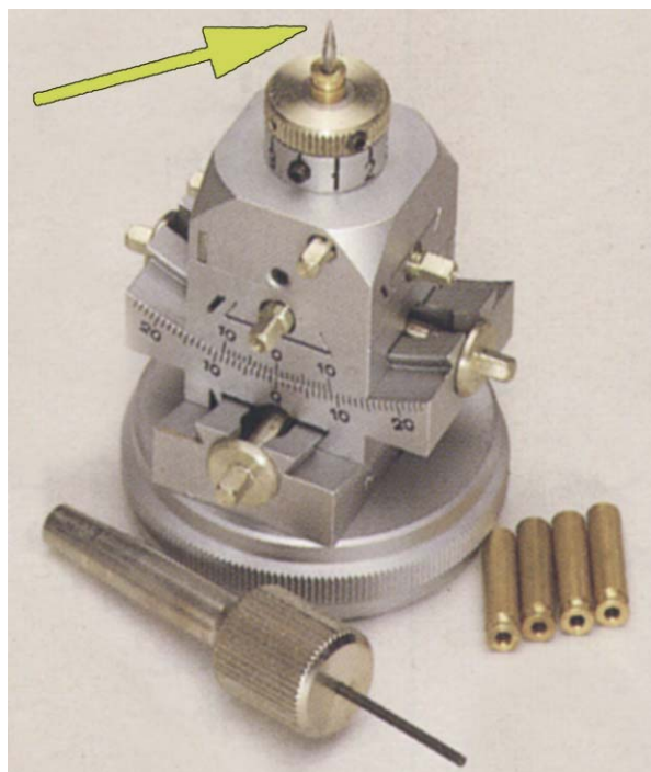
Figure 6 A goniometer head. The arrow shows the location of the crystal. (Reproduced with permission from Huber Diffraktionstechnik, Rimsting, Germany.)
