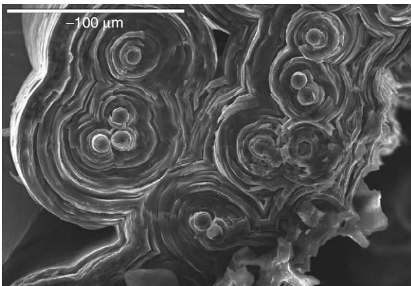
Figure 5 Scanning electron microscope image of CVD carbon layers deposited around fibers within a carbon-carbon composite.
