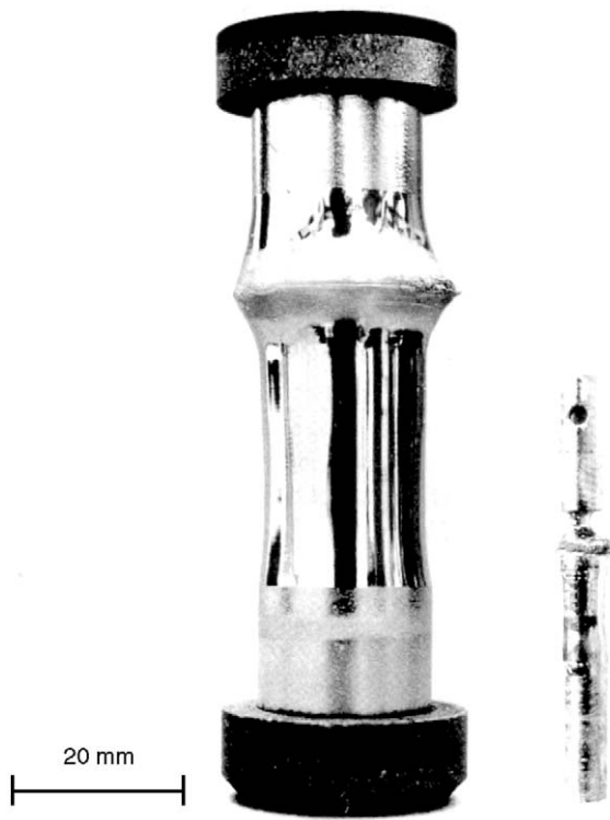
Figure 18 GaAs crystals grown by the FZ technique; left: sample grown in space under microgravity during the German Spacelab mission D2, right: sample grown on earth with maximum size. (Source: Crystal Growth Laboratory, Fraunhofer IISB, Erlangen.)
