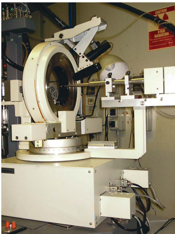
Figure 7 A single crystal 4-circle diffractometer using a rotating anode X-ray source (Istituto di Cristallografia – Sezione di Monterotondo, Rome, Italy). (Reproduced with permission from Huber Diffractionstechnik, Rimsting, Germany.)
