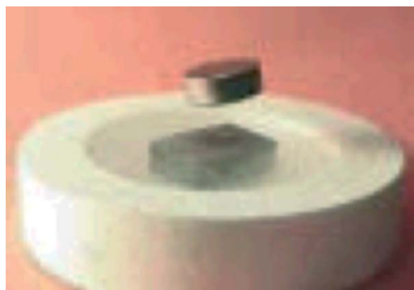
Figure 1 Magnetic levitation of a magnet about a YBCO sample.
