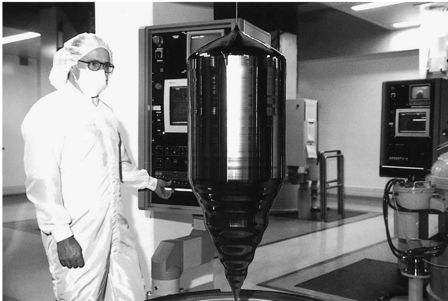
Figure 14 A single crystal ingot of silicon having a diameter of 300 mm. Such an ingot is sliced horizontally into circular wafers whose surfaces become the site of integrated circuits. (Courtesy of H Fusstetter of Wacker and Siltronic AE.)
