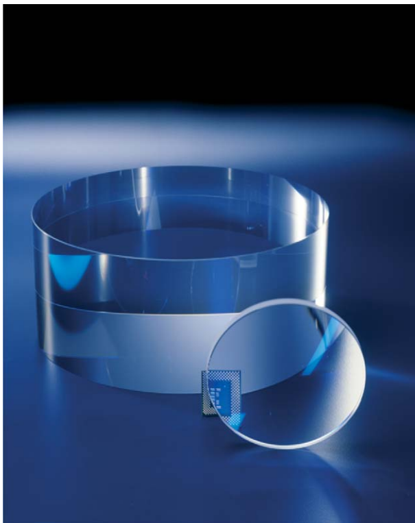
Figure 12 \text{CaF}_2 crystals as lense material for the micro-lithography are grown by modified Bridgman–Stockbarger methods. (Source: SCHOTT Lithotec.)
