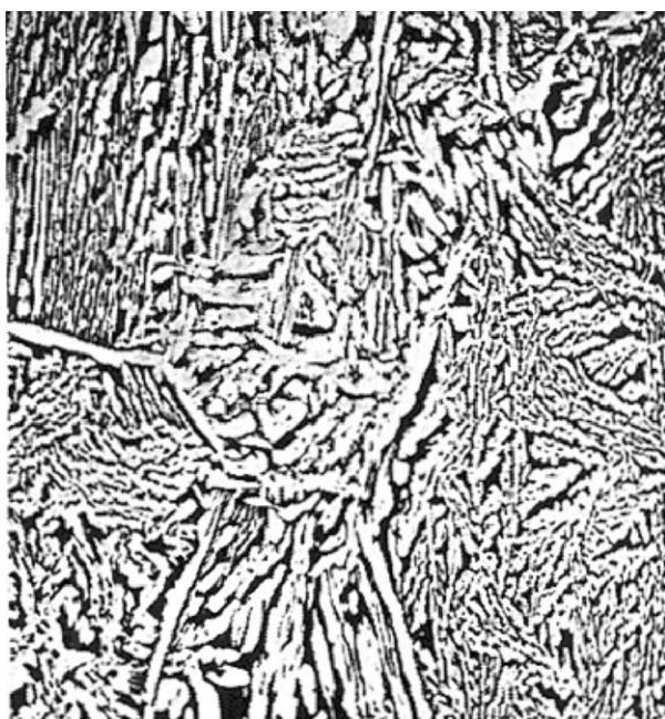
Figure 19 Photomicrograph of a Muntz metal (40% Zn) after air cooling. The dark phase is \beta and the light phase is \alpha , which has precipitated during cooling. (Adapted from Brick RM, Gordon RB, and Phillips A (1965) Structure and Properties of Alloys . New York: McGraw-Hill.)
