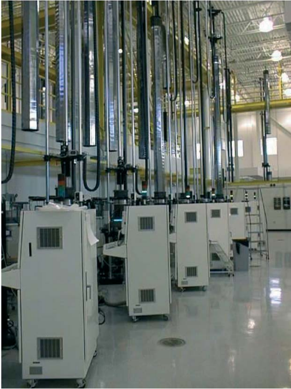
Figure 10 Silicon octagons grown by the EFG method. (Reproduced from Kalejs JP (2002) Silicon ribbons and foils – state of the art. Solar Energy Materials and Solar Cells 72(1–4): 139–153, with permission from Elsevier.)
