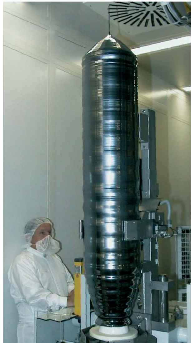
Figure 3 Silicon crystal with a diameter of 300 mm and a weight exceeding 250 kg, grown by the Cz method. (Reproduced with permission from Siltronic.)
