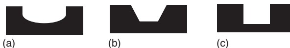
Figure 1 Semiconductor shapes obtained with diverse etching techniques. (a) Isotropic etching; (b) Anisotropic etching – dependent on orientation; (c) Anisotropic etching – independent of orientation.
