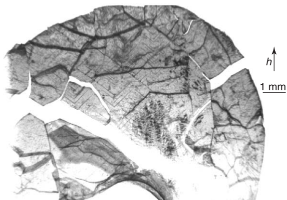
Figure 7 White beam topograph of an Fe-3%Si crystal, E \approx 25 keV, showing orientation contrast associated with sub-grains. A fir-tree magnetic domain pattern is also visible.
