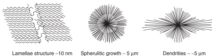
Figure 2 Chain folding in poly(ethylene) leading to lamellae formation and a pictorial representation of spherulitic growth.
