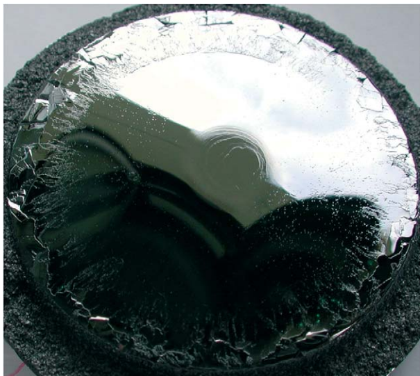
Figure 23 SiC crystal with 50 mm diameter grown by the PVT method. (Reproduced with permission from Institute for Material Science, Department of Electrical Engineering Materials, University Erlangen-Nuernberg.)
