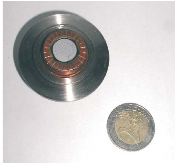
Figure 2 The cathode (gray disk) assembly of an S-band Linac gun. (Courtesy of Sincrotrone Trieste.)
