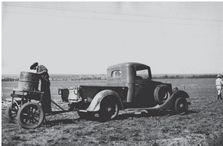
Food-Based Poisoned Baits for Insect Control, Figure 66 If bait distribution is to be accomplished on a large scale, some type of machinery is usually needed. Shown here is a primitive (but effective) bait spreader used in the 1937 grasshopper suppression effort in Colorado. Ground distribution of bait was soon replaced by aerial application, and both solid and liquid baits are now generally applied by air if the land area to be treated is extensive.
