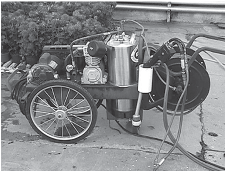
Insecticide Application: The Dose Transfer Process, Figure 13 The Electrostatic Spraying Systems Inc. EPS-5 sprayer. The sprayer delivers a fine mist that is electrically charged and forced into the canopy by compressed air.
