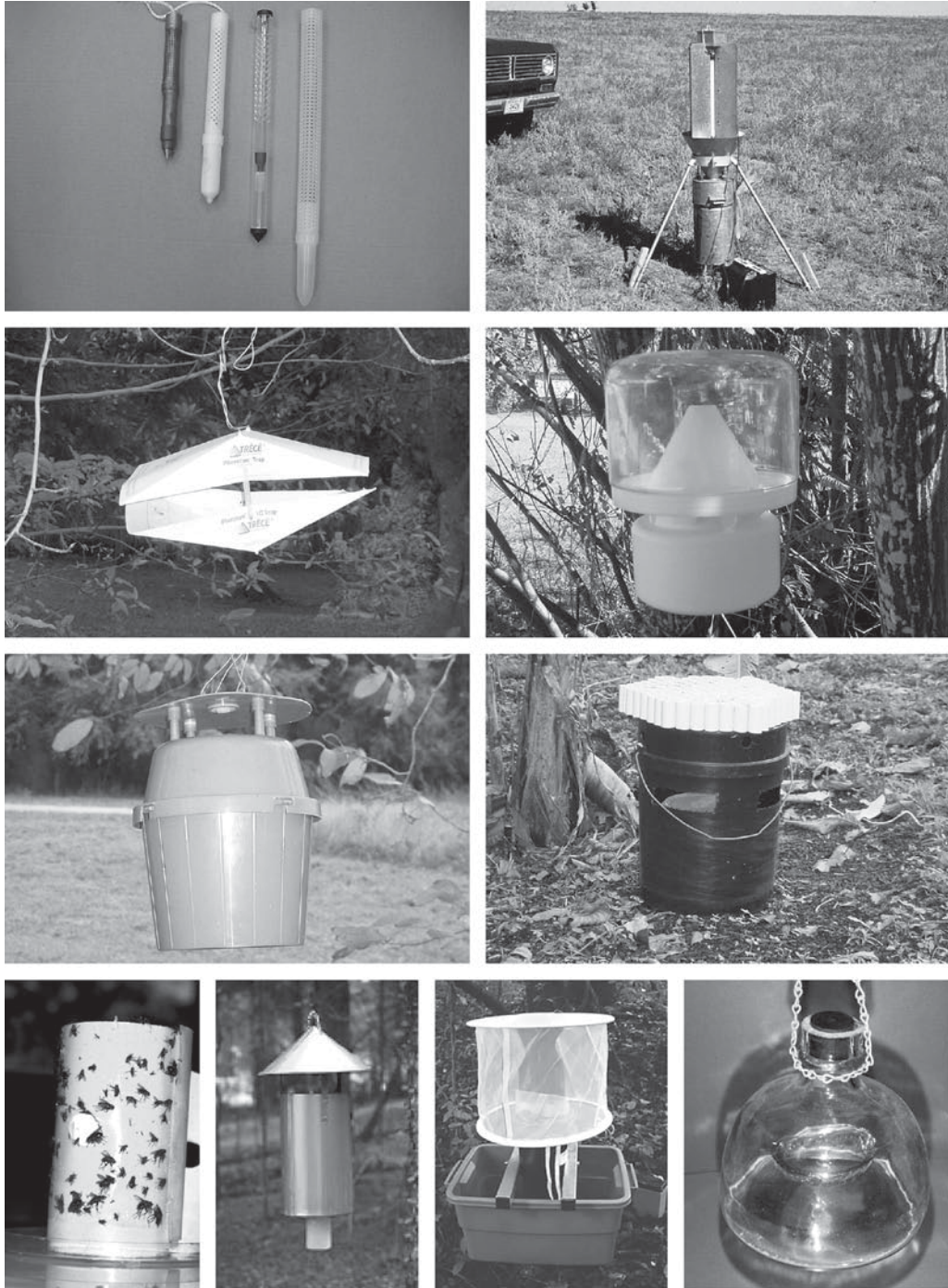
Traps for Capturing Insects, Figure 98 Additional insect traps: top left , grain probe traps for detection of stored grain insects; top right , blacklight trap for detection of nocturnal flying insects; second row left , wing trap, a lure-based trap with a sticky interior for sampling flying insects; second row right , wasp trap, a food lure-based trap; third row left , unitraap, a popular pheromone-based trap for capture of moths; third row right , a bucket trap baited with pineapple and pheromone for capture of palm-infesting weevils; bottom left , a cylindrical yellow panel coated with adhesive for detection of flying insects; bottom second from left , New Jersey light trap for capturing mosquitoes; bottom third from left , mosquito emergence trap; bottom right , McPhail trap, a food lure-based trap for capture of fruit flies.
