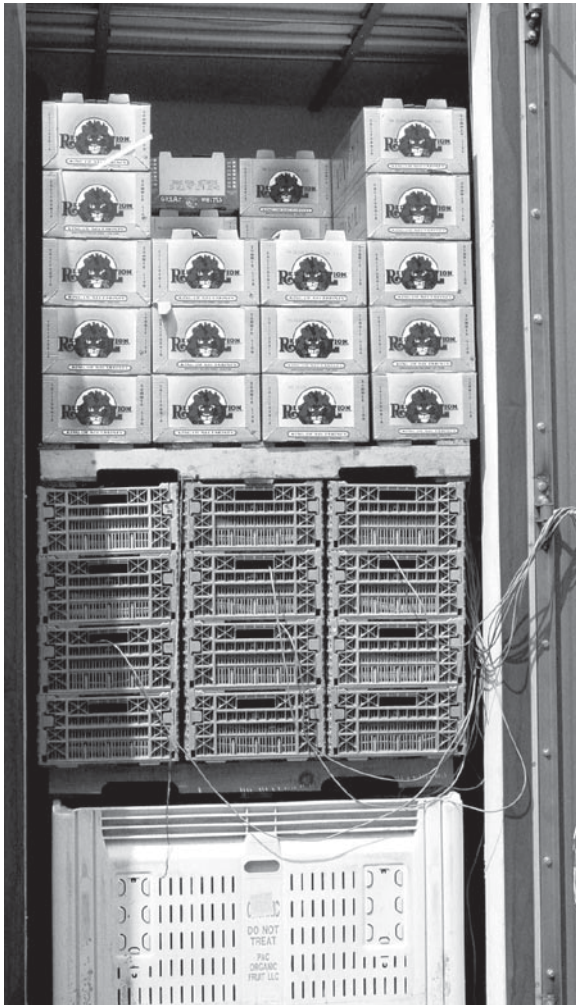
Controlled Atmosphere Technologies for Insect Control, Figure 98 A commercial CATTs (controlled atmosphere temperature treatment system) can accommodate various types of produce and packaging, and produce insect-free products.
