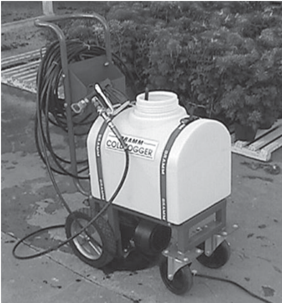
Insecticide Application: The Dose Transfer Process, Figure 12 The DRAMM Coldfogger sprayer for greenhouse pest management. The sprayer delivers a fine mist under high pressure.
