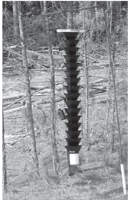
Visual Attractants and Repellents in IPM, Figure 22 Black cylindrical funnel traps mimic the silhouette of pine trees and are used, in conjunction with odor baits, to capture bark beetles (photograph by J. Foltz).
