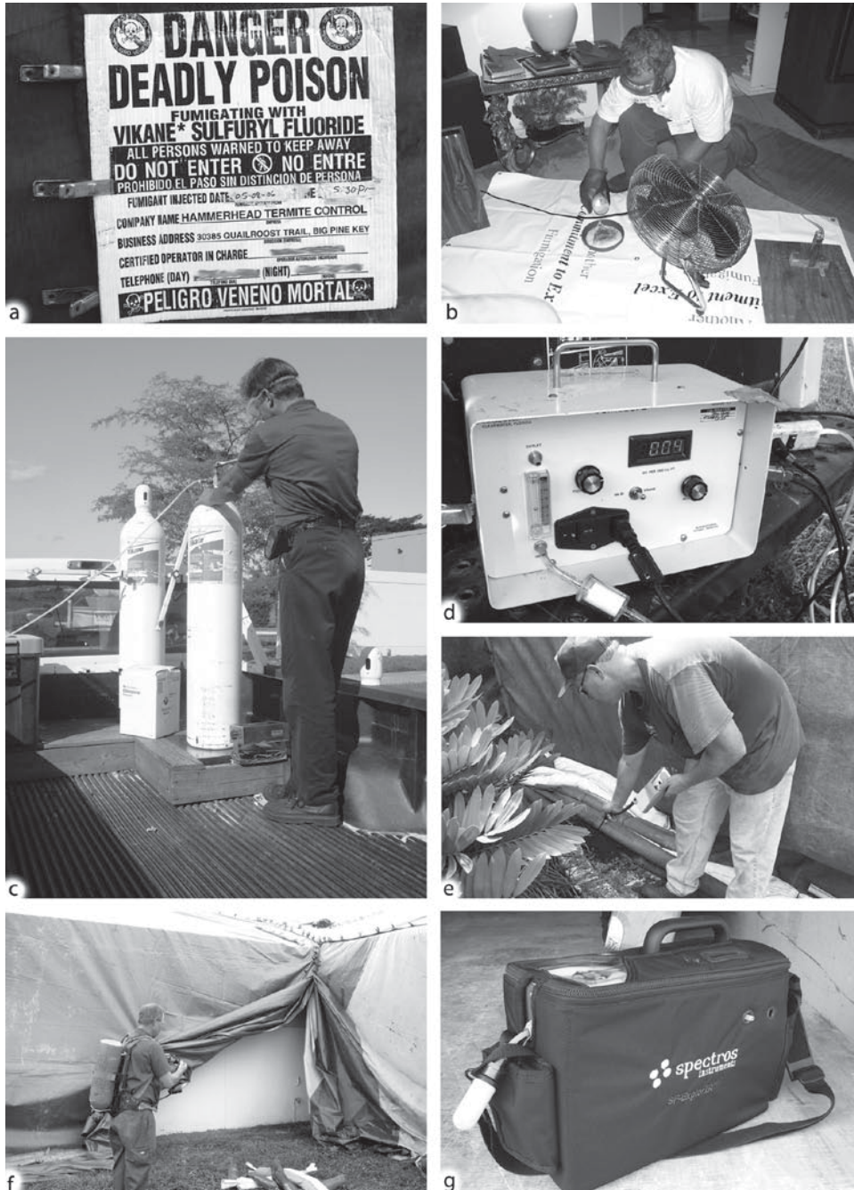
Structural Fumigation, Figure 146 Fumigation, continued: (a) warning signs should be placed on all sides of the structure, (b) liquid chloropicrin is poured into an evaporation pan placed next to a fan and the outlet of the sulfuranyl fluoride release hose, (c) sulfuranyl fluoride is released as a liquid. Upon exiting the end of the release hose, the liquid boils and spontaneously turns into a gas at atmospheric temperature and pressure, (d) Fumiscope ® used to measure working concentrations of fumigant, (e) halogen leak detector is useful for finding leaks in the seal of a fumigated structure, (f) initial aeration requires that the fumigator enters the building to open doors wearing a self-contained breathing apparatus, (g) gn Explorer IR clearance detector can measure down to 1 ppm sulfuranyl fluoride.
