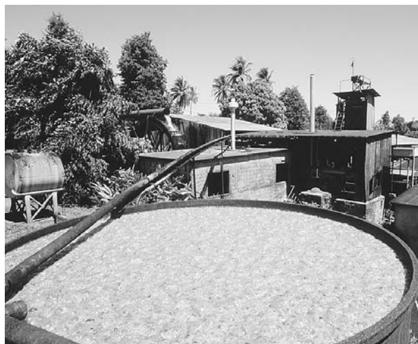
Sugar products are shown fermenting in an open tank at a rum distillery in Guadeloupe. © REINHARD EISELE/CORBIS.
