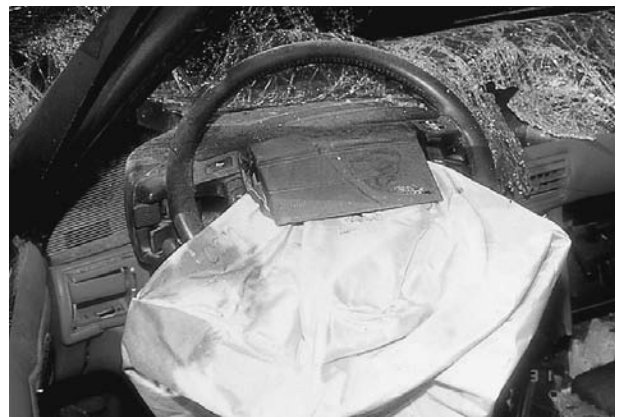
Figure 2 The injury-producing components of the air bag system are the air bag and the module cover which overlies it.
