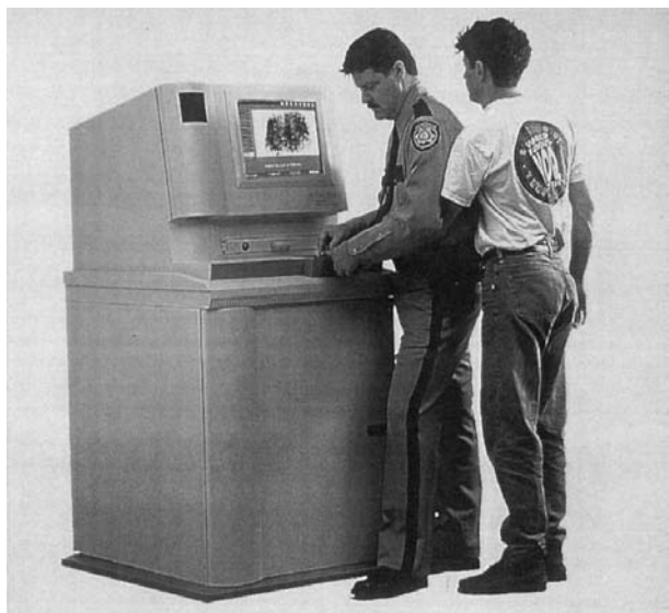
Figure 6 Livescan station for electronic recording of fingerprints. Courtesy Printrak International.
