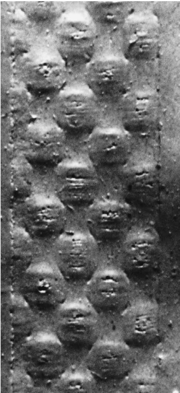
Figure 10 Cast of the sealed surface on the opposing side of the plastic bags sealed with the heat sealer (Figs 8 and 9). The Teflon-coated cloth material which covers the heating element (on the base of such heat sealers) will also be quite different from one sealer to another, with defects developing during use.
