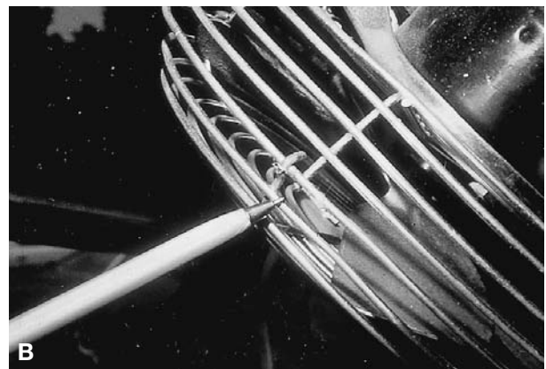
Figure 21 (A) There is a fan on the roof of the trailer cab (Fig. 20). (B) Close examination of the left side of the fan revealed the presence of trace evidence, including blood and tissue. Based upon a 90° rotation to the right, the occupant kinematics of the collision would dictate that the driver could impact the fan and it would be impossible for the passenger to make contact with the left side of the fan.
