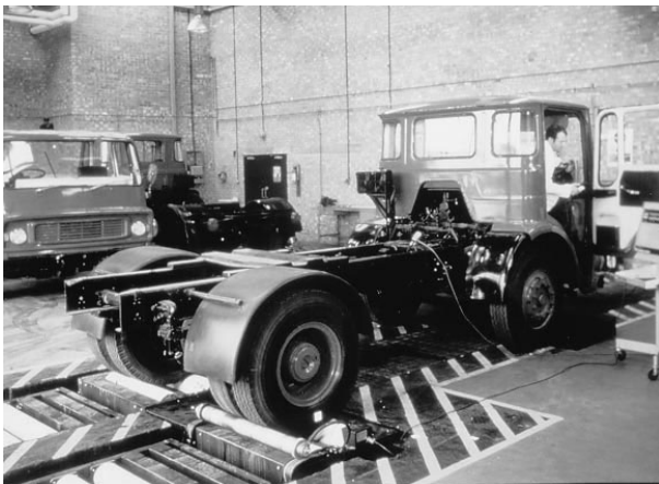
Figure 10 Calibration of a tachograph installation on a Hartridge Rolling Road. (VDO Kienzle (UK) Ltd)
