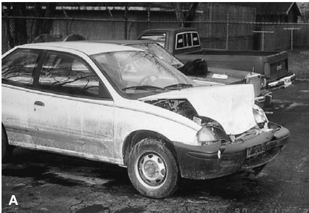
Figure 12 (A) and (B) A 1995 GEO Metro with minor front-end damage consistent with an impact speed of less than 15 k.p.h. (9 m.p.h.).
