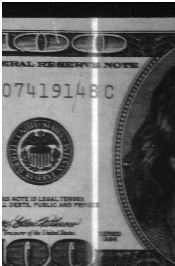
Figure 11 (see color plate 29) Fluorescence of counterfeit $100 FRN simulated security thread.
