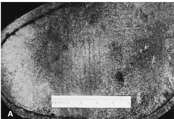
Figure 10 (A) Examination of leather-soled shoes may reveal the presence of a pedal imprint. (B) The shoe reflects an imprint from the vehicle's brake pedal and indicates that the wearer of the shoe was, in fact, the driver.
