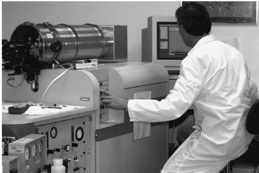
Figure 10 Dr Mark Kirms examines blood stains by electrospray mass spectrometry to determine species identities from hemoglobin molecular weights.
