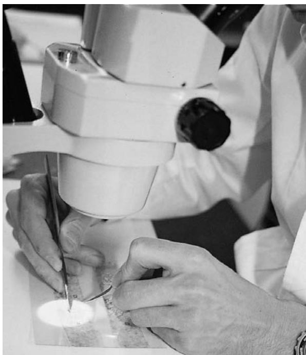
Figure 3 (see color plate 22) Searching for and removing matching fibers from surface debris tapings using stereomicroscopy.
