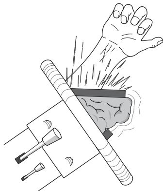
Figure 4 A diagrammatic representation of a forearm injury from contact with the deploying air bag module cover. This will give rise to the fracture pattern seen in Fig. 5.
