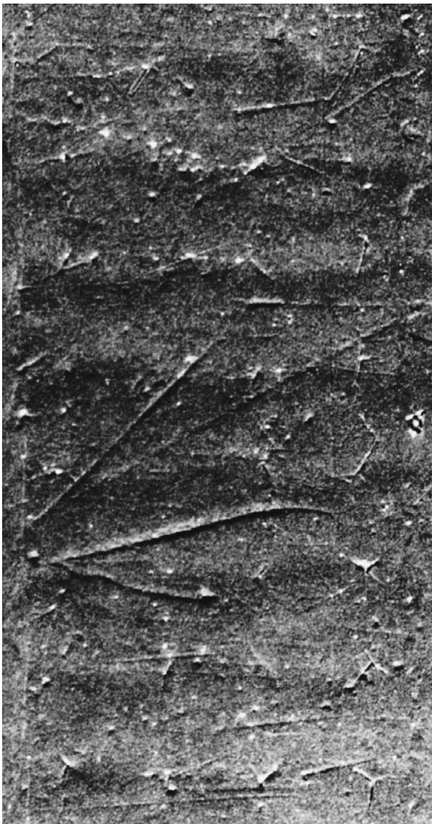
Figure 8 A cast of one small section of the seal produced on a plastic bag.
