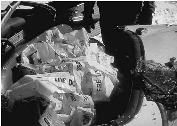
Figure 19 The interior of the vehicle (Fig. 18) was contaminated with vehicle components and scene evidence tape. The investigating agency took no steps to preserve or protect the integrity of trace evidence within the interior of the vehicle.
