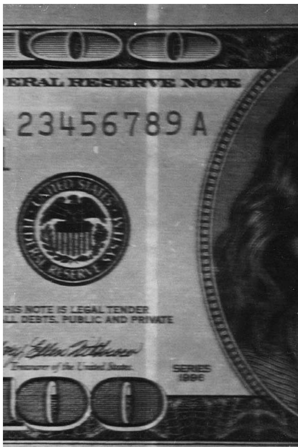
Figure 10 (see color plate 28) Fluorescence of genuine US $100 FRN security thread.
