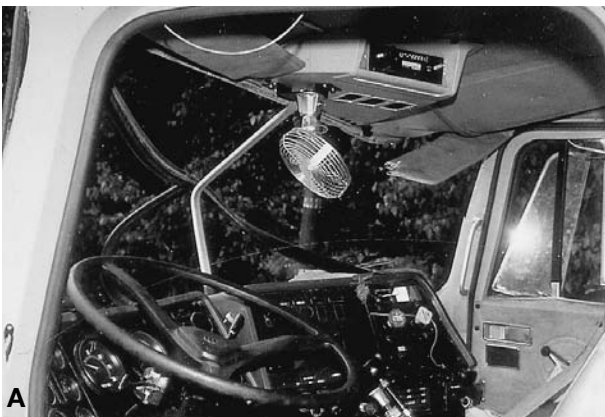
Figure 21 (A) There is a fan on the roof of the trailer cab (Fig. 20). (B) Close examination of the left side of the fan revealed the presence of trace evidence, including blood and tissue. Based upon a 90° rotation to the right, the occupant kinematics of the collision would dictate that the driver could impact the fan and it would be impossible for the passenger to make contact with the left side of the fan.
