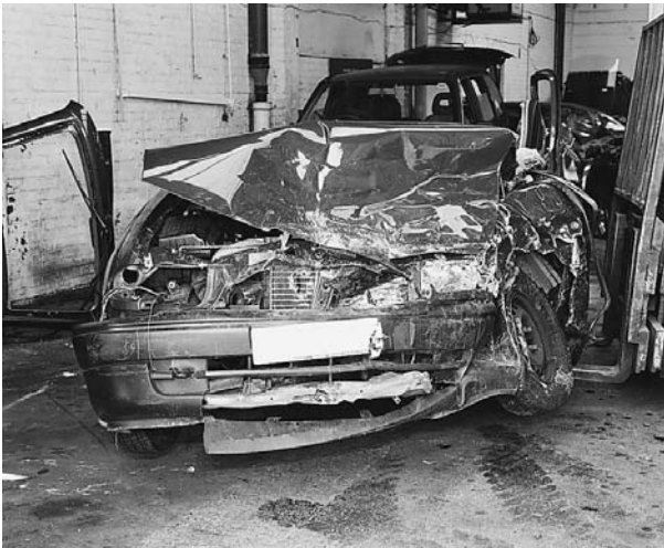
Figure 2 The relative position of this car and the one that struck it can be deduced from the damage to the front. © Metropolitan Police Service.
