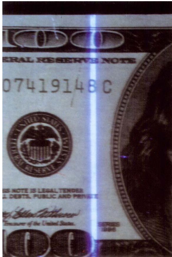
Plate 29 FORGERY AND FRAUD/Counterfeit Currency Fluorescence of counterfeit $100 FRN simulated security thread.
