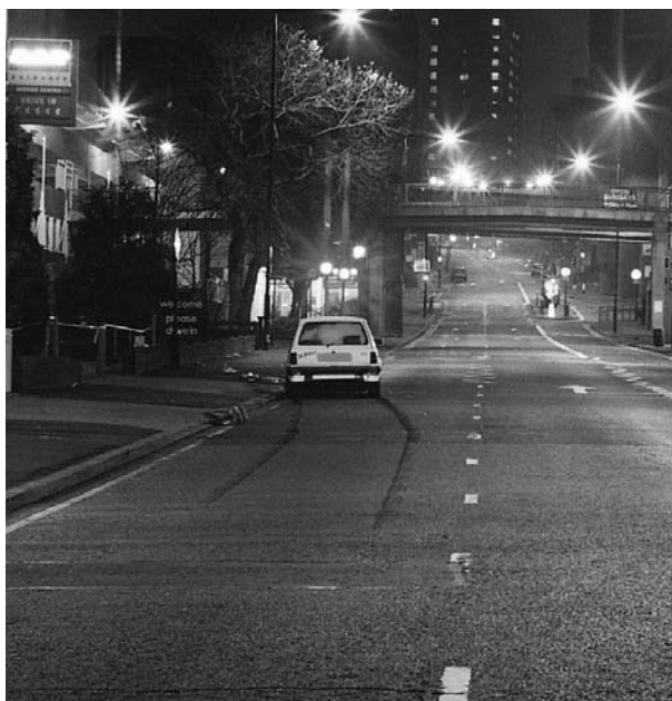
Figure 4 This car left two clearly defined skid marks which deviate sharply to the left part way along. This indicates the point of impact with the victim. © Metropolitan Police Service
