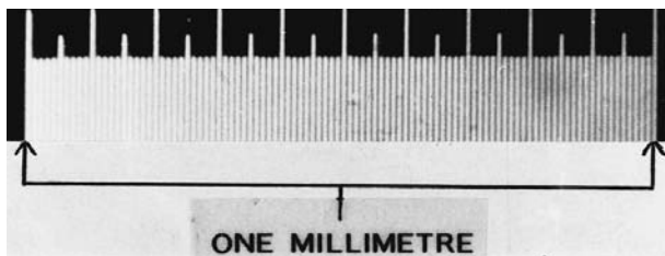
Figure 7 A 1 mm scale included here to give some indication of size. While these marks were only one-tenth the size of the marks in Case study 4 (the letter stamps), electron microscopy was found quite unsuitable for demonstrating the striae comparison results.
