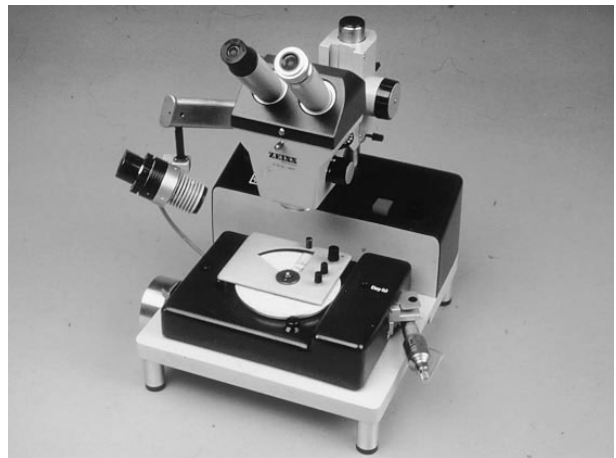
Figure 8 (see color plate 6) The Kienzle microscope with computer-linking modifications (VDO Kienzle (UK) Ltd).
