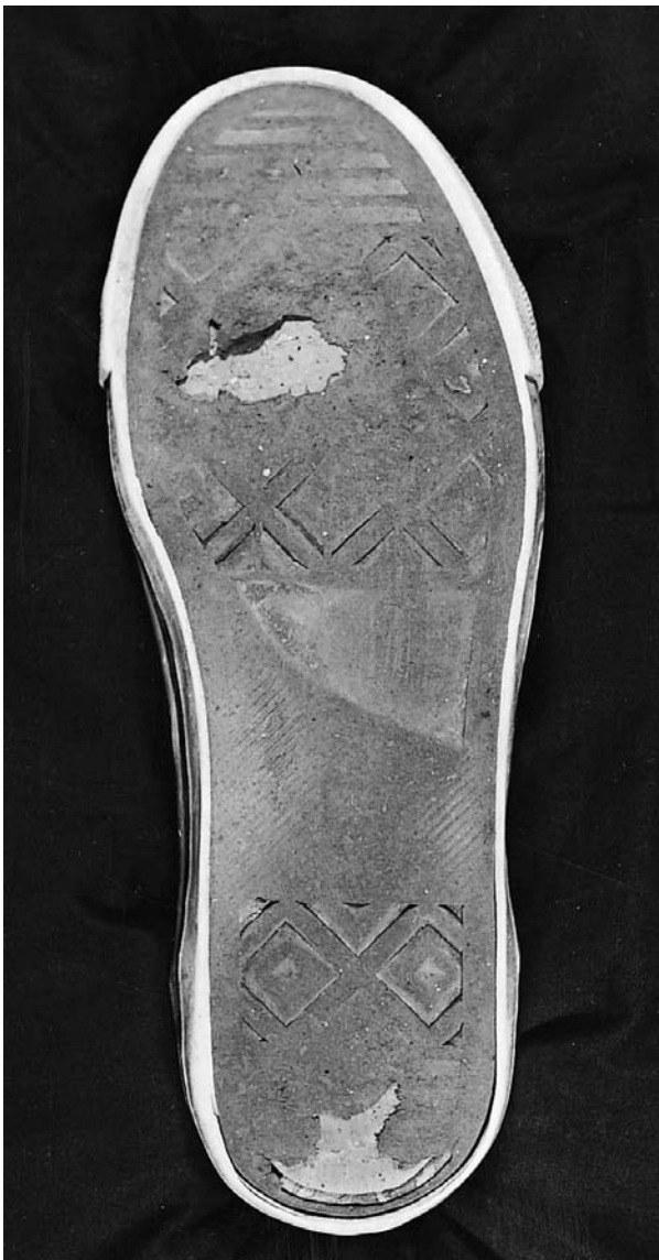
Figure 2 (see color plate 40) Outsole of a running shoe, showing wear areas on the ball of the foot and the heel.
