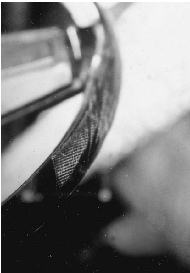
Figure 13 Forceful contact of clothing to vehicle components may impart a fabric transfer. A fabric imprint is noted on the steering wheel. Comparison of the weave pattern on the patient's pants to the pattern on the steering wheel confirmed the patient's role as the driver.
