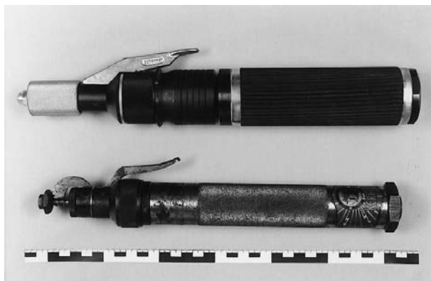
Figure 1 Two makes of captive-bolt stunners. Top: Schermer type (mod. ME, cal. 10 × 11 mm, diameter of the bolt 12 mm); bottom: Kerner type (mod. 289, cal. 9 × 17 mm, diameter of the bolt 11 mm).
