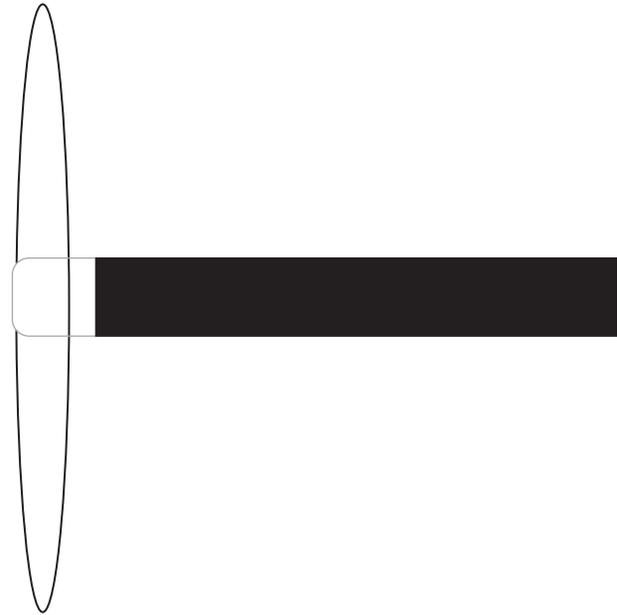
**FIGURE 1** Diagram of radial scanning echoendoscope showing the US scanning plane perpendicular to the shaft of the scope. Reproduced with permission from Rosch and Classen (1992).
