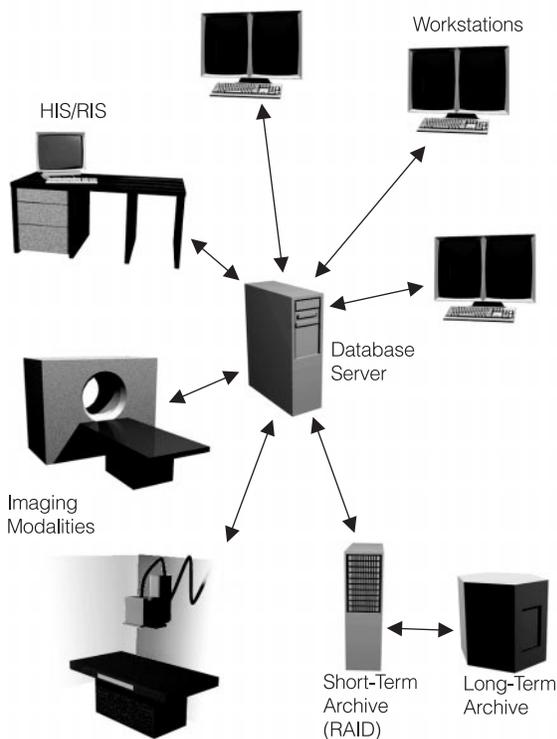
**FIGURE 1** An example of a basic PACS configuration. HIS, Hospital information system; RIS, radiology information system; RAID, redundant array of inexpensive disks. © ECRI (2000). Reprinted with permission from *Health Devices* 2000 Nov; 29(11): 387.
