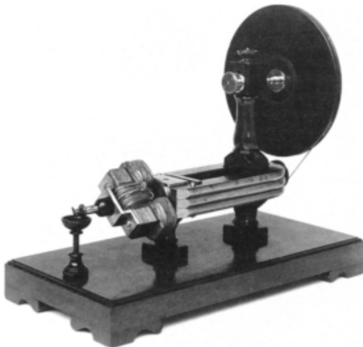
Figure 6.3: Magneto-electric generator by Saxton, 1833. Note that no wires come from this machine. It was used simply to demonstrate that rotating a coil in front of a magnet could generate electricity, which appeared as a spark when the circuit was broken as the contact strip at the end of the shaft came out of mercury in the small cup mounted on a pillar.
