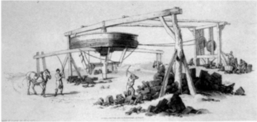
Figure 4.7: A two-horse winding engine for a colliery. This illustration from Pyne's Microcosm of 1803 is of a one-up one-down arrangement.
