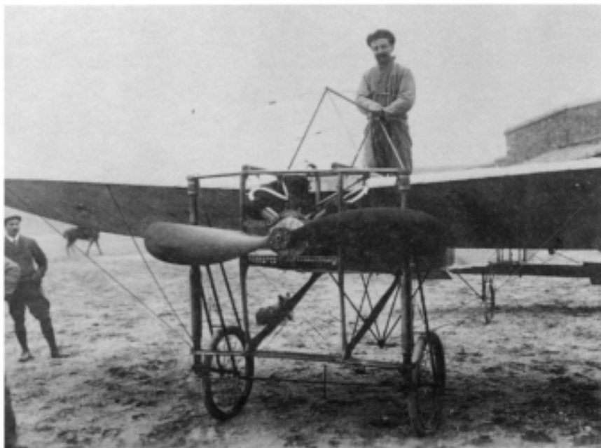
Figure 12.5: Louis Blériot standing on the seat of his Type XI aircraft, in which he flew the English Channel on 25 July 1909. The 3-cylinder Anzani engine and wooden Chauvière propeller are well shown in this picture, but the top bracing wires are less clear.
