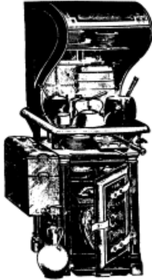
Figure 19.7: Parkinson cooker, c. 1890. Made of cast iron with silicate packing for insulation. Water heater at left side. Plate warming hood over hotplate. The Gas Council.
