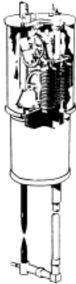
Figure 6.7: Compton arc lamp mechanism of about 1878.
