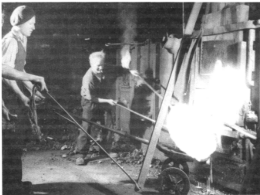
Figure 2.2: The product of the puddling furnace was a white-hot spongy mass of wrought iron. It was taken out as four or five balls and hammered (shingled) to blooms.
