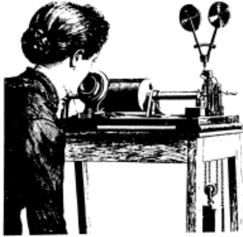
Figure 15.3: Cylinder phonograph for recording and transcribing dictation; the governor regulated the speed of the weight-driven 'motor'.
