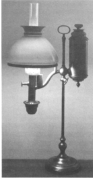
Figure 19.1: Colza oil-burning Argand reading lamp. The burner is fed by oil flowing under gravity from the reservoir above the level of the wick. The oil level in the reservoir is controlled by a float valve which closes the filling hole.
