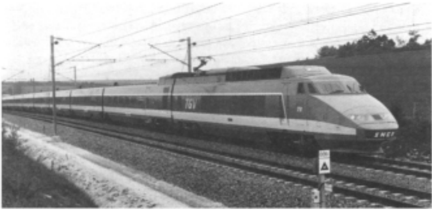
Figure 11.5: French Train à Grande Vitesse runs at speeds up to 270km/hr (168mph) on the high speed line built between 1976 and 1983 to link Paris with Lyon and south-east France. French Railways–Vignal.
