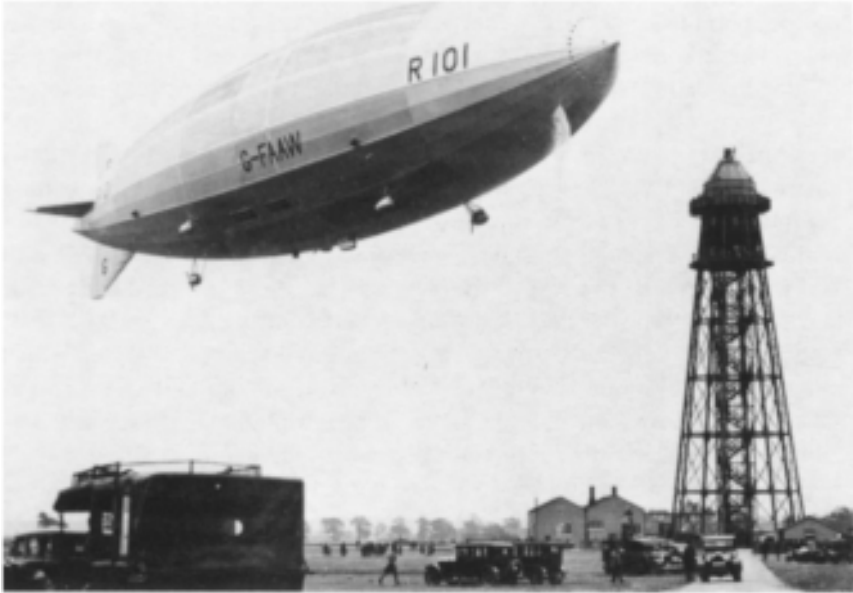
Figure 12.2: The British airship R101 leaving the passenger access tower at Cardington during test flying, October 1929. Water-ballast is being discharged near the nose, and the four ‘forward’ engines are stationary while the ship is maneuvered by the ‘reverse’ engine.
