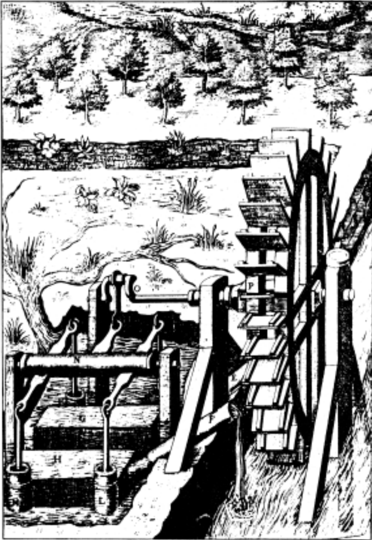
Figure 4: The crank—a key element in mechanism. From Agostino Ramelli's Diverse et Artificiose Machine , 1588.
