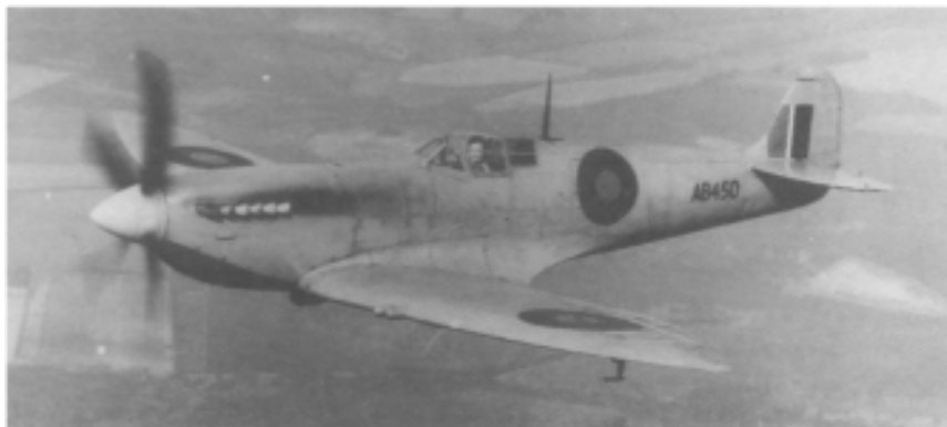
Figure 12.10: A Supermarine Spitfire VII of 1942, typical of the high-performance fighter of its time, with all-metal structure and thin cantilever wings. The engine is a 1120kW (1500hp) Rolls-Royce Merlin 61 with two-speed supercharger and the cabin was pressurized to allow operation up to 12,000m (40,000ft) altitude.
