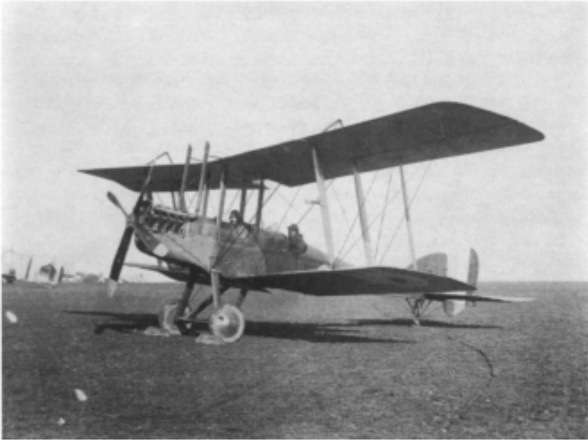
Figure 12.6: The classic biplane configuration was adopted by the Royal Aircraft Establishment to produce a stable aeroplane for military reconnaissance. This is a B.E.2E, first delivered to the Royal Flying Corps in 1916.
