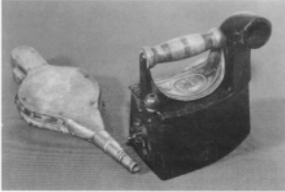
Figure 19.6: 'Cannon' charcoal iron with bellows.
