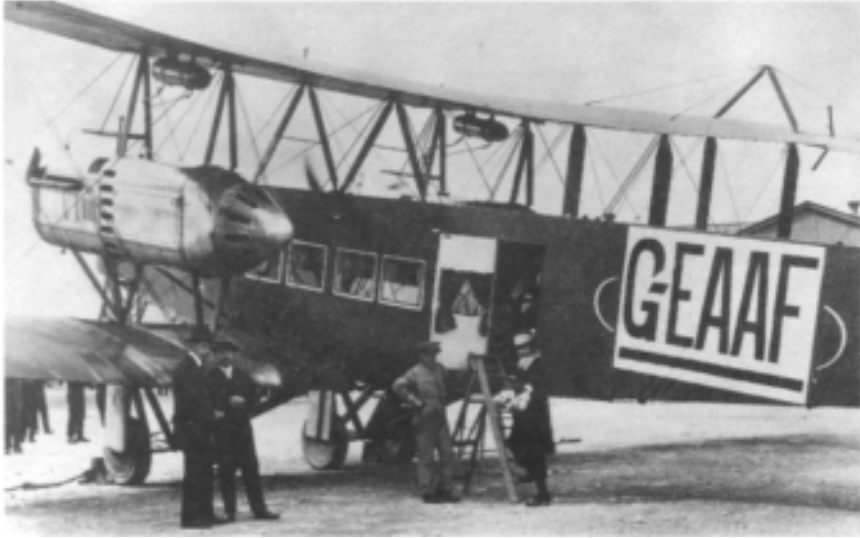
Figure 12.7: The first passenger services from London to Paris in 1919 were flown by converted bombers like this Handley Page 0/7. Ground facilities for the passengers were limited, but curtains were provided in the cabin.
