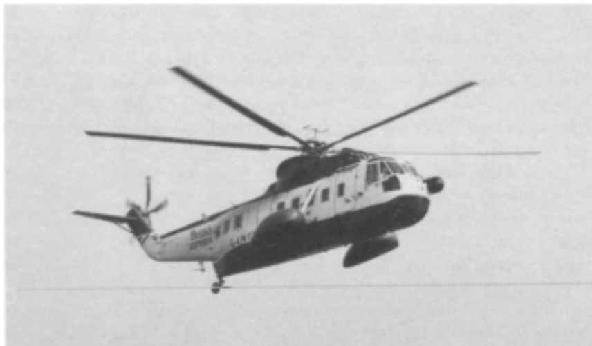
Figure 12.13: A Sikorsky S-61N helicopter carrying two dozen passengers: the classic helicopter configuration with one main rotor and a small tail rotor to balance the torque.
