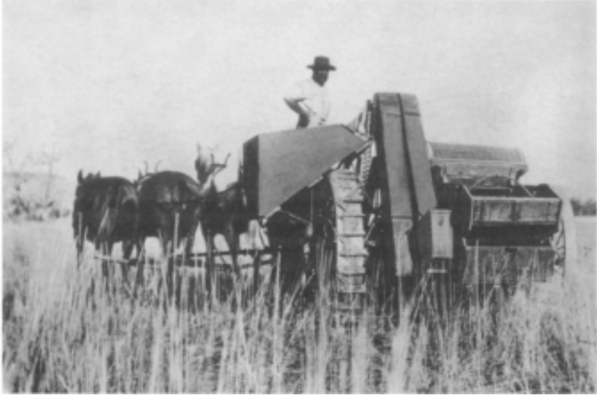
Figure 16.2: The McCormick reaper, patented in 1834. This machine employed the essential features of the modern reaper: vibrating sickle-edged blade, fingers to hold the grain and reel, divider and platform to receive it.
