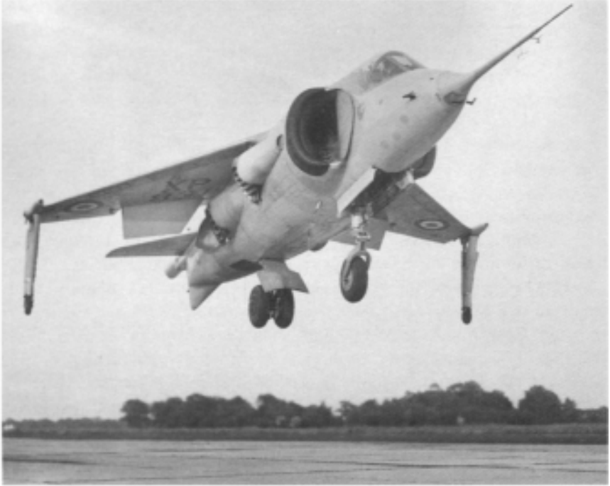
Figure 12.12: The Hawker P.1127 supported by the thrust from the four deflected jets produced by its Bristol Pegasus engine. Hawker Aircraft photograph.
