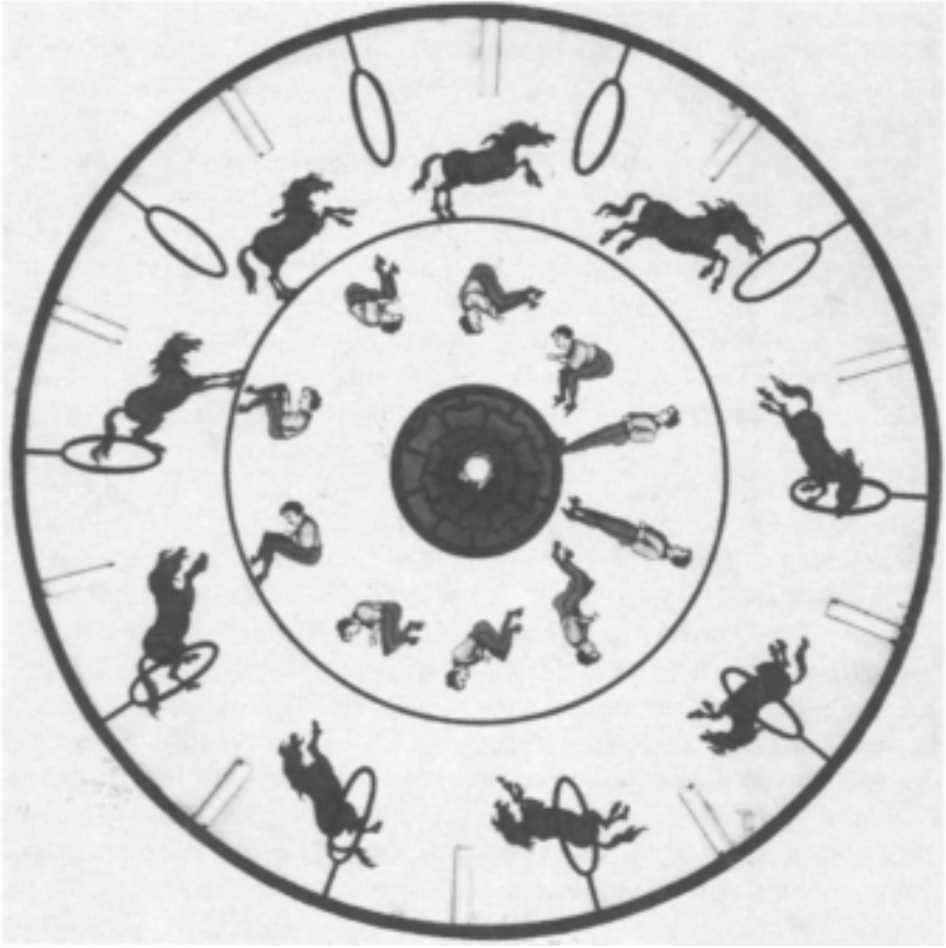
Figure 15.4: A disc for the 1833 phenakistoscope; two different, complete picture cycles are incorporated.
