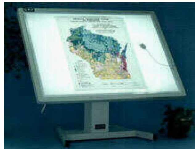
Figure 3. A digitizing board with an input device to capture data from a source map (GIS@Purdue, 2003)
