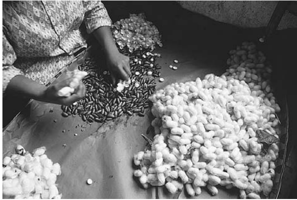
A woman in Chengdu, China, separates larvae from the silk cocoons, an early step in the process that produces silk. (TOM NEBBIA/CORBIS)
