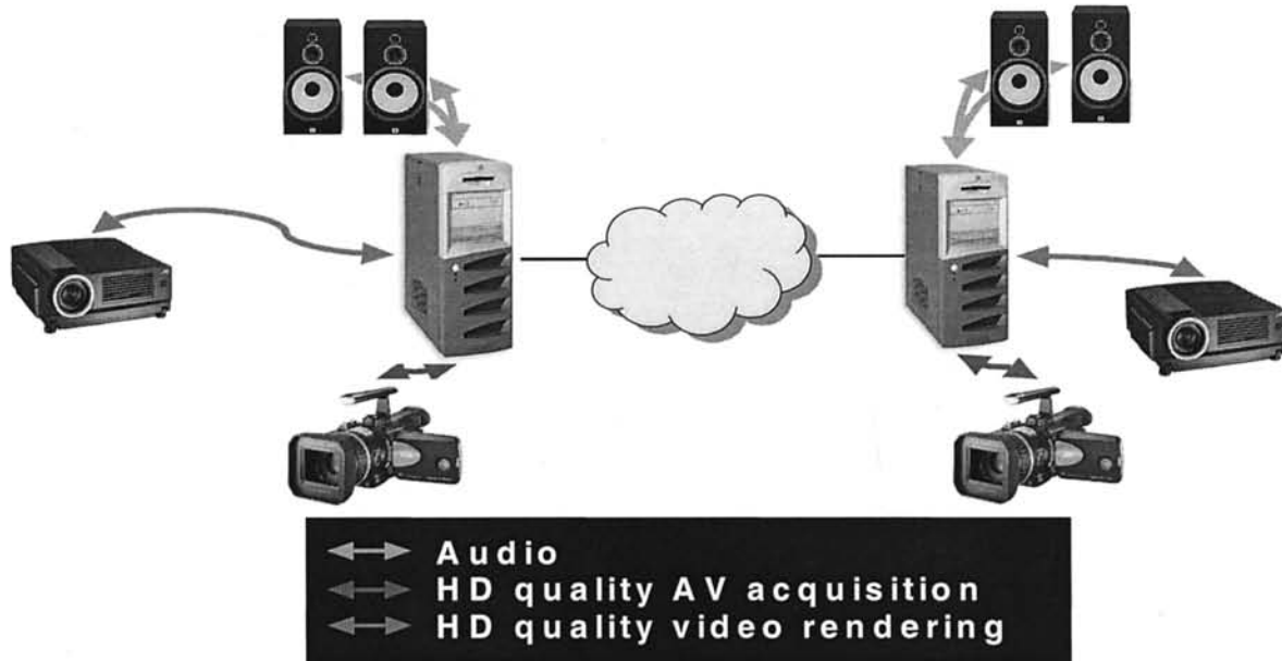
Figure 1. The HYDRA live-streaming architecture. Live HD video and audio streams captured from a camera are transmitted to the stream transmitter, which is connected to the receiver node via an IP network; the audio and video streams are then decoded and rendered.
