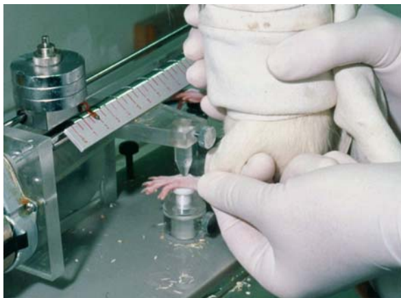
Randall-Selitto Paw Pressure Test, Figure 1 Mechanical stimulation is made using the procedure of Randall and Selitto (1957), with an Ugo Basile analgesimeter: a linearly increasing force is applied via a dome shaped plastic tip ( \varnothing = 1 mm) onto the surface of the hindpaw. The force causing paw withdrawal is quoted, as well as that inducing vocalization (audible squeak).
