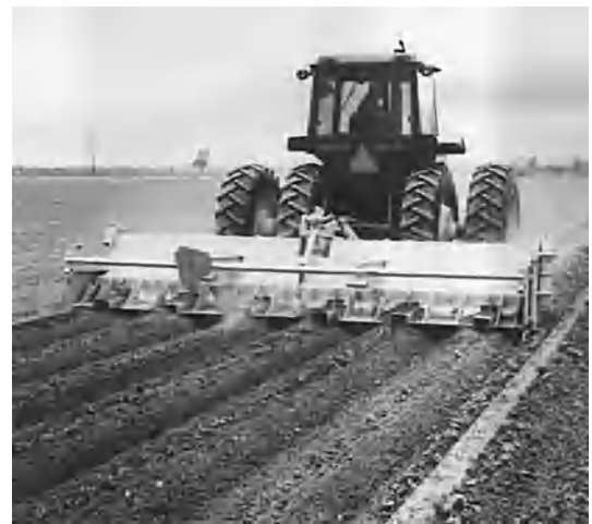
Fig. 1. Multipurpose machine used for precision tillage, planting, bed shaping, and fertilizing in one pass, and for later bed shaping, cultivating, and fertilizing. (Johnson Farm Machinery Co.)
