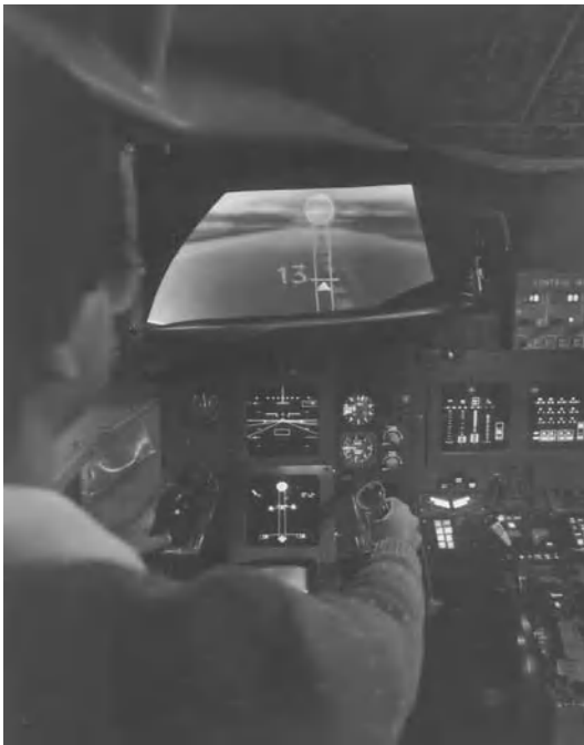
Fig. 6. Controls of transport-systems research-vehicle simulator, used to develop automated pilot aids, being operated by engineer. (NASA)
