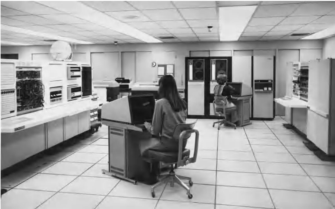
Fig. 2. Analog-hybrid laboratory equipped with a HYSHARE 600 system. This system can include up to six analog computer consoles and one or more digital processors for multiuser, multitask applications. ( Electronic Associates, Inc. )
