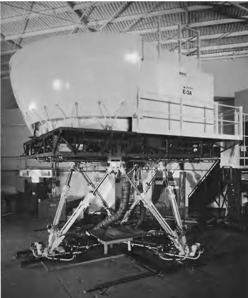
Fig. 9. Training simulator for the Boeing E-3A (AWACS) aircraft. Cabin containing flight deck, exterior of visual display system, and supporting six-degree-of-freedom motion system are shown. (Rediffusion Simulation)
