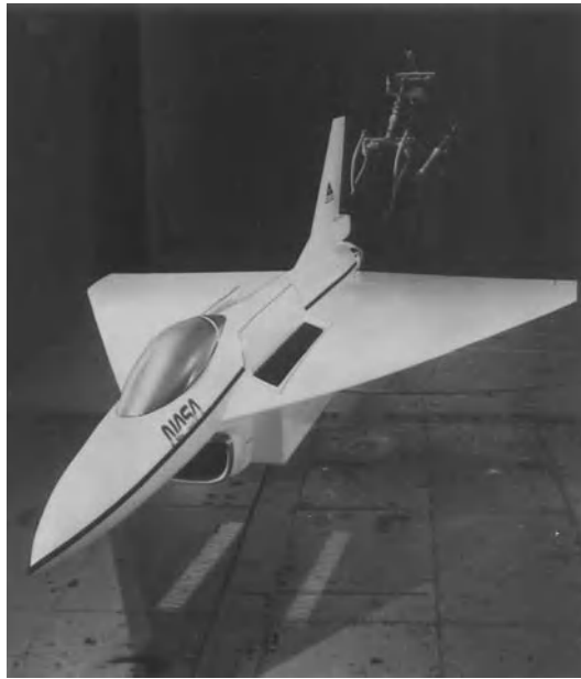
Fig. 3. Scale model of E-7 advanced fighter aircraft used for tests of experimental component called augmenter (rectangular opening in wing with open flap). (NASA)
