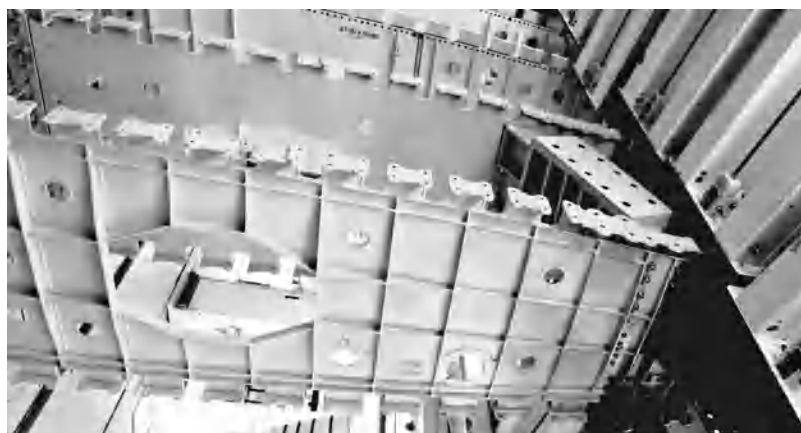
Fig. 5. Wing rib for taking engine mounting on Airbus 380 aircraft. (Courtesy of Airbus UK)
