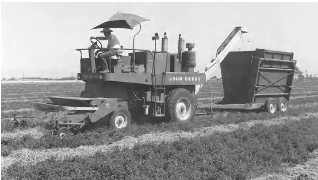
Fig. 4. Hay cuber compressing alfalfa hay into 1.6-in.-square (4-cm-square) cubes. (University of California)
