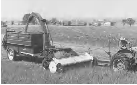
Fig. 6. Forage harvester chopping haylage for livestock feed. (Sperry New Holland, Division of Sperry Rand Corp.)
