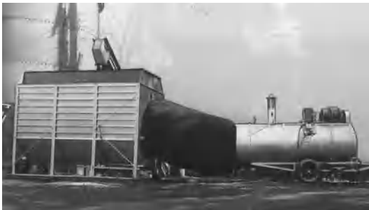
Fig. 19. Perforated metal bin for drying small grain and shelled corn with heated air from portable crop dryer.
