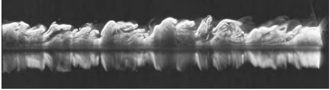
Fig. 3. Large-eddy structures (one type of coherent structure) in a turbulent boundary layer. The side view is visualized using a sheet of laser light and a fluorescent dye. (From M. Gad-el-Hak, R. F. Blackwelder, and J. J. Riley, On the interaction of compliant coatings with boundary layer flows , J. Fluid Mech. , 140:257–280, 1984)
