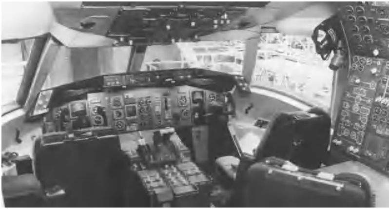
Fig. 2. Flight deck mock-up of Boeing 767 configuration for crew of three. (Boeing Co.)
