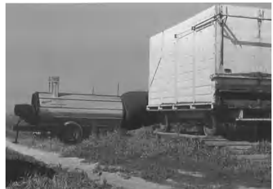
Fig. 16. Special wagon rack attached to portable oil-burning crop drier for finish-drying chopped forage.
