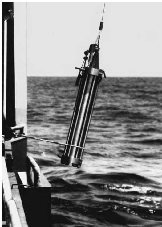
Fig. 2. Pressure- and temperature-retaining bacteriological water sampler during recovery from a depth of 6000 m (about 4 mi). Transfer into pressurized reaction vessels permits the measurement of microbial activity under field conditions. (Courtesy of S. Molyneux)
