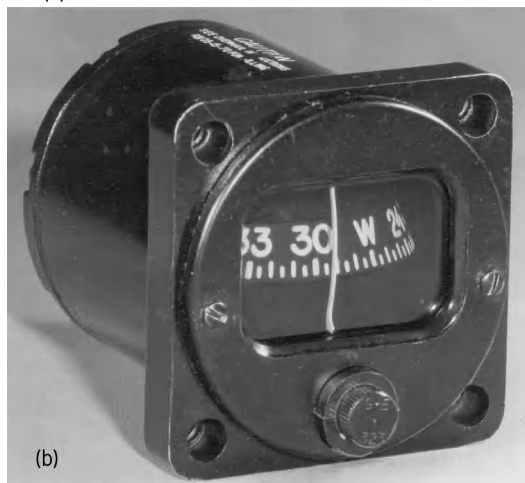
Typical magnetic compasses. (a) Marine. (b) Aircraft (Aviation Electric, Ltd.).
