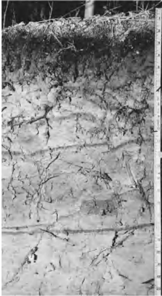
Fig. 12. Profile of an Ochrept with litter on the surface, dark A horizon 4 in. (10 cm) thick, thin B horizon, and pale C horizon; deeper profile is marked by plant roots and traces of former roots; numbers on scale indicate inches. 1 in. = 2.5 cm. (Photograph by R. W. Simonson)
