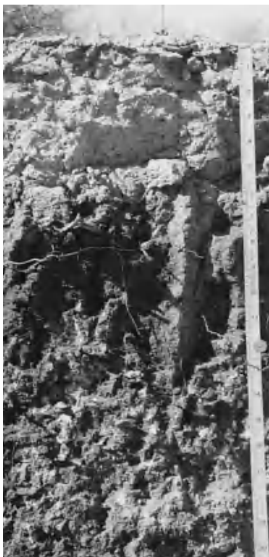
Fig. 7. Profile of an Argid with pale silty A and E horizons, darker B horizon higher in clay, and calcareous C horizon; profile shown in 20 in. (50 cm) deep; numbers on scale indicate inches. 1 in. = 2.5 cm. (Photograph by R. W. Simonson)
