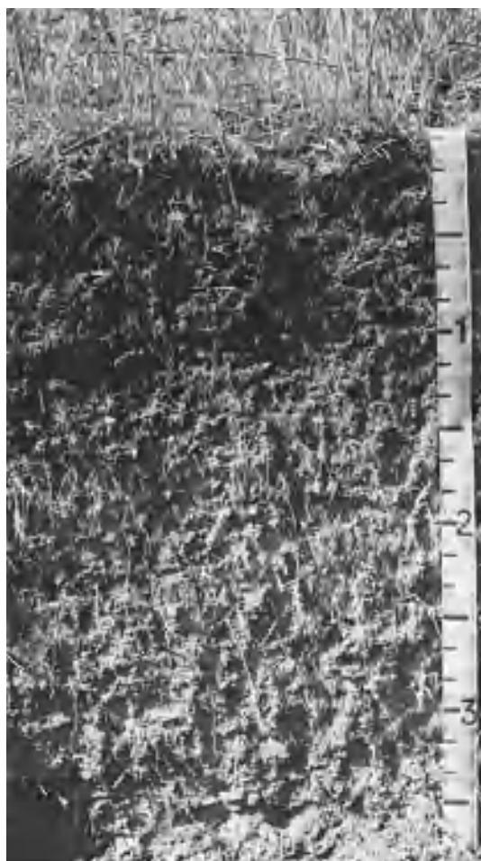
Fig. 10. Profile of an Andept with thick, dark A horizon, faint B horizon, and lighter C horizon; fine plant roots are numerous; numbers on scale indicate feet. 1 ft = 30 cm. (Photograph by R. W. Simonson)
