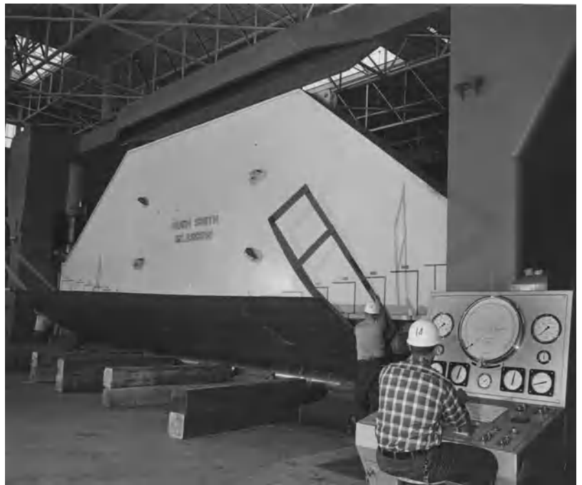
Fig. 5. Steel plate being formed in a roll press. (Newport News Shipbuilding)
