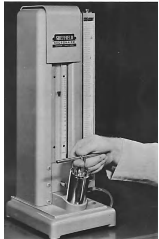
Fig. 6. The micronaire is a device for measuring wool fiber diameter, which is expressed in microns (micrometers).
