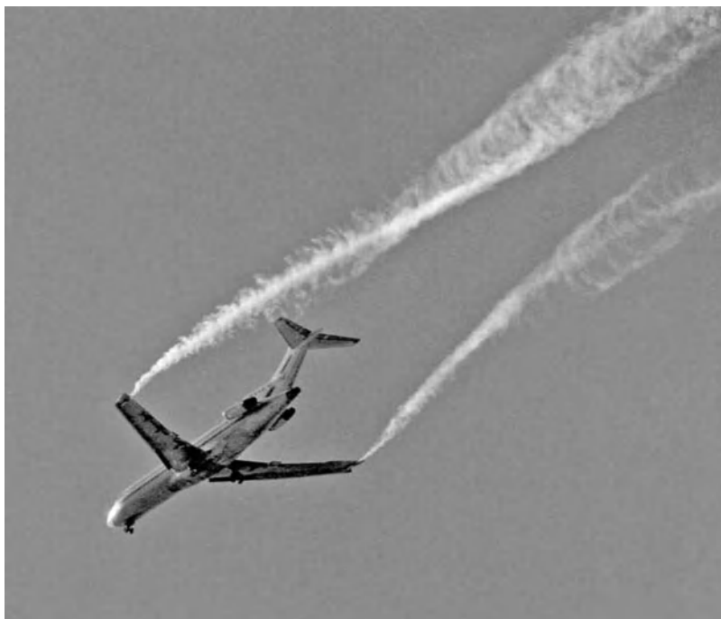
Fig. 3. Trailing vortex pair behind a Boeing 727 airplane (NASA Dryden Flight Research Center file photograph ECN 3831)
