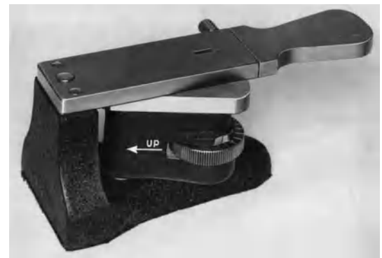
Fig. 5. Hardy sectioning device used in laboratory research for measuring wool fiber diameter.
