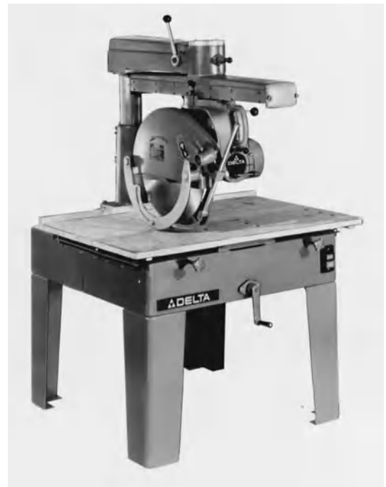
Fig. 4. Radial saw allows wood to be clamped in position while it is being cut. (Delta International Machinery Corp., Pittsburgh)
