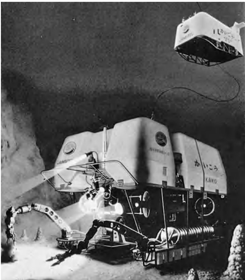
Fig. 6. Japan's 36,000-ft (11,000-m) Kaiko , a large working ROV. ( Jamstec & Mitsui Engineering and Shipbuilding )
