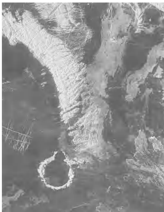
Fig. 4. Magellan image of a portion of Leda Planitia. The smooth (radar-dark) plains were formed by volcanic lava flows that covered the region. These flows embayed the older, radar-bright, highly fractured or chaotic highlands, sometimes called tessera, that rise out of the plains in the upper-left or northwest part of the image, as well as the circular ring structure in the lower left, which is probably an impact crater. Subsequent volcanism produced radar-bright flows in the upper right. (Jet Propulsion Laboratory; NASA)
