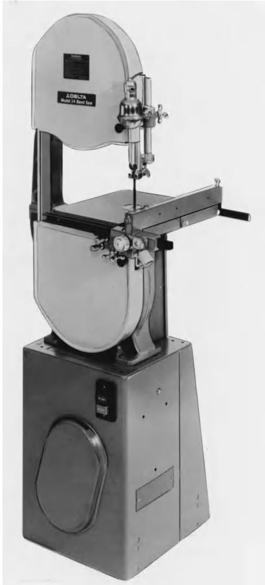
Fig. 2. Narrow bandsaw, a flexible band of steel, can make curved as well as straight cuts even in thick pieces. (Delta International Machinery Corp., Pittsburgh)
