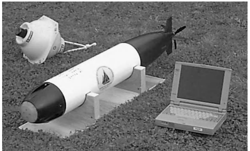
Fig. 10. REMUS is rated for continental shelf depths (355 ft; 200 m) and is compact and lightweight (40 kg; 88 lb). It is depicted with its laptop computer for downloading missions and uploading data, and one of the acoustic transponders used for navigation. (Woods Hole Oceanographic Institution)
