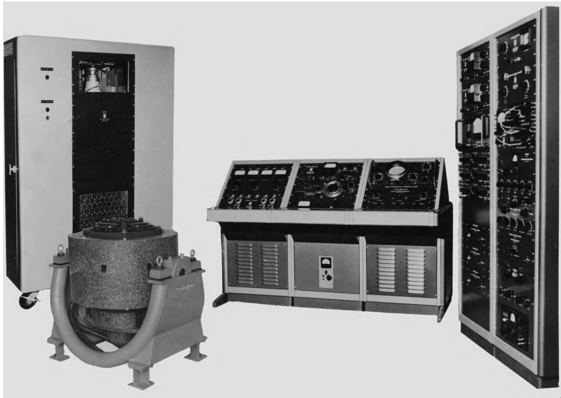
Fig. 3. Complete vibration test system showing the electrodynamic shaker in the left foreground. In the rear, from left to right, are the power amplifier, control console, and instrumentation cabinets. (Calidyne Co.)
