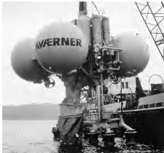
Fig. 9. Structurally reliant vehicle used for servicing seafloor oil well structures. (Kvaener Brug A/S)
