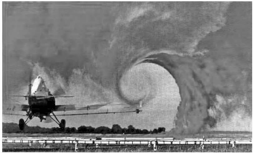
Flow visualization of aircraft wing-tip vortices. (NASA)
