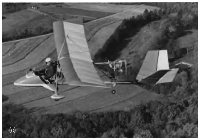
Ultralight aircraft. (a) Pterodactyl Ascender, a canard-type aircraft with 35-hp (26-kW) engine ( Freedom Fliers, Inc. ). (b) FP-303, with all-wood, latticed construction ( Fisher Flying Products ). (c) "Hummer" aircraft, with three-axis controls and V-tail ( Maxair ). (d) Quicksilver GT, which uses three-axis controls and 28-hp (21-kW) engine ( Eipper Aircraft ).
