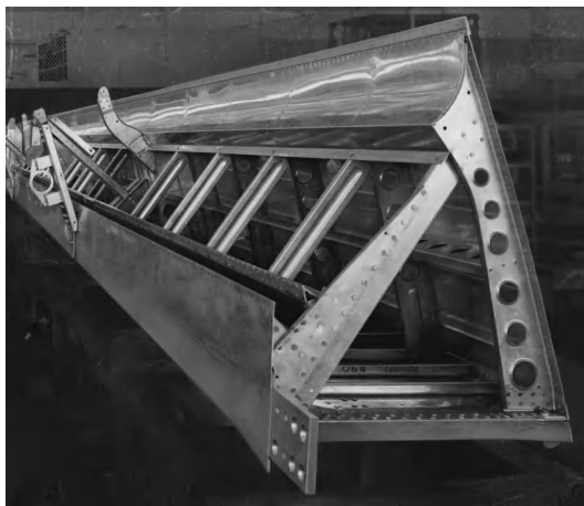
Fig. 20. Trailing edge with hinges for movable surfaces.
