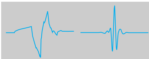
Fig. 2. Two examples of wavelets which generate an orthonormal basis, and which are associated with fast algorithms.
