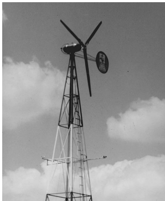
Fig. 1. A small dc horizontal-axis wind machine for rural use.
