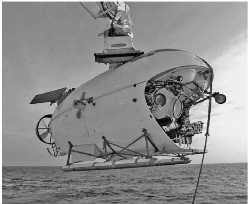
Fig. 12. One of the two Russian Mir 20,000-ft (6,000-m) manned submersibles. (P.P. Shirshov Institute of Oceanology)
