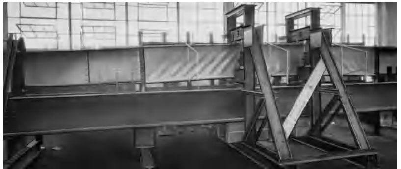
Fig. 12. Partial tension field beam under test.
