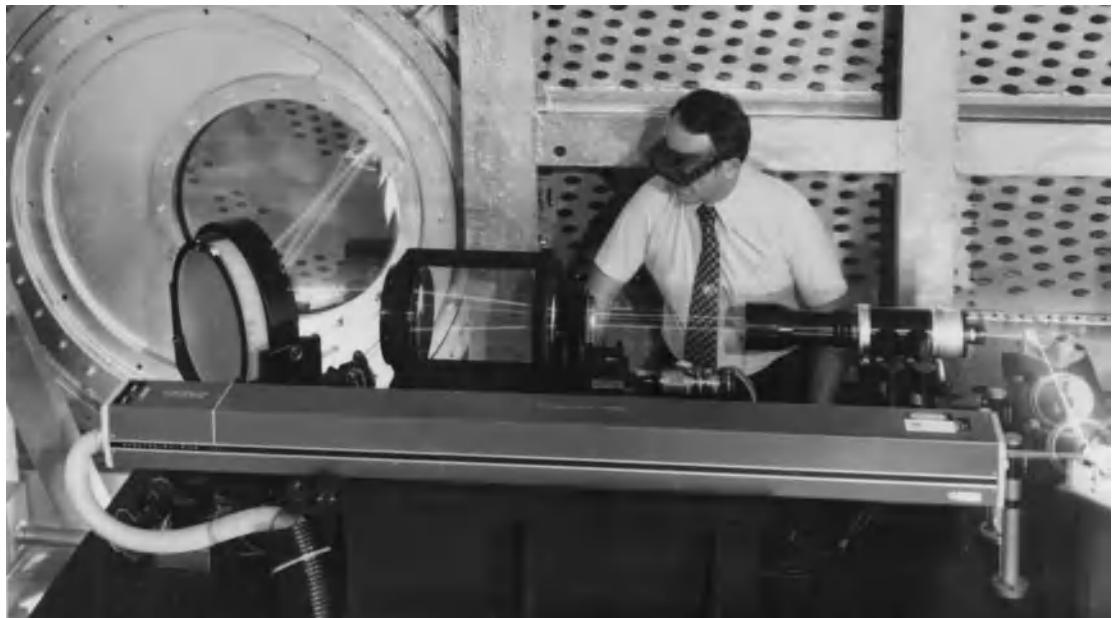
Fig. 17. Laser velocimeter used for turboprop flowfield analysis in wind tunnel at NASA Lewis Research Center.
