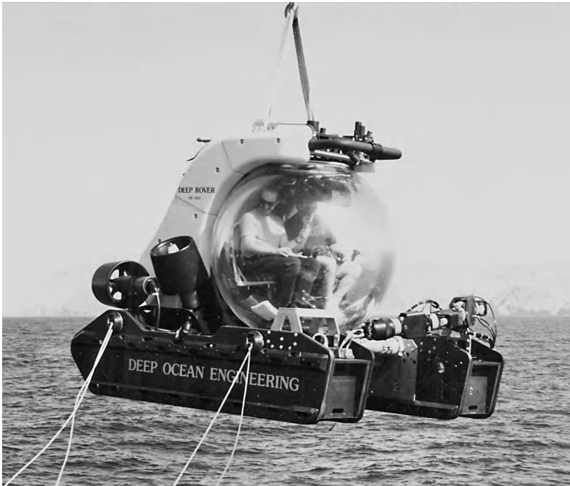
Fig. 1. Two-person deep submersible vehicle Deep Rover with all-acrylic pressure hull. (Deep Ocean Engineering, Inc.)
