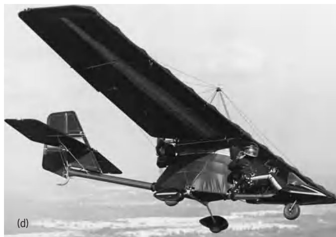
Ultralight aircraft. (a) Pterodactyl Ascender, a canard-type aircraft with 35-hp (26-kW) engine ( Freedom Fliers, Inc. ). (b) FP-303, with all-wood, latticed construction ( Fisher Flying Products ). (c) "Hummer" aircraft, with three-axis controls and V-tail ( Maxair ). (d) Quicksilver GT, which uses three-axis controls and 28-hp (21-kW) engine ( Eipper Aircraft ).
