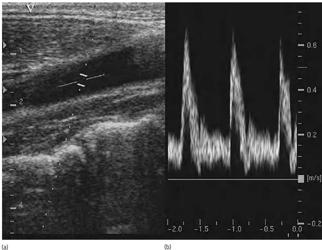
Fig. 10. Duplex display from a diagnostic ultrasound scanner. (a) B-mode image of the human carotid artery. The depth in centimeters is shown along the left side. The three triangles at left mark the position of the electronic focal zones for transmit. The graphic in the center of the image indicates the location where the Doppler measurement is being made. (b) Spectral Doppler display. The abscissa (horizontal axis) is time in seconds, and the ordinate (vertical axis) is flow velocity from the angle-corrected Doppler measurement. The gray scale in the display is the relative power in the Doppler signal for the velocity and time specified by the location on the display.
