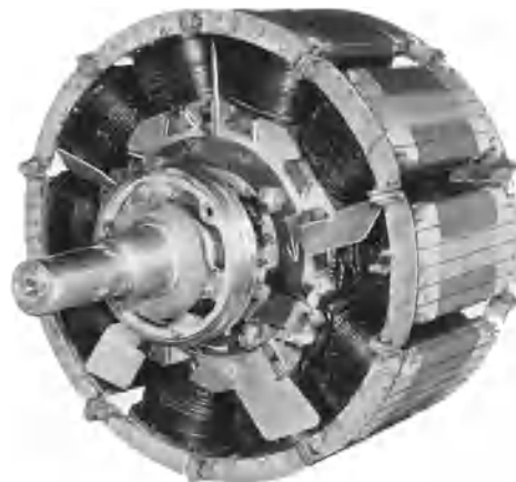
Fig. 1. Salient-pole field winding on rotor of synchronous motor. (Allis-Chalmers)
