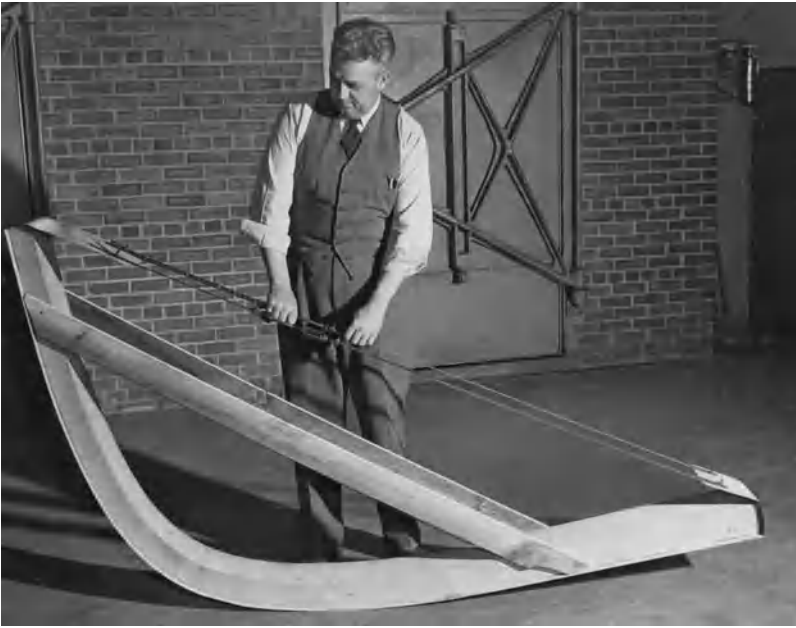
Fig. 6. Bent boat rib is prepared for drying with end pressure applied by the strap and the rods placed against the convex side of the piece. Wood stays assist in holding the work in position. (Forest Products Laboratory, Madison, Wisconsin)
