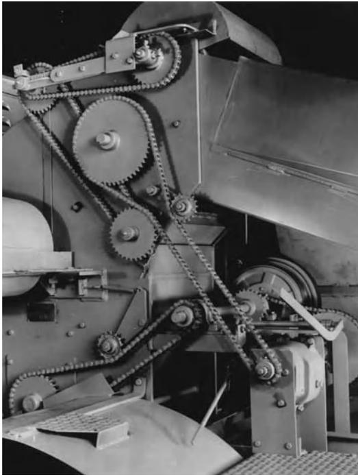
Fig. 2. Roller chain drive. (FMC Corp.)
