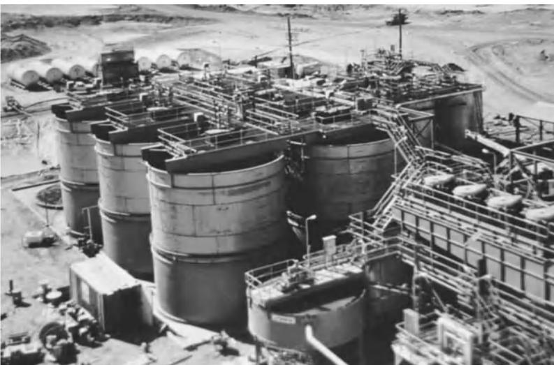
Industrial-scale, aerated, continuously stirred tank plant for bioleaching sulfidic-refractory gold concentrate. The large tanks are the bioleach circuit for pretreating the mineral concentrate and in front of them is the circuit for extracting the gold from the bioleached solids. (Photo courtesy of BacTech Mining Corp.)
