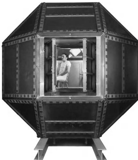
Fig. 2. Magnetic field of the brain being measured in a magnetically shielded room. The SQUID detector is in the tail of a Dewar cylinder containing liquid helium, which maintains the cryogenic temperature of the SQUID.
