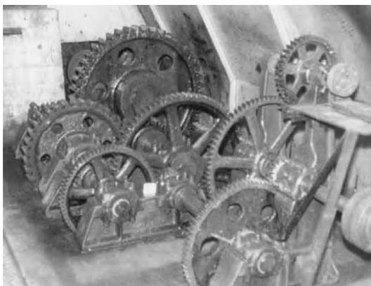
Fig. 8. Exposed gear reductions on an early bascule bridge.
