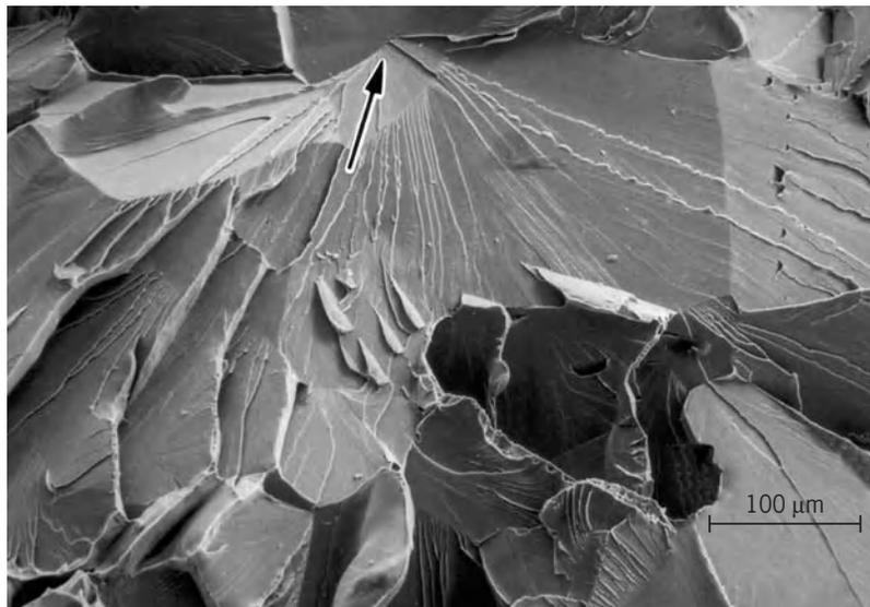
**Fig. 2.** Scanning electron microscope image of a transgranular cleavage fracture surface in a steel tested at a temperature below its brittle-to-ductile transition. The arrow indicates the likely fracture initiation site.
