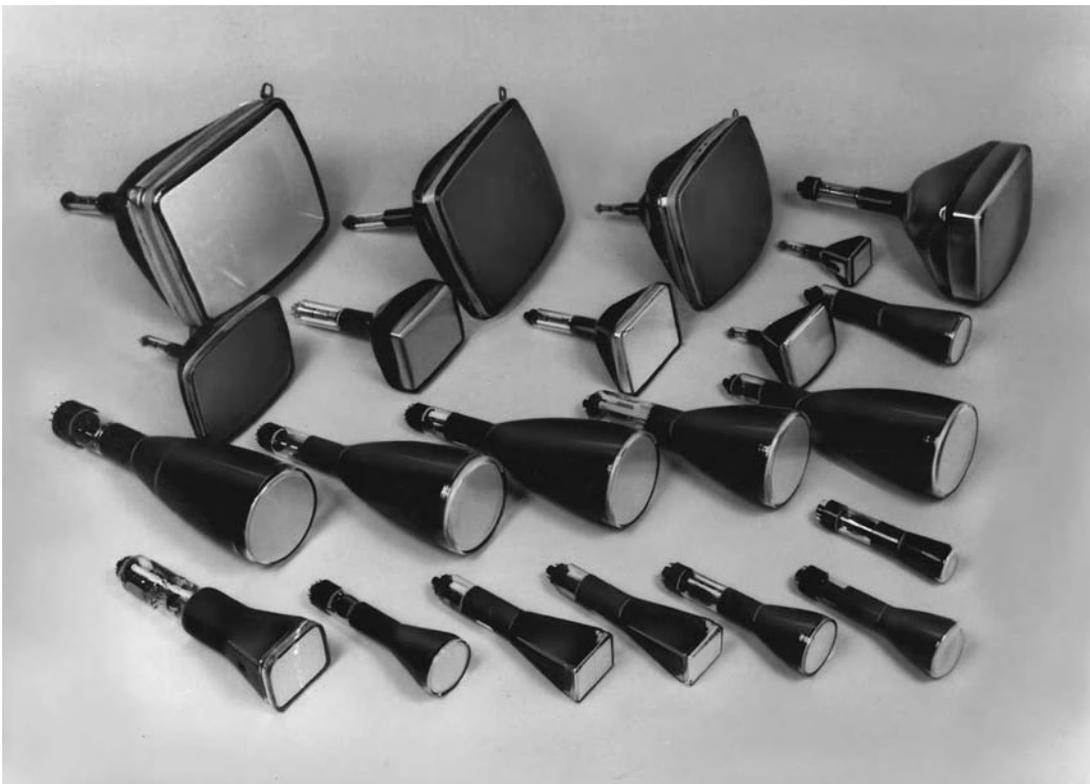
Fig. 2. Typical cathode-ray tubes.
