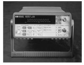
Fig. 3. General-purpose frequency counter. (Hewlett-Packard Co.)
