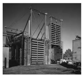
Fig. 15. Vacuum cooler of railroad-car size. (Gay Engineering Corp.)
