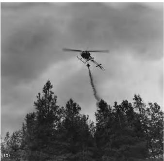
Fig. 7. Aerial fire suppression. (a) Mixing and loading fire retardants in preparation for an air drop. (b) A helicopter with a detachable 40-gal (151-liter) tank drops borate slurry on a pinpoint target. (U.S. Forest Service)
