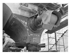
Fig. 4. Large waterjet propulsors used in high-speed catamaran ferry. (*Hitachi Zosen*)
