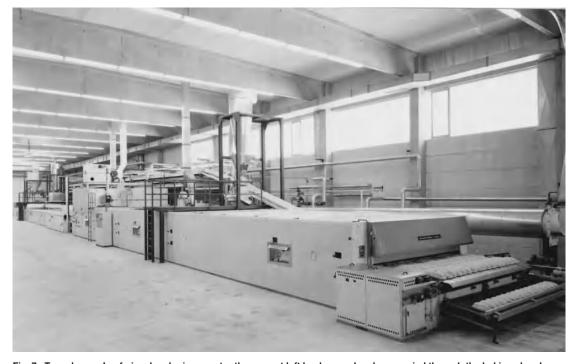
Fig. 7. Tunnel oven. Loaf-size dough pieces enter the oven at left background and are carried through the baking chamber on a continuous metal belt which serves as the hearth. The baked loaves exit at right foreground. Ordinary pan bread would require sets of pans conveyed by a slightly different mechanism, but the basic oven structure would be the same. (Adam Equipment Co.)
