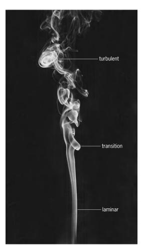
Fig. 5. Laminar and turbulent flow in a smoke plume. (From S. Whitaker, Introduction to Fluid Mechanics, Krieger Publishing, 1981)
