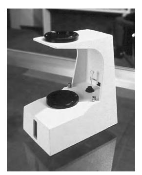
Fig. 2. Polariscope to distinguish between single and double refraction. (Gemological Institute of America)
