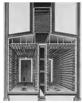
Fig. 1. Double radiant box furnace. (Lummus Co.)
