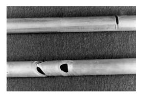
Fig. 2. Heat exchanger tubes cut through at supports and damaged by impacting from broken tubes due to flow-induced vibration.
