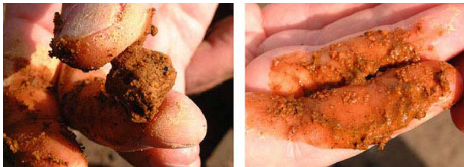
Figure A24 Thixotropy. Undisturbed clod is shown on to the left, but disturbed clod to the right. The soil reaches the liquid limit when disturbed with gentle pressure, even though the clod appears relatively dry. The soil is hydric andosol from the Azores (Portugal).
