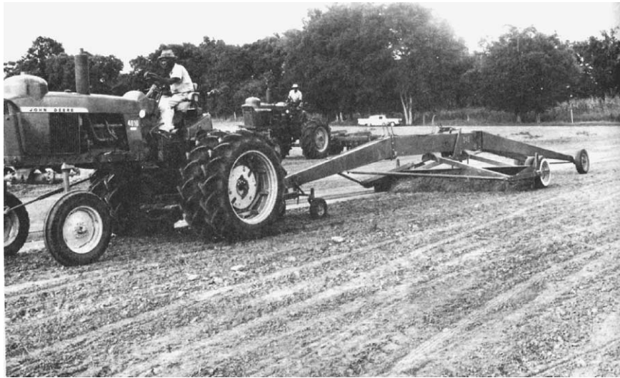
Figure 2 Landplane used for smoothing the soil between surface drains. Reprinted from Pavelis GA (ed.) (1987) Farm Drainage in the United States: History, Status, and Prospects . Miscellaneous Publication No. 1455. Economic Research Service. US Department of Agriculture. Washington, DC: US Government Printing Office.
