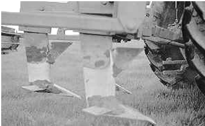
Figure 5 A three-shanked subsoiler. (Photo by K C Cameron, Lincoln University, Canterbury, New Zealand.)
