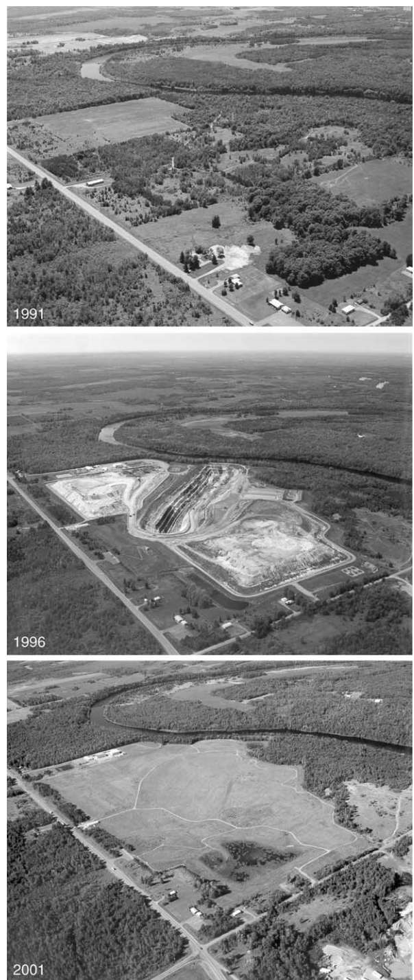
Figure 7 The Kennecott Flambeau Mine near Ladysmith, Wisconsin, was mined for copper, gold, and silver in the 1990s. At the end of mining, the open pit was completely backfilled and native vegetative communities were established. The site now includes high quality wetlands, native prairie, woodlands, and nature trails. Photographs before mining (1991), during mining (1996), and after restoration (2001) by T-B0 and courtesy of the Kennecott Flambeau Mining Company.
