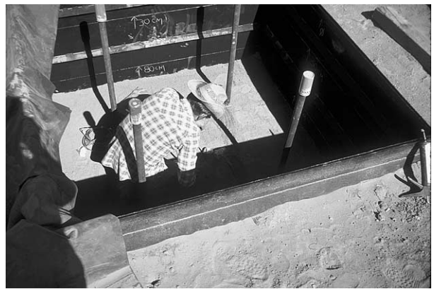
Figure 3 Technician installing soil-water sensors in a repacked lysimeter near Five Points, California. The lysimeter is a 2-m square ( 4\text{ m}^2 ). (Photo courtesy of USDA-ARS, Water Management Research Laboratory, Parlier, California, USA.)
