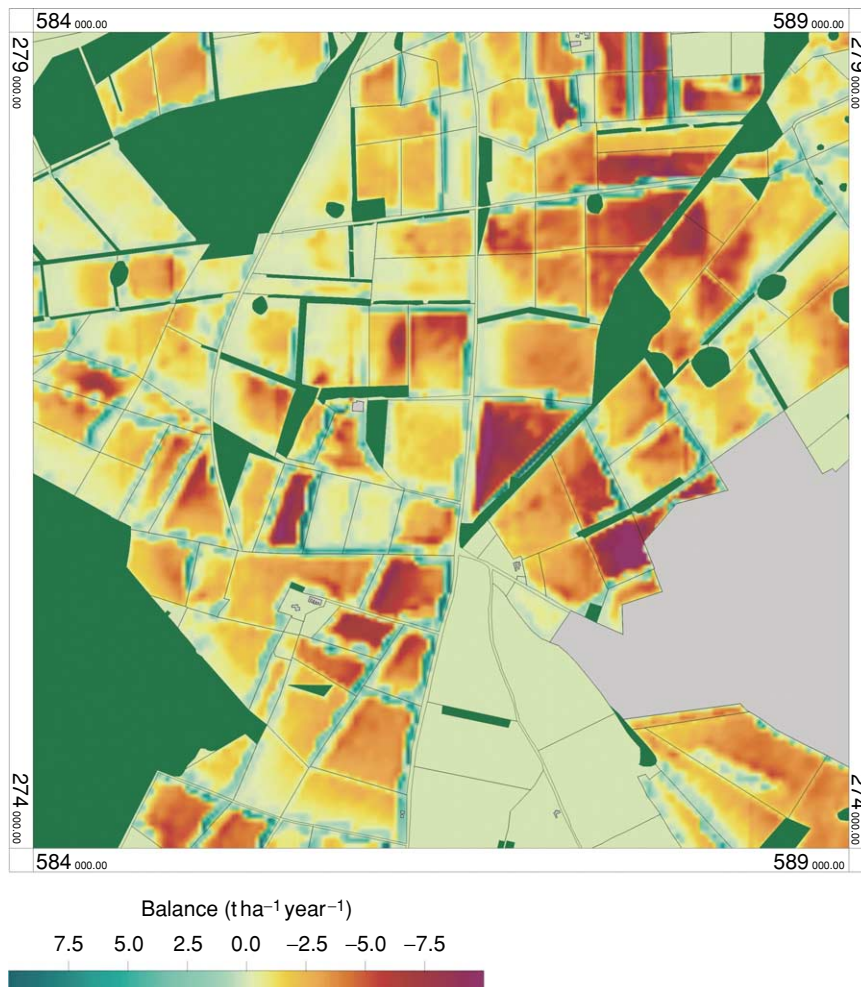
Figure 5 Modeled spatial distribution of the mean annual erosion–accumulation balance at the Barnham test site, UK (1970–98). Due to changing wind directions and annually varying vegetation cover, the orientation of the soil erosion rate gradient may differ among the individual fields (dark green, forests; gray, settlements and Honington airport). Model domain covers 5 × 5 km. Reproduced from Bohner et al. (2003) The Weels model: methods, results and limitations . Catena 52: 289–308, with permission from Elsevier.
