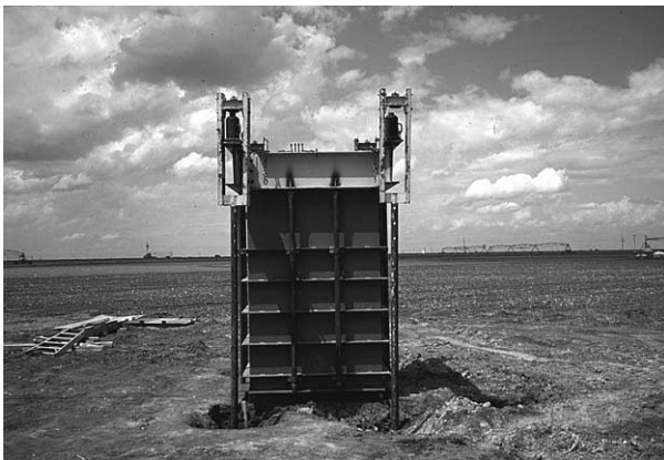
Figure 4 A monolith soil tank (1.5 m square and 2.3 m in depth) ready for insertion at Bushland, Texas. The hydraulic rams are located on the top corners and offset to permit a backhoe to excavate along the outside of the tank as it is pressed into the soil against the anchors secured into concrete piers. (Photo courtesy of USDA-ARS, Conservation and Production Research Laboratory, Bushland, Texas.)
