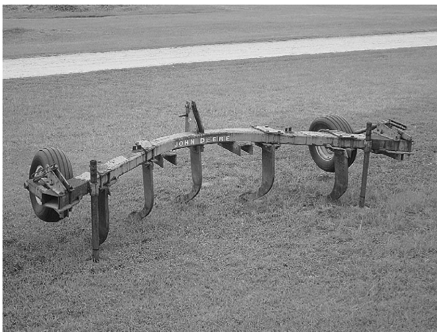
Figure 5 V-frame subsoiler used for complete disruption of soil compaction.
