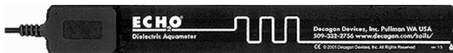
Figure 1 An example of a capacitance soil-water content sensor. The circuitry to measure the capacitance is in the overmolded head of the probe. The capacitance sensor is in the blade and consists of parallel conductors sandwiched between insulating layers.
