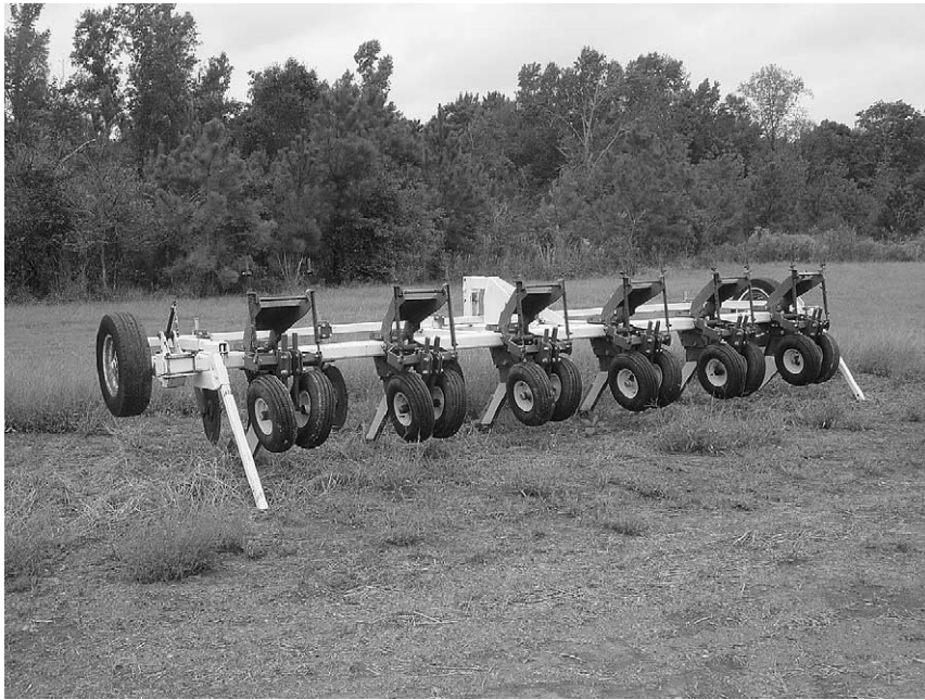
Figure 6 Strip-tillage subsoiler used for subsoiling beneath rows. Note closing wheels, which prepare the seedbed for planting.
