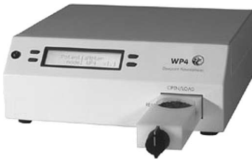
Figure 4 Dew-point potentiometer for measuring water potential of soil samples using vapor equilibration. The sample is placed in the cup, sealed inside the instrument, and the dew point and sample temperature are measured.
