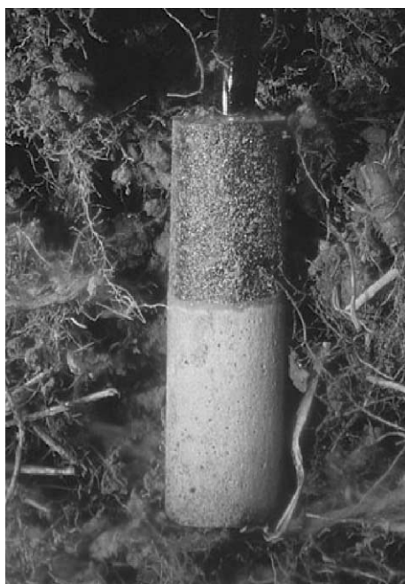
Figure 3 Heat-dissipation matric-potential sensor. The darker, upper part of the cylinder is the overmold, containing wires and connections. The lighter, lower part is the ceramic matrix, which equilibrates with the soil.
