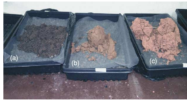
Figure 17 Fragmentation state of large clods after six wetting-drying cycles; (a) clayey vertisols; (b) clayey oxisols; and (c) clayey ultisols.
