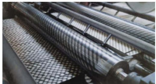
Fig. 3: Typical vigoureux patterning on combed tops (Fleissner).
