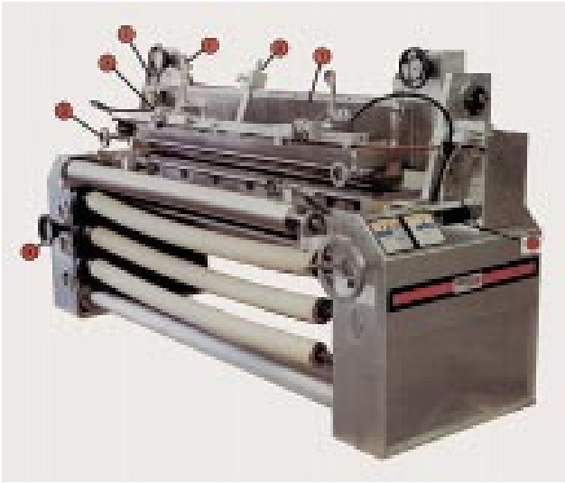
Fig.: Coating machine (Mascoe) with the following elements: 1 = individual side adjustment of the coating blade; 2 = vertical height adjustment of the blade; 3 = horizontal adjustment of the blade; 4 = coating table adjustment; 5 = oscillating compound supply system; 6 = display showing horizontal blade settings; 7 = blade holder; 8 = flexible cable.
