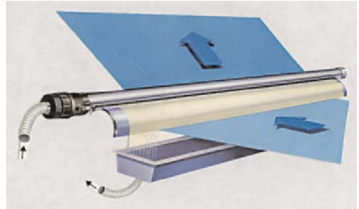
Fig. 3: Liquor pouring as a method of product application (curved blade/West Point).
