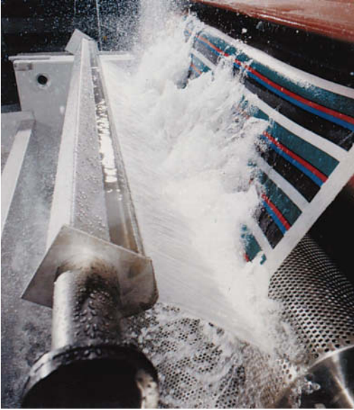
Fig. 1: An Arioli spray system in the first washing bath of an after-print washing of printed goods.
