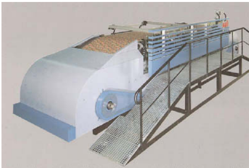
Fig. 1: A short-run rotary printing machine using an endless steel band (Gali).
