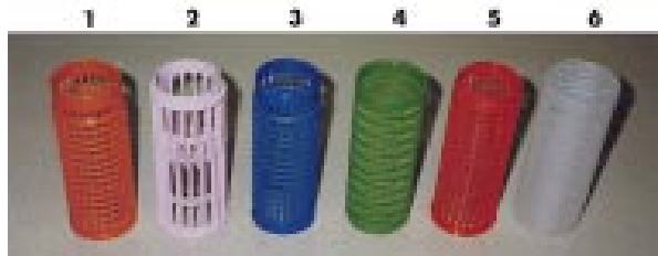
Fig.: Axial-flexible cores from different manufacturers. 1 = Karo core: disposable pressure dyeing core; diam. 54/60 mm, 170 mm (Karo Kunststoffwerke); 2 = Combi-Flex: ribbed core; diam. 54/60 mm, 170 mm (J. Zimmermann-Eisbär Nadelfabrik); 3 = Becker core: disposable pressure dyeing core; diam. 54/60 mm, 170 mm (Karo Kunststoffwerke); 4 = Zet-Flex core: coarse screen core; diam. 54/59 mm, 170 mm (H. N. Zapf KG); 5 = AC dyeing core: coarse screen core; 54/59 mm, 170 mm (J. Zimmermann-Eisbär Nadelfabrik); 6 = "Engel" dyeing core: diam. 58 mm, 170 mm (Engel Multiflex System GmbH).
