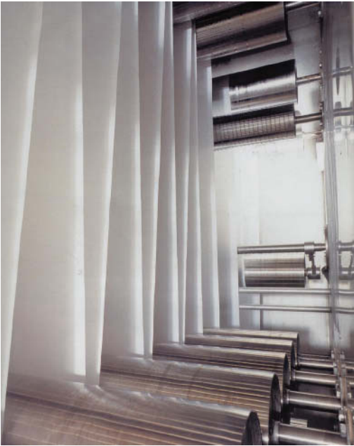
Fig. 7: Fabric guide rollers in the Brugman steamer.
