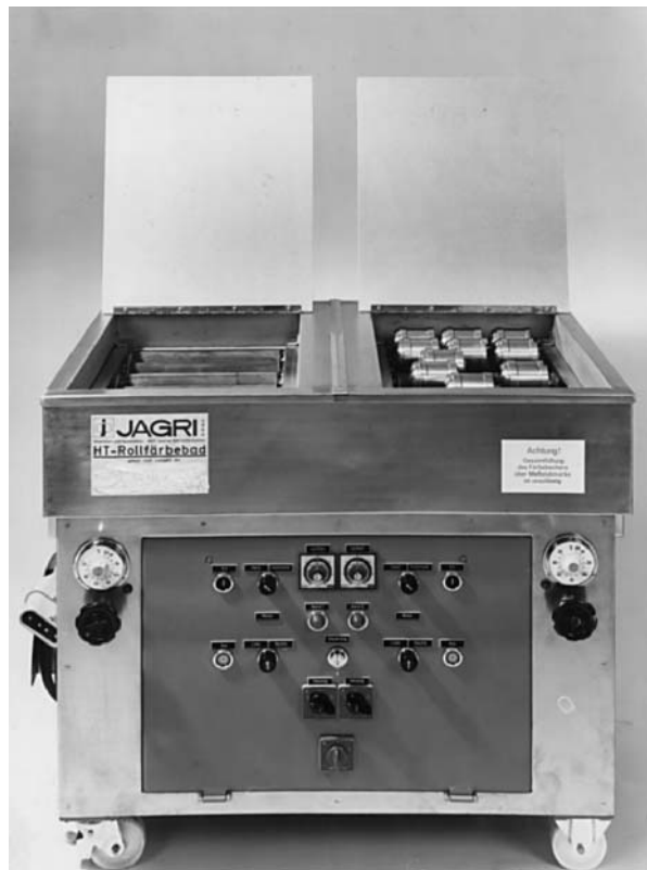
Fig. 1: Roller dye bath by Jagri.
