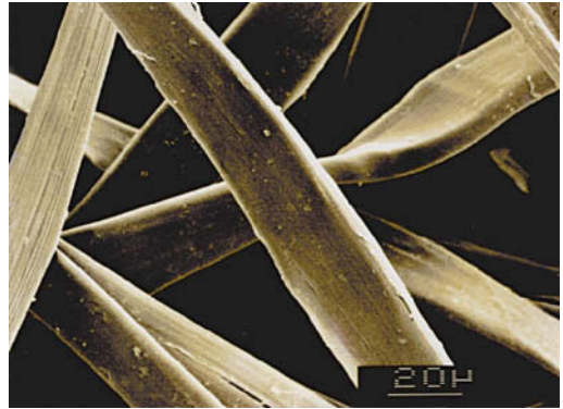
Fig. 3: Scanning electron microscope image of tussah silk.
