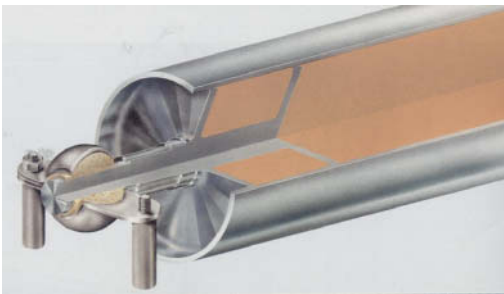
Fig. 2: Internal bearing method complete with special bearing.
