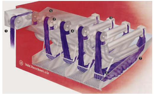
Fig. 3: Henriksen shrink: a shrinkage drier for tubular knitted goods, which are transported into air jet shafts by drive rollers (2) and thrown against baffle plates (3) by hot air before residing for a period of time in the basket (7) during each cycle of the continuous process.
