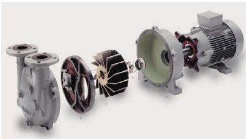
Fig. 2: Exploded view of a vacuum pump (Siemens Elmo F) a) side casing; b) cam plate; c) impeller; d) floating ring seal; e) pump housing; f) motor.
