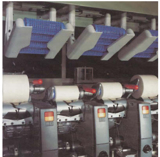
Fig. 1: Axially pressable dyeing tubes on the Autoconer 238 (Schlafhorst) ready for yarn winding.
