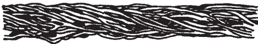
Fig. 3: A longitudinal view of the Rosenbaum model. A bundle of chain molecules in the non-crystalline region of a fibre lies above the glass transition temperature and has a fraction of free volume. Dye molecules enter the free volume through a series of location-changing leaps.
