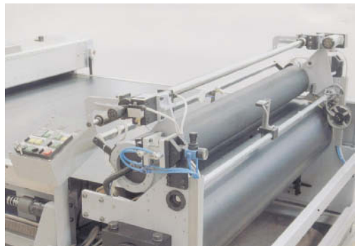
Fig. 4: Feeder and glueing device for fabrics to be printed (Viero).
