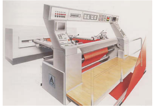
Fig. 6: A stenter control bridge with the Babcock "Dasy-Tex" process control system. The "Dasy-Tex" hardware includes local autonomous control loops, a higher-order computer, the program memory, the operator's keyboard, a monitor and a page printer.
