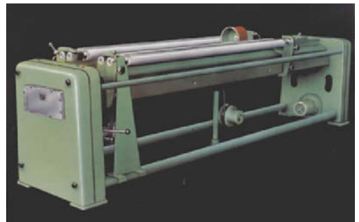
Fig. 15: A card grinding machine AH 5 (grinding stand) by Franz Müller.
