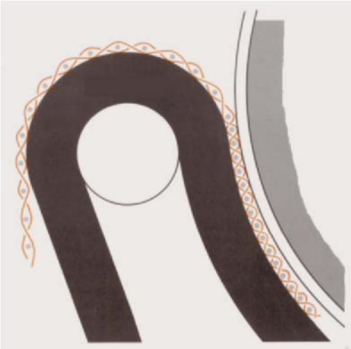
Fig. 5: Controlled shrink between a hot cylinder (right) and thick rubber belt (black) (by Morrison).
