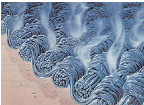
Fig. 7: Perspiration molecules quickly evaporate through the fabric pores which are thousands of times larger; the body temperature remains stable and the fabric stays dry inside (source: Hoechst).
