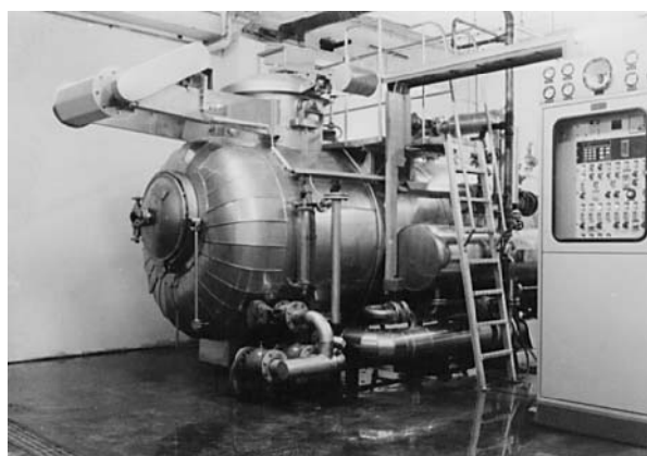
Fig. 2: Liloc-Overflow dyeing machine by Jagri.
