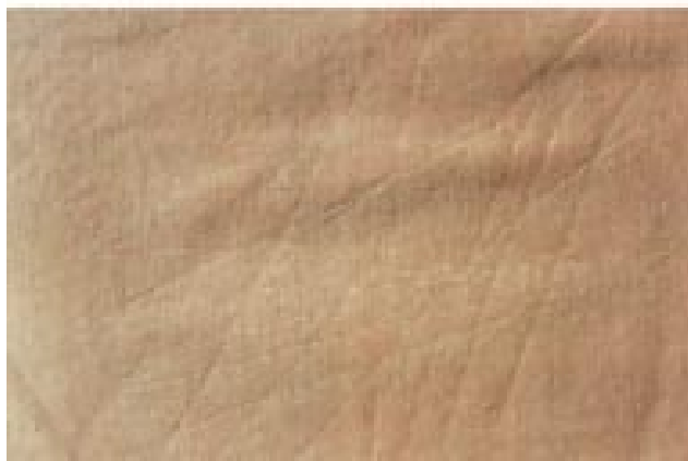
Fig.: Surface-sensitive, relatively hard, plasticizable knitted fabric. Threads and meshes are permanently displaced by mechanical influences, causing a change to the reflection of light. Flattened areas shine, the surrounding surface gives a diffuse reflection (top = right side; bottom = reverse side) (source: Steinbrecher).
