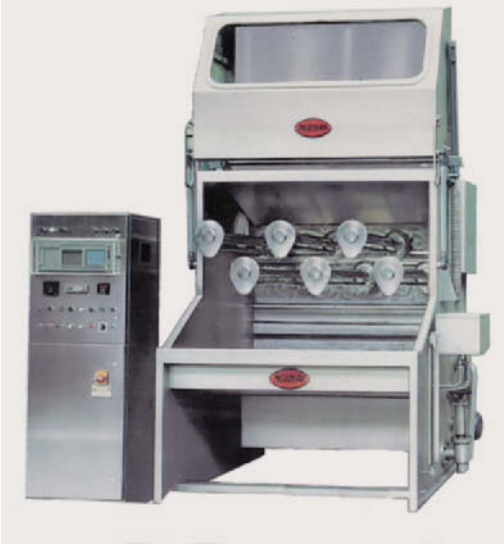
Fig. 4: Mezzera spray dyeing machine for six yarn hank rows.
