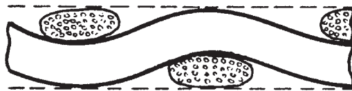
Fig 2: Thread porosity: the threads are porous, while their fibres are solid.
