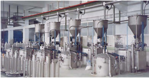
Fig. 1: Crosswound yarn package dyehouse (Thies) with material transport by means of roller conveyer and crane way plus metering and automation units on each dyeing machine.
