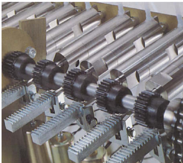
Fig. 2: Rack-and-pinion drive in a dispenser (Ishizaka).
