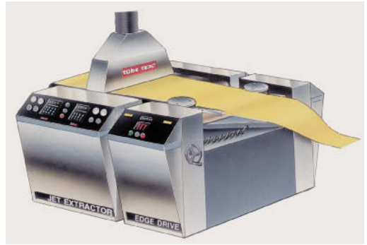
Fig. 2: Tube-Tex-Jet-Extractor (vacuum extraction) for knitgoods.
