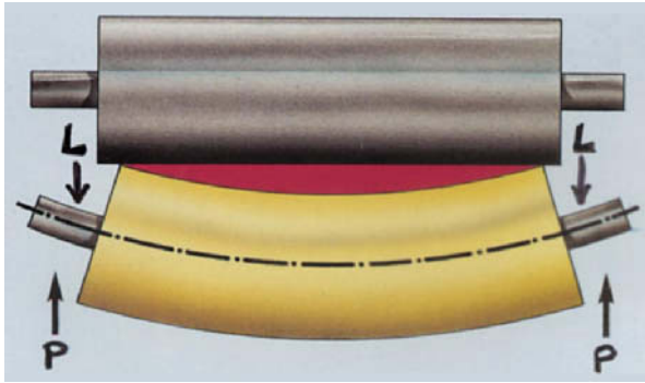
Fig. 3: Padder roller flexure. L = bearing counterpressure; P = pressure.
