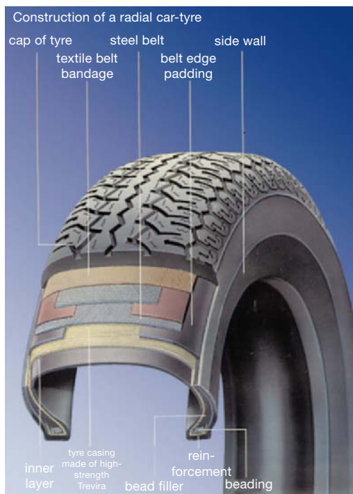
Fig.: Construction of a car tyre from tyre cord layers, made composite through vulcanization of layered rubber (Hoechst).
