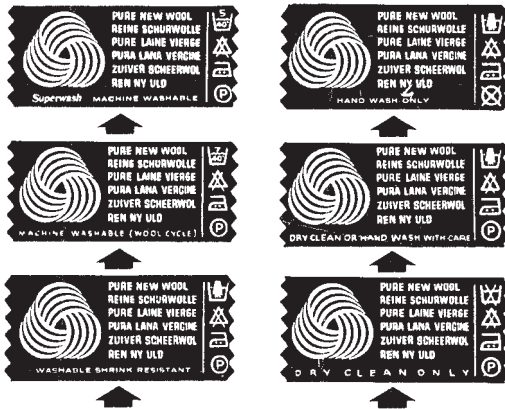
Fig.: The relationship between the care symbols and the additional information supplied beneath the woolmark for pure virgin wool (reading from lower right to upper left, the quality increases up to nonfelting wool in washing).
