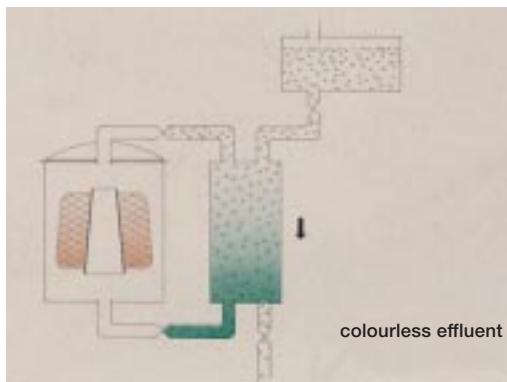
Fig. 3: Phase 1: regeneration (source: Jasper).
