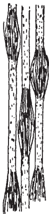
Fig. 1: Model showing a fibre which has been swollen in water (according to Hermanns).
