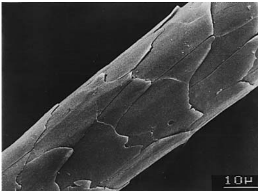
Fig.: SEM image of a mohair fibre under strong magnification.
