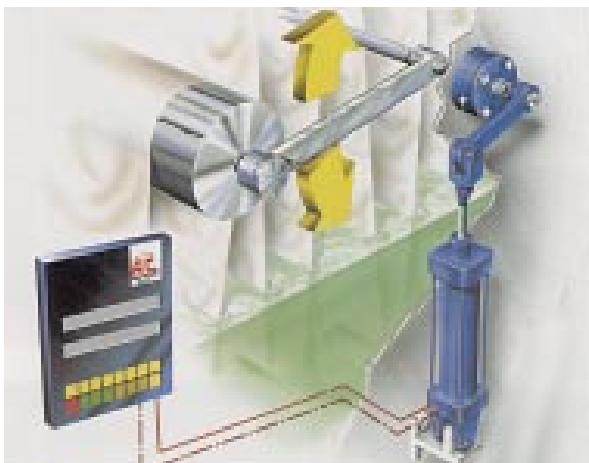
Fig. 8: Control of compensating roller setting.
