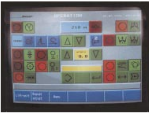
Fig.: Monitor screen display with direct touch basic control panels (masks) on a Buser rotary screen printing machine.
