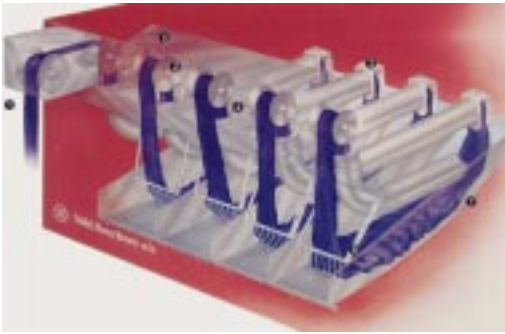
Fig. 5: Henriksen drier for tubular knitgoods. 1 = fabric feed; 2 = reel; 3 = drying tube outlet; 4 = jet; 5 = jet compartment; 6 = fabric basket; 7 = fabric chamber with Teflon coating.
