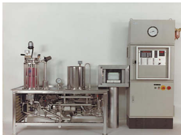
Fig. 4: Laboratory dyeing machine for 3 packages in a dyeing column (Jasper).
