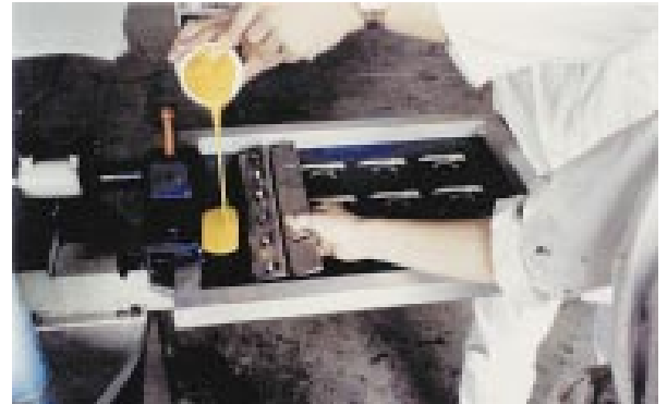
Fig. 1: Printing of flock paper with dye paste based on a special printing recipe (Tubi trans. CHT).
