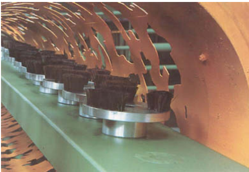
Fig. 1: Circular brushes (not set) inside a circular screen for the pattern brushing of pile fabrics (Comet).
