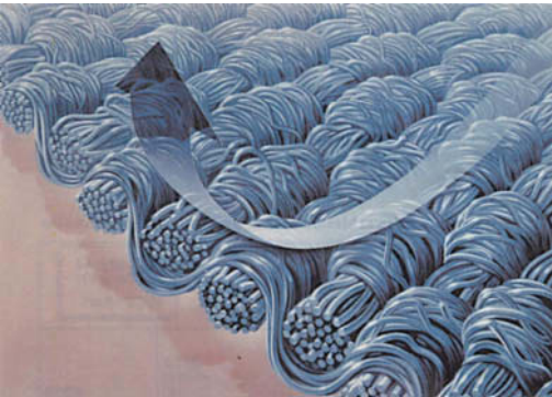
Fig. 6: The large number of densely-layered microfilaments keep the wind away; cooling is thus avoided (source: Hoechst).
