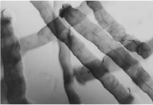
Fig. 12: Cibacron Marine C-G (Ciba Geigy) after 15 min. The fibres are entirely swollen but no dissolving has taken place.
