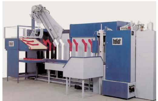
Fig. 1: Heliot machine for the continuous setting of hosiery.
