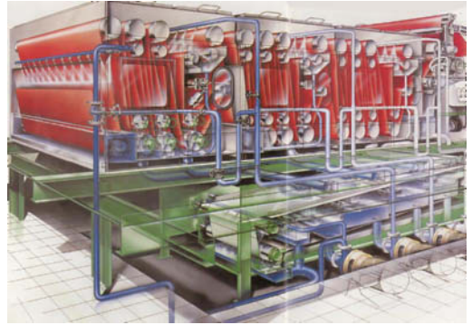
Fig. 4: Econ-Text open-width washing machine (Babcock).
