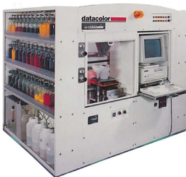
Fig. 1: Dispenser (by datacolor) for dispensing standard solutions in the laboratory.
