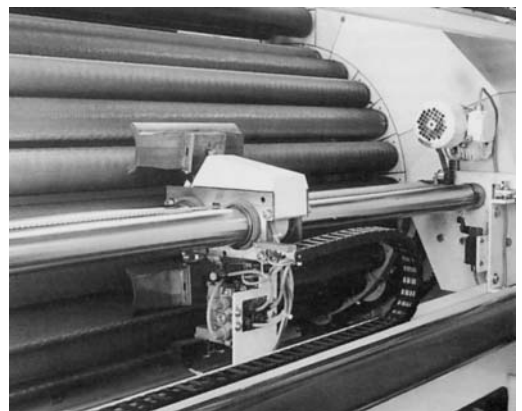
Fig. 16: An automatic raising element sharpening device from the Sucker-Müller company.
