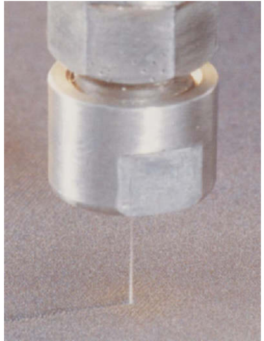
Fig. 1: Typical water jet cutter nozzle.
