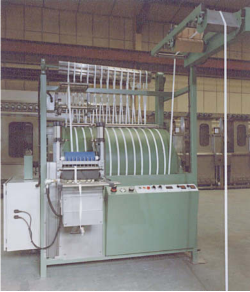
Fig.: Webtex narrow fabric finishing plant (left: entry; right: exit).
