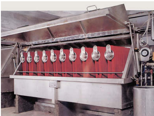
Fig. 1: Fong's rope dyeing machine.
