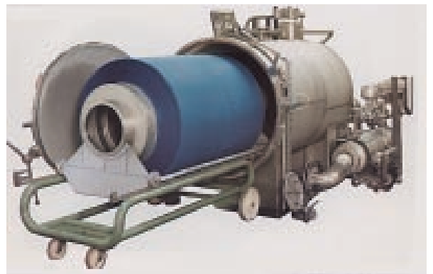
Fig. 1: Running out the dyed fabric beam on a beam dyeing machine (Durand).
