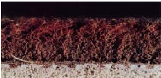
Fig. 7: Carpet without finish, subjected to wear (Reich).
