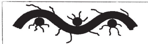
c) linty fibrils after primary fibrillation
