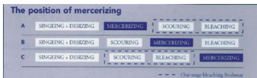
Fig.: Mercerizing position in cotton pretreatment.
