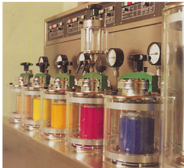
Fig. 2: Ahiba Turbocolor with transparent walled dye containers.
