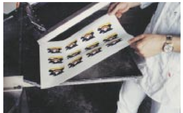
Fig. 2: Completed print in three colours on the flocked ground (Tubi trans. CHT).
