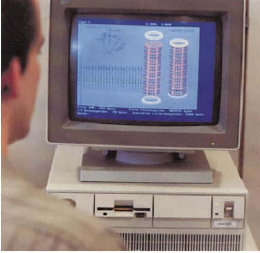
Fig. 2: The design and material-compatible conversion of technical textile requirements in a plastics injection moulding tool is effected by the tube manufacturer, also with the aid of specially designed electronic data processing systems.
