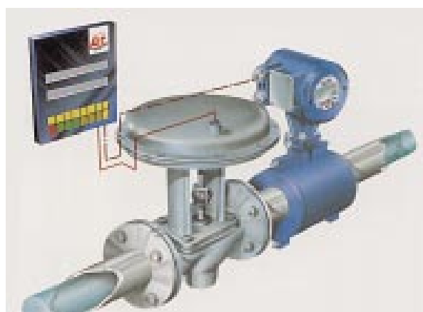
Fig. 4: Control of addition of water with a flow meter.
