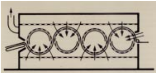
Fig. 10: Through-flow drier based on the sieve-drum principle (Fleissner).
