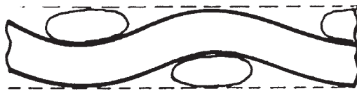
Fig. 1: Fabric porosity: the fabric is a porous plate, while the threads are solid.
