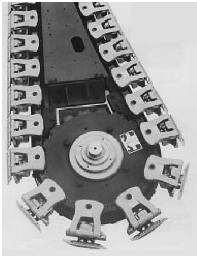
Fig. 3: Horizontal chain return (Babcock).
