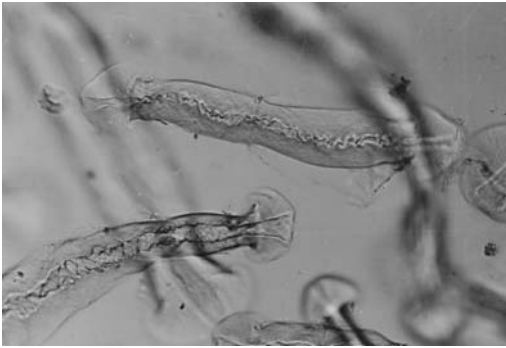
Fig. 11: Solubility in cuprammonium as endless swelling. Blank dyed sample after 10 s: the dissolving process here is also connected to a swelling process, as shown in the photograph.
