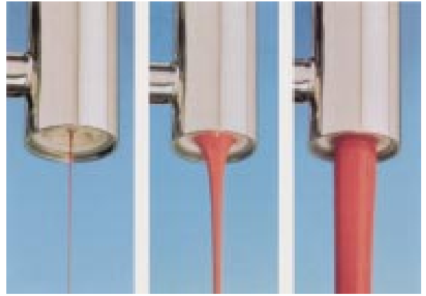
Fig. 1: Flow characteristics of print pastes demonstrated on an ACS datacolor metering valve.
