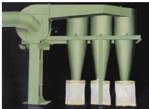
Fig. 1: Cyclone unit (LTG).
