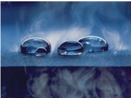
Fig.: Water droplets being repelled on a water repellent fabric (by Sulzer Rütli).
