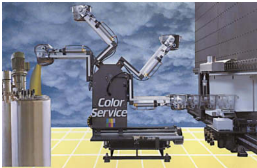
Fig. 2: Robot for transferring weighed dye powder container from scales to dissolving container.
