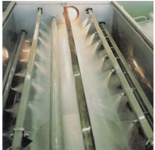
Fig. 3: A suction drum wash compartment with a spraying system (Babcock) covering the full width of the goods.
