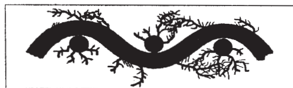
d) fabric after cellulase treatment
