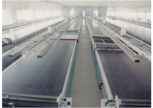
Fig. 2: Table printing room with electrically heated tables and typical repeat edges (by Sigma).
