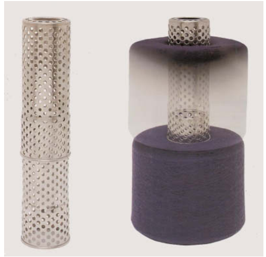
Fig. 1: Perforated steel dyeing cores for the dyeing of cross-wound yarn packages (Fong's).
