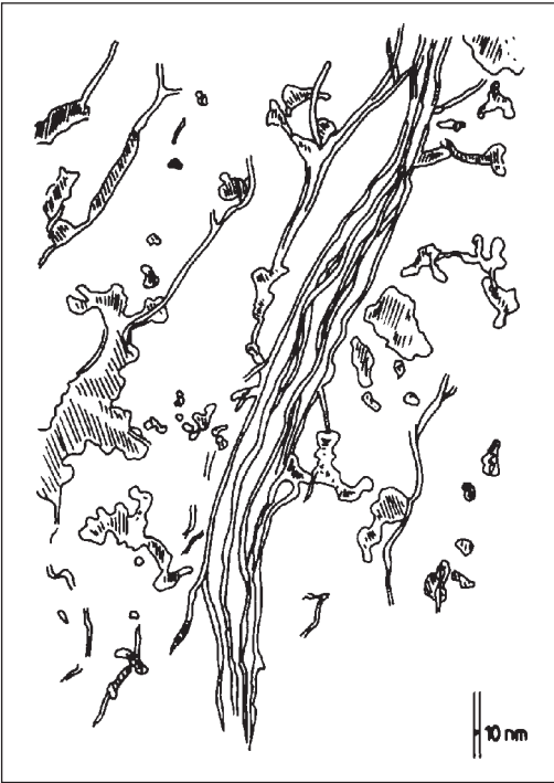
Fig. 18: Diagram, drawn from electron microphotographs, of reconstructed microfibrils from low-sulphur wool proteins in thiol form (Thomas, Conrads and Phan 1985).
