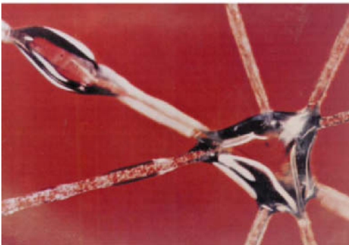
Fig. 3: Differences in binder cover depending on application: Bonding points from dipping (top) and foam application (bottom) (Bayer).
