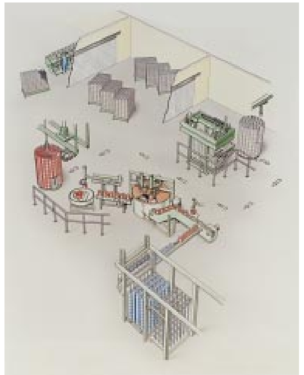
Fig. 12: The Jasper automatic system for preparation of bobbins in a yarn dyehouse.
