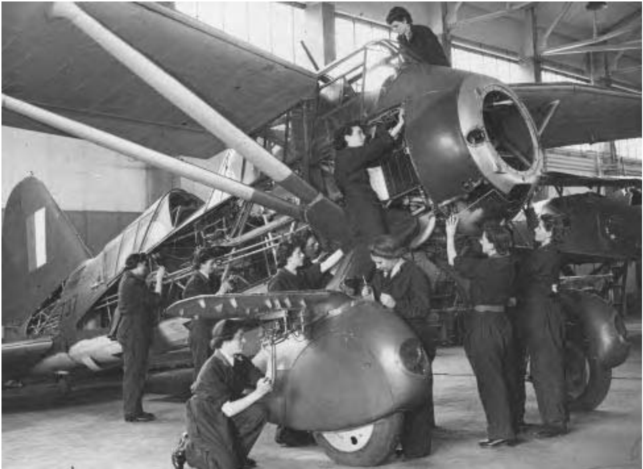
WAAF personnel work on the advanced rigging maintenance of a Lysander aircraft. (Hulton Archive)
