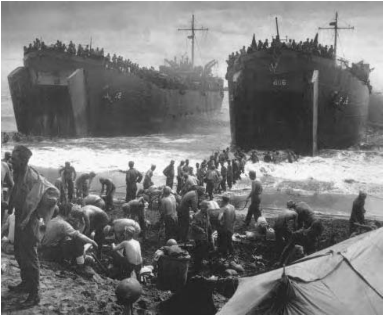
Two Coast Guard-manned LSTs open their bows in the surf that washes on Leyte Island beach, as soldiers strip down and build sandbag piers out to their ramps to speed up unloading operations. 1944. (National Archives)
