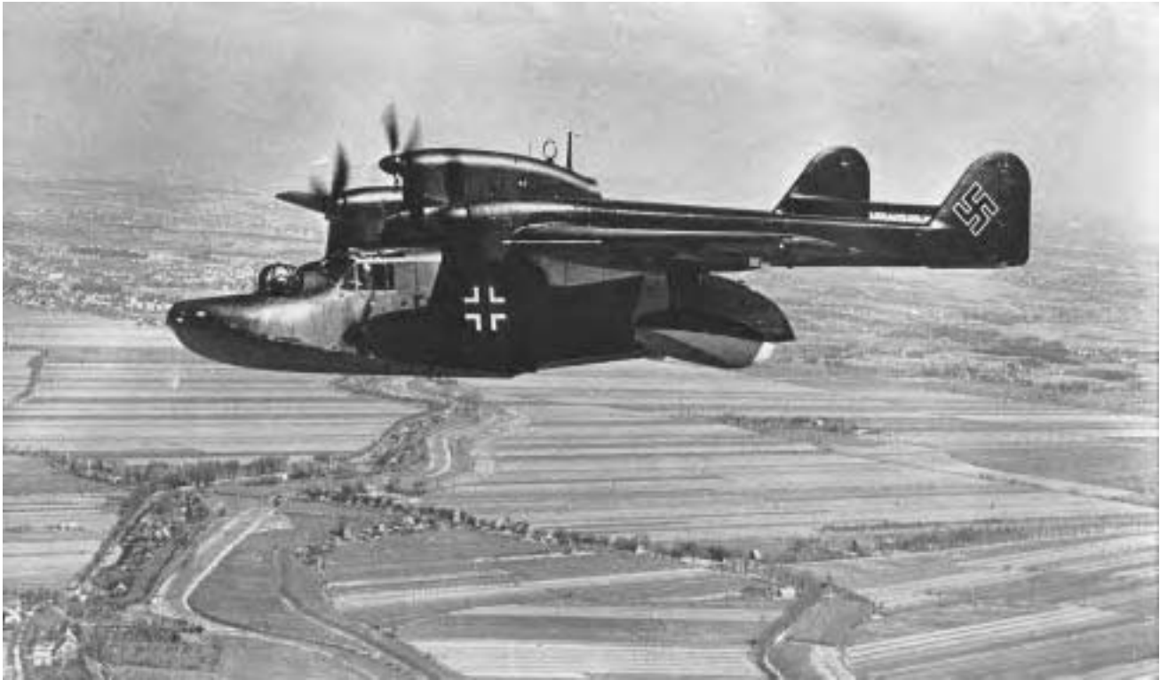
A German Blohm und Voss Bv.138B reconnaissance bomber seaplane. (Museum of Flight/Corbis)
