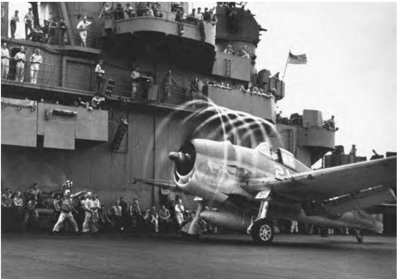
The motion of its props causes an “aura” to form around this U.S. Navy Grumman F6F Hellcat on the carrier Yorktown. Rapid change of pressure and drop in temperature create condensation. Rotating with the blades, the halo moves aft, giving depth and perspective. November 1943. (National Archives)
