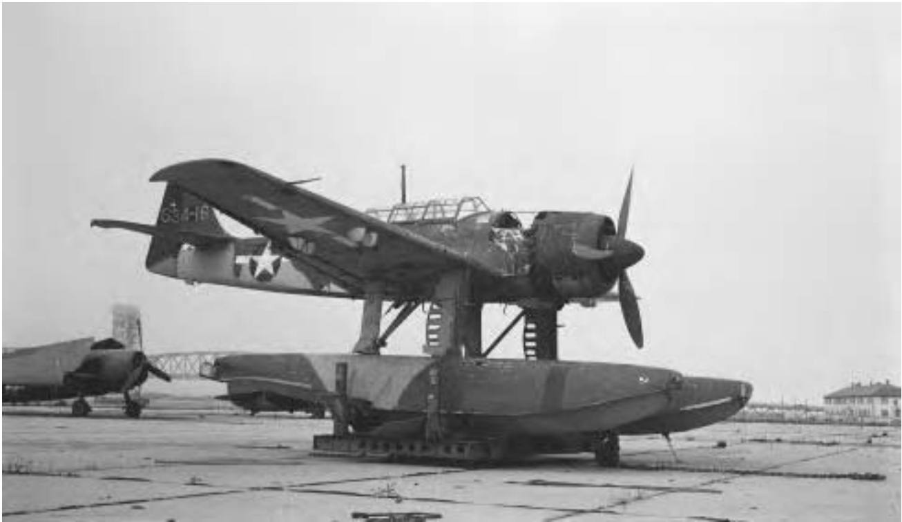
A Japanese Aichi Eiga Zuiun naval reconnaissance and dive bomber with the Allied code name “Paul.” The U.S. Navy insignia was placed on the aircraft after its capture. (Museum of Flight/Corbis)
