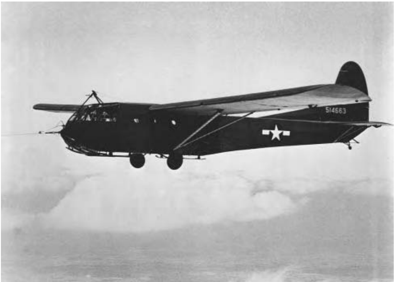
A U.S. Waco CG-4A glider with a Griswold Corey nose skid, under tow. (Corbis)
