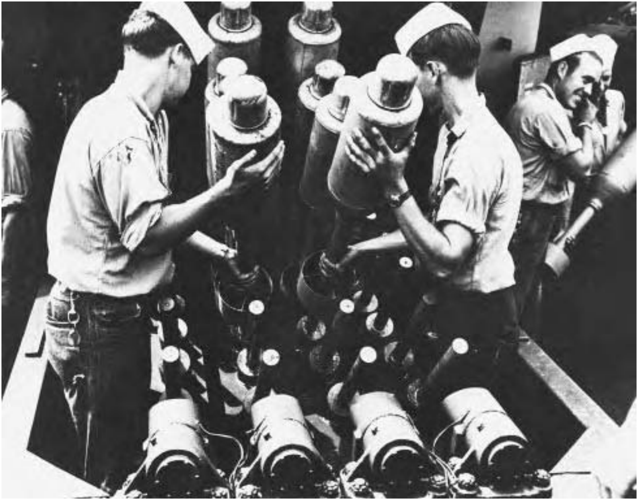
U.S. Navy sailors load hedgehog bomb projectors used in antisubmarine warfare. (Corbis)
