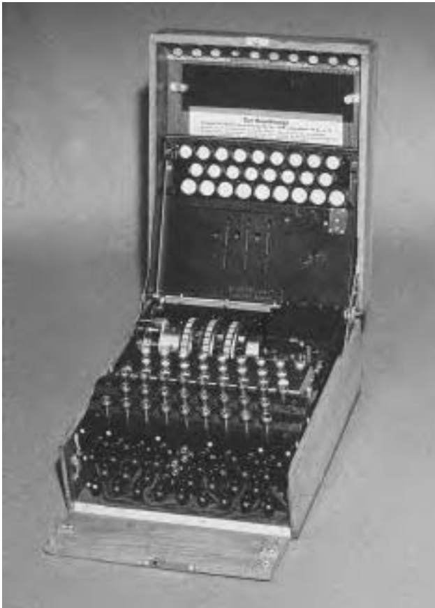
An Enigma cipher machine, used by the German military in World War II. (Hulton Archive)
