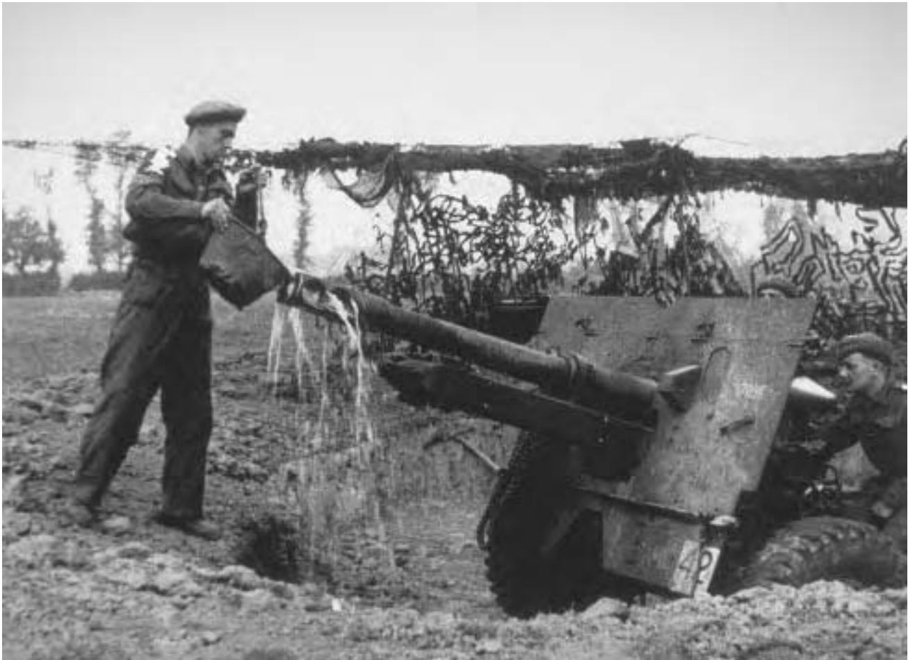
This British Army 25 pounder was part of an eight gun battery which fired 4000 rounds in just over 15 hours. Firing was continuous and water was used to keep the guns cool. (Photo by Keystone/Getty Images)
