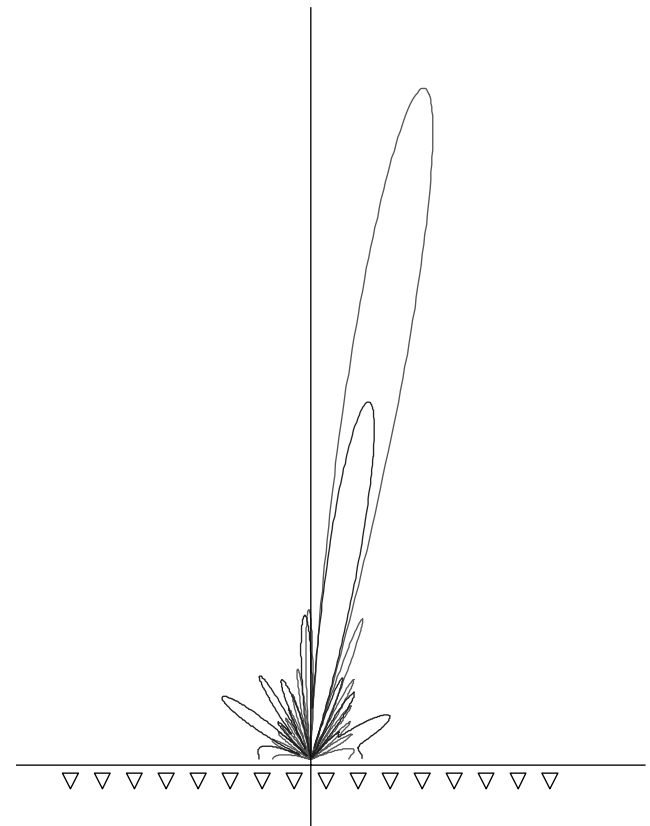
Figure 9. One statistical representation of single beam adaptive beamforming of a 16-element linear array with 0 dB SNR per element. Adaptively formed beam — blue; ideal beam — red.
