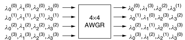
Figure 14. Input port and wavelength redistribution for a 4 \times 4 AWGR.
