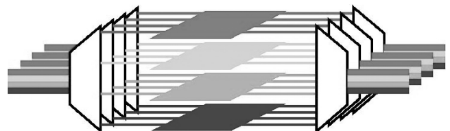
Figure 8. Wavelength-Selective Crossconnects uses small N \times N switches as building block. The small switch port count ( N ) is equal to the input fiber number. The total package number ( M ) is increased when new wavelengths are turned on. The total bandwidth capacity of a WSXC is N times M , which can be extremely large with scalability and low first-install cost.
