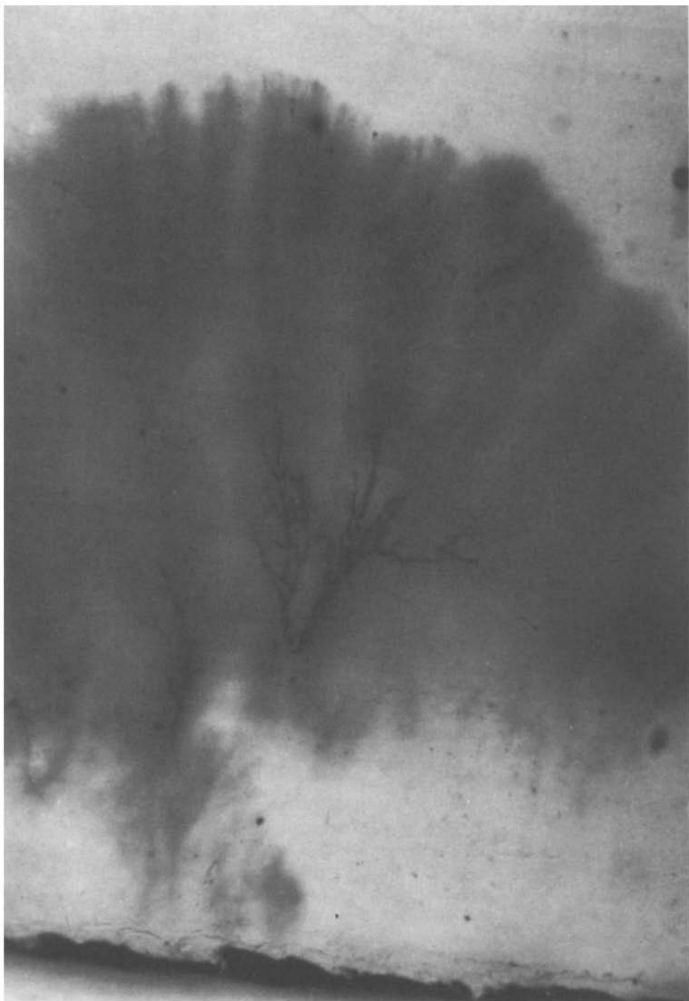
Fig. 24.4 Electrical tree forming within a water tree
