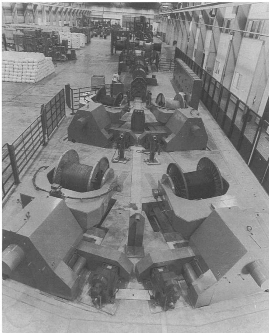
Fig. 25.7 Drum-twister laying-up machine
