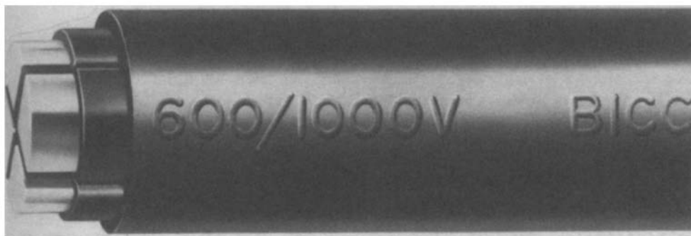
Fig. 21.2 600/1000 V, 4-core unarmoured cable with solid aluminium conductors
