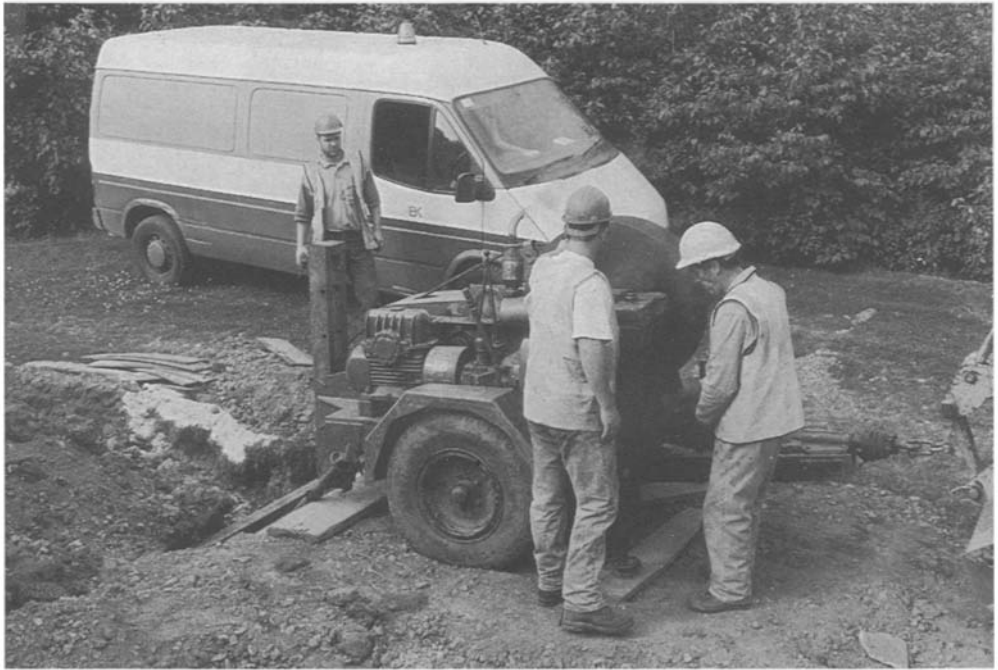
Fig. 26.5 Diesel driven winch for safe working load of 4 tonnes. Transmission is through a gear box coupled to a pair of 'bull wheels'
