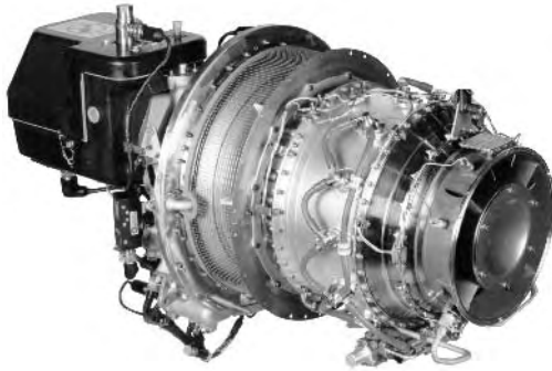
Figure 11-2. Courtesy of United Technologies Corporation, Pratt & Whitney Aircraft. The PW206 turboprop engine is a 700 shaft horsepower engine used primarily in helicopter applications. Current applications include the Agusta A109E Power , Bell M427, Eurocopter EC135P1/P2, and the MDHI MD900/902.
