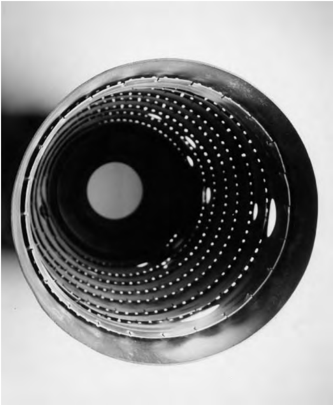
Figure 3-12. Courtesy of United Technologies Corporation, Pratt & Whitney Aircraft. A combustor outlet view of one of the nine combustors in the, 25.5 megawatt, FT8 aero-derivative gas turbine. Flame temperature at the center of the combustor approaches 3,000°F. The small cooling holes enable a flow of compressor air to continuously cool the combustor liner walls.
