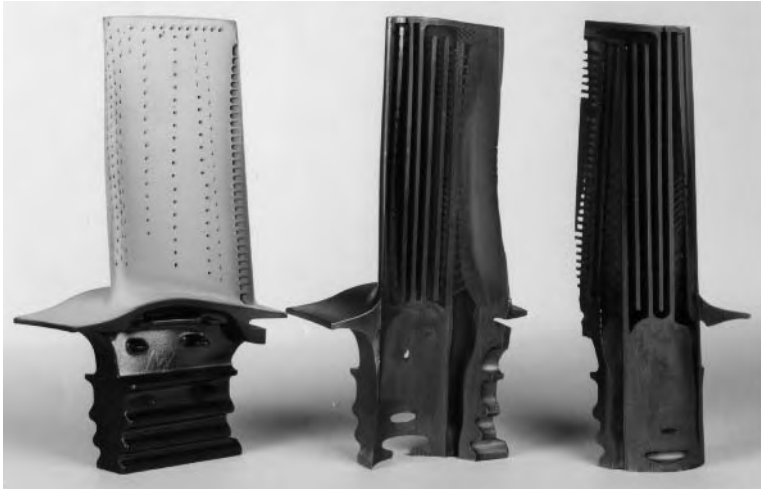
Figure 3-10. Courtesy of United Technologies Corporation, Pratt & Whitney Aircraft. Internal structure of high pressure turbine blade showing the cooling distribution throughout the core of the blade airfoil and root.
