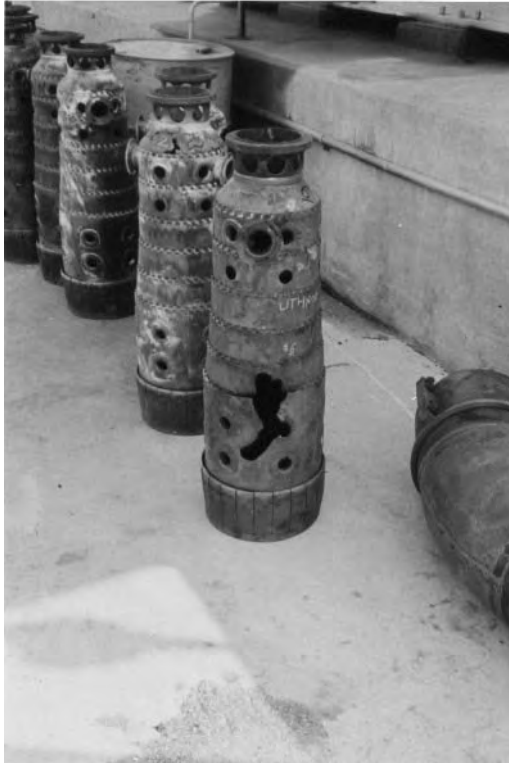
Figure 13-10. Can-annular combustor failure (burning and cracking) due to liquid mist in the fuel gas. 55,000 horsepower gas turbine-generator unit with less than 10,000 operating hours.
