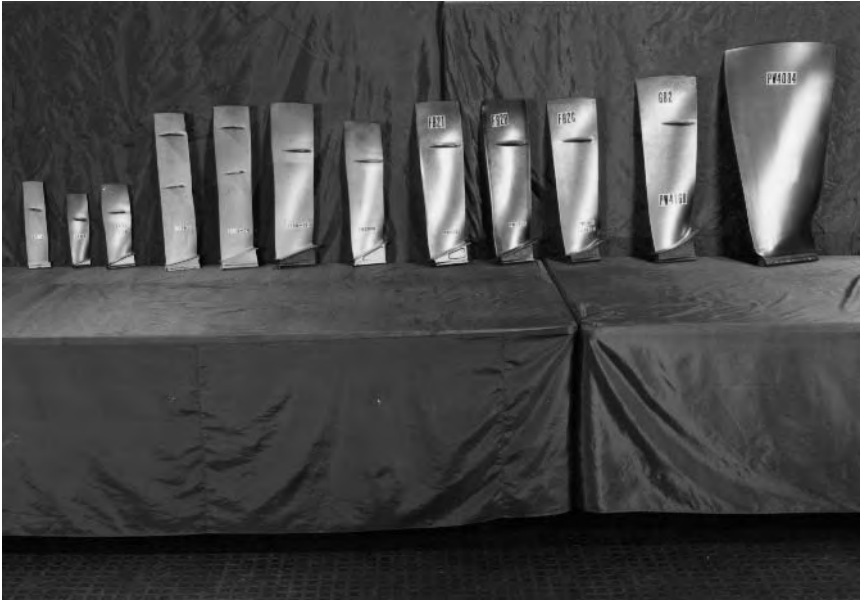
Figure 3-5. Courtesy of United Technologies Corporation, Pratt & Whitney Aircraft. A pictorial summary portraying the history of compressor blades from the early JT3 turbojet compressor blade on the left through to the most recent PW4084 blade on the right. This photograph represents a three-fold increase in compressor pressure ratios.
