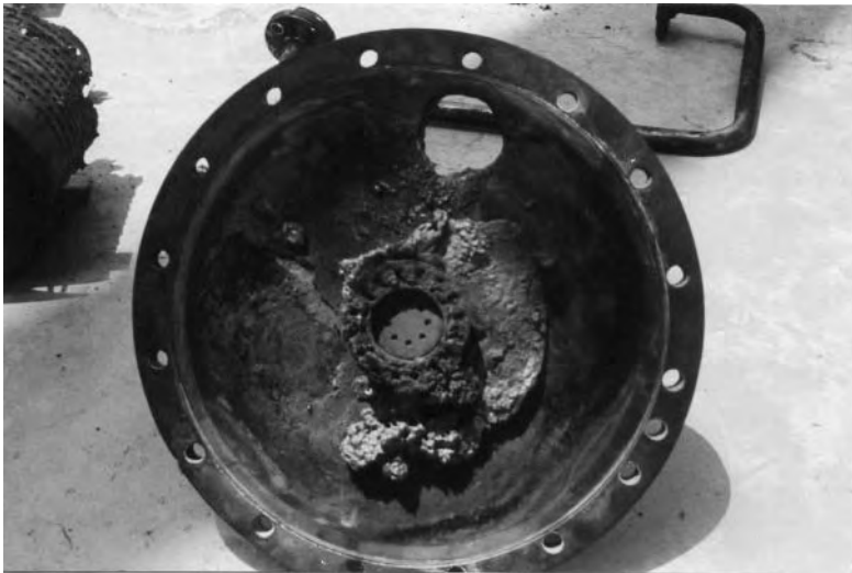
Figure 13-12. Can-annular combustor fuel nozzle coking. 30,000 horsepower gas turbine-pump drive unit. Operating hours unknown.
