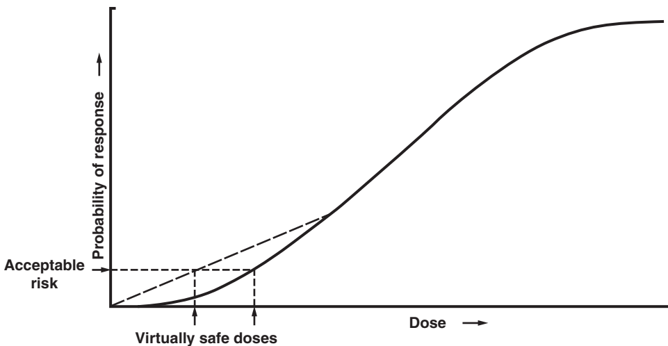
FIGURE 24.25 The effect of linear extrapolation of a sublinear dose-response curve on the determination of a virtually safe dose (VSD). (Reprinted from Munro, I.C. and Krewski, D.R., FD. Chem. Toxicol. , 19, 549, 1981, 20 with kind permission from Elsevier Science, The Boulevard, Langford Lane, Kidlington OX5168B UK.)
